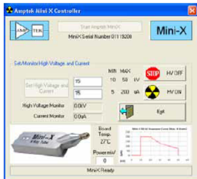
USB Software Interface. Allows the user to set the voltage and current as well as monitor both parameters.
