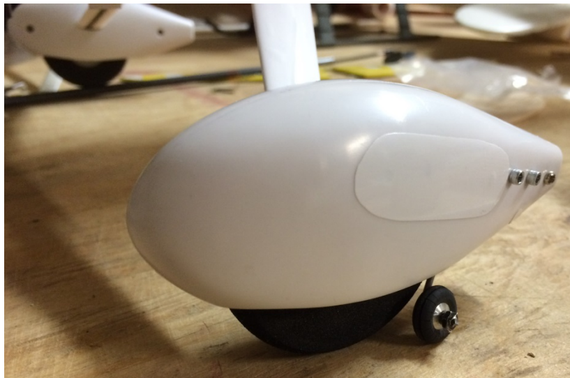
Figure 14. Weight on Wheels Switch Nestled Inside the Left Main Landing Gear Fairing.
