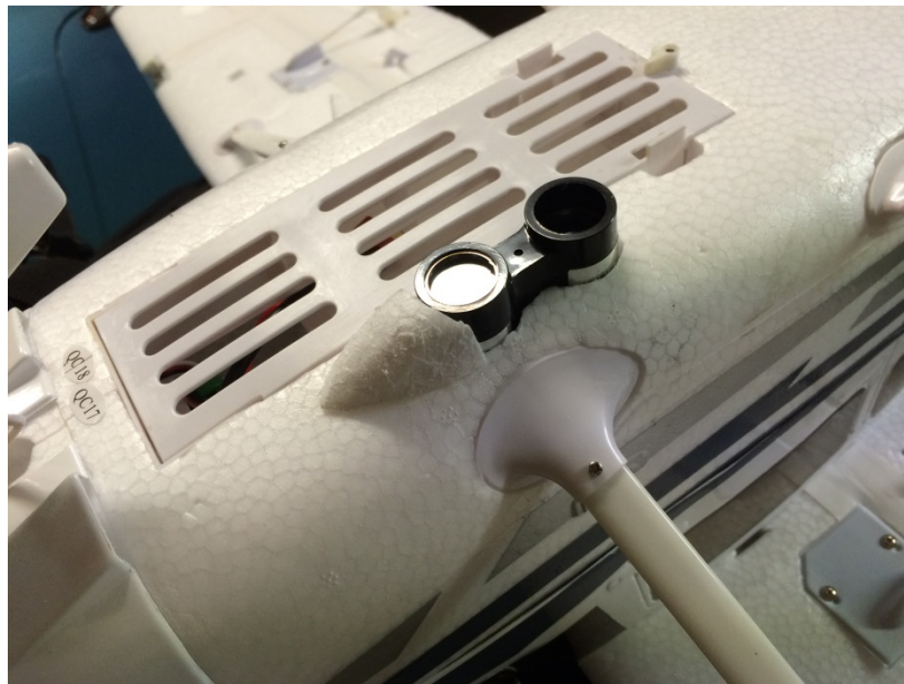
Figure 3. Detail of the LIDAR-Lite Installation.
