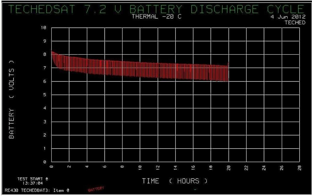
Figure XX-Test Battery Discharge at -20C
