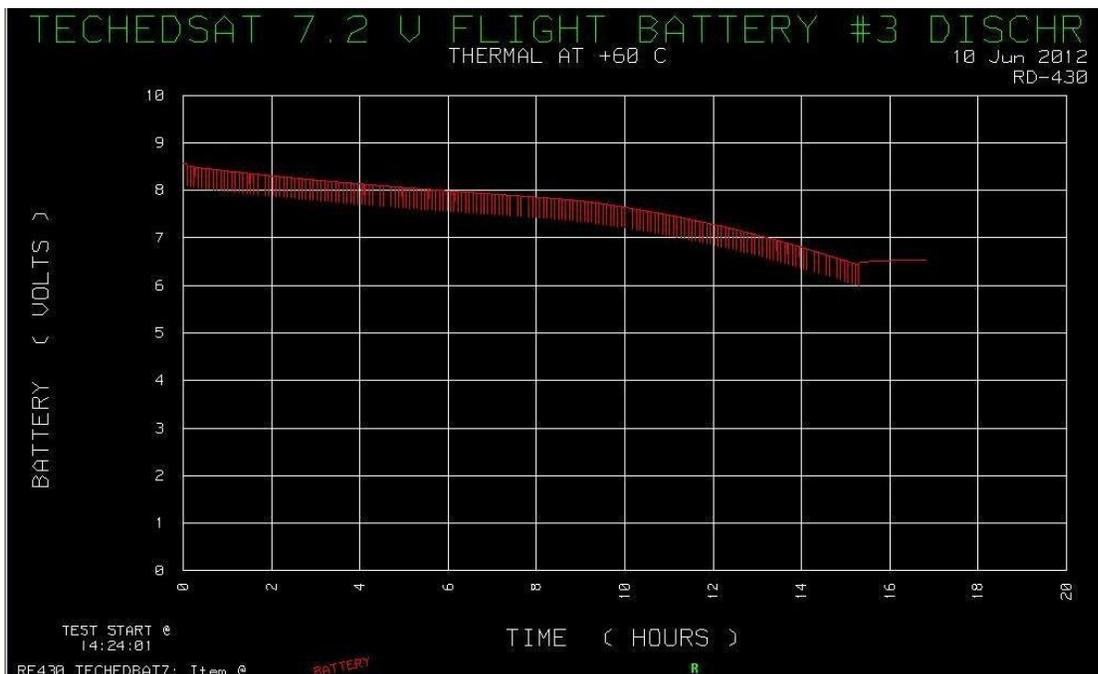
Figure XX=Spare Flight Battery Discharge Cycle at 60°C
