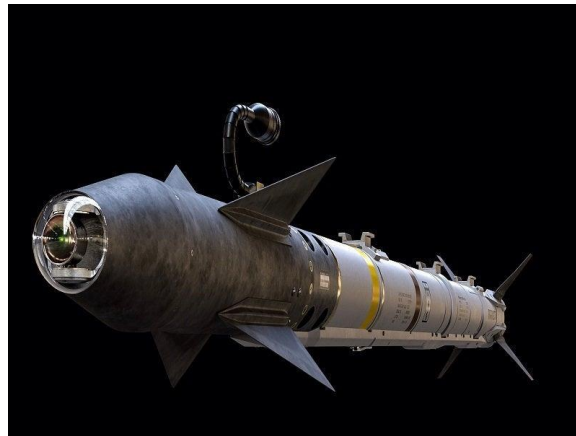
Figure 1-3 – U.S. Air Force and U.S. Navy AIM-9X Sidewinder missiles use vector-controlled fins [3].
