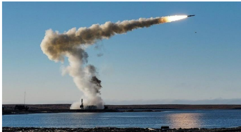
Figure 1-6 – The Russian K-300P Bastion P missile is launched vertically, and an attitude control system is used to adjust the heading angle [23].
