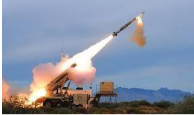
Figure 1-7 – The American Lockheed Martin Patriot PAC-3 missile engages an attitude control system to adjust the heading angle after launch [24].
