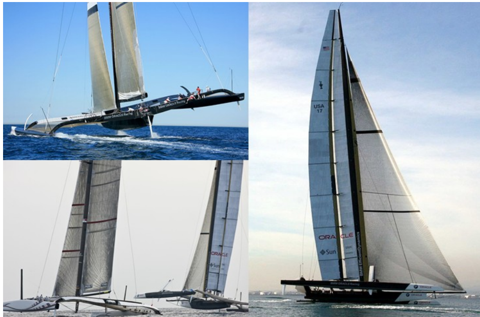
Figure 2: (Clockwise from top left): USA 17 with its traditional soft sail B , USA 17 with the wing mast and sail C , USA 17 and Alinghi 5 racing in the 2010 America's Cup D
