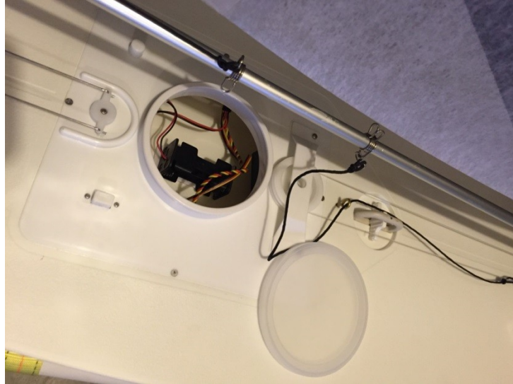
Figure 12: Servos and battery pack for the RC Laser
