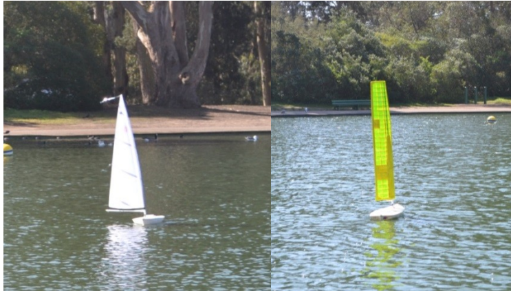
Figure 14: Testing on Spreckles Lake, traditional sail (left) and wing sail (right)
