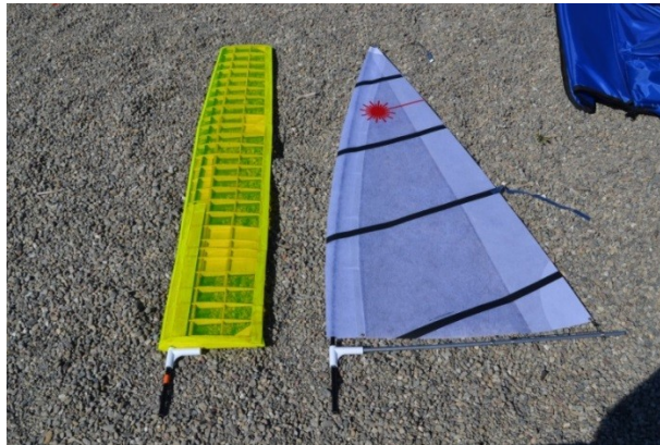
Figure 13: Wing sail (left) and traditional sail (right) used for the testing
