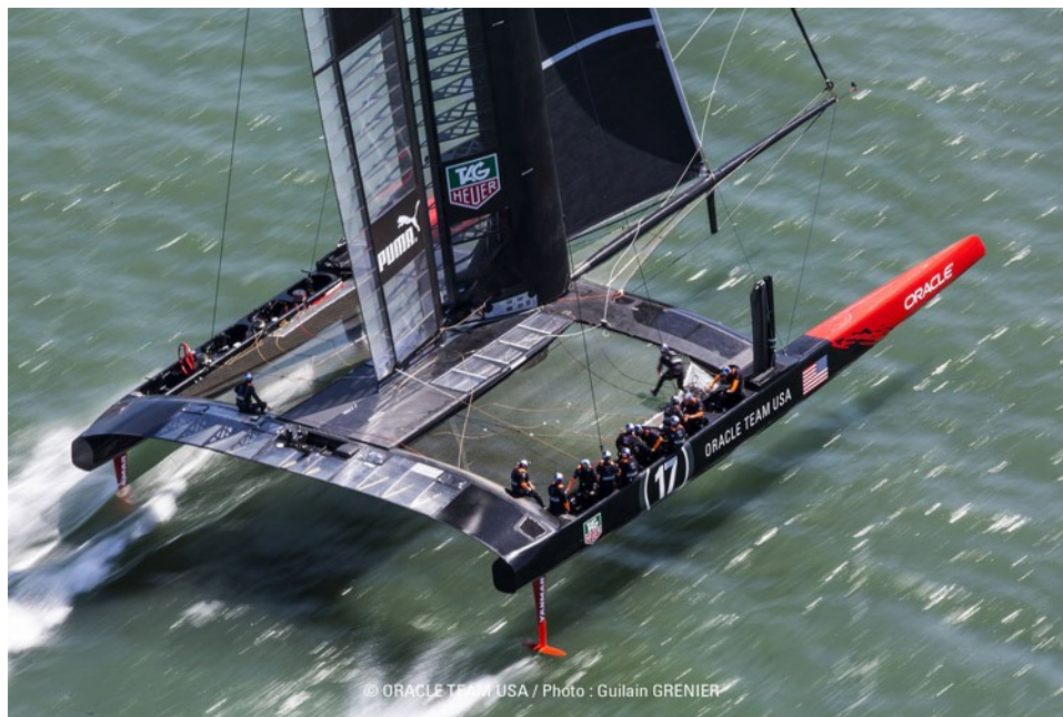
Figure 19: Oracle Team USA, winner of the 34th America's Cup with their cambered wing main sail 4
