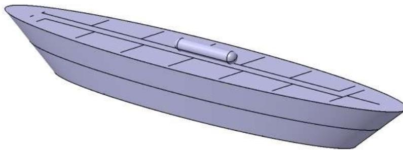
**Figure 19 Preliminary hull design, indicating fuel tank position and relative size.**
