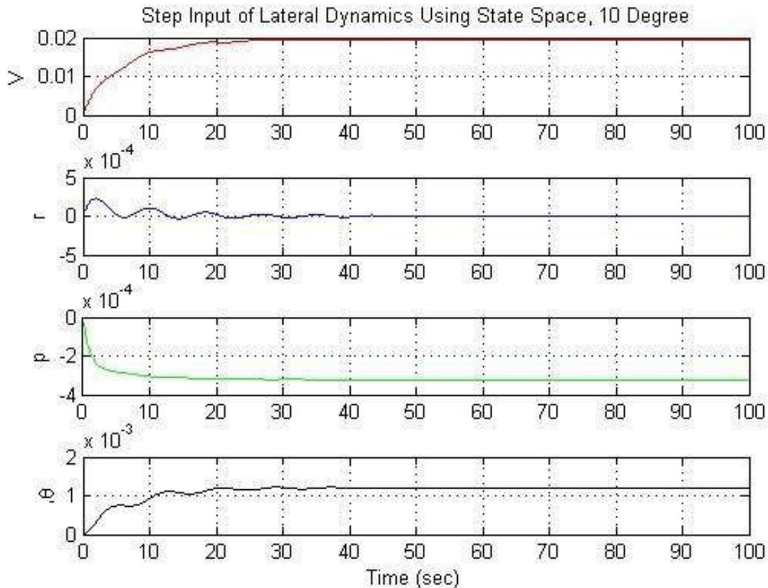
**Figure 40 Step input of Lateral Dynamics using state space for 10-degree input**
