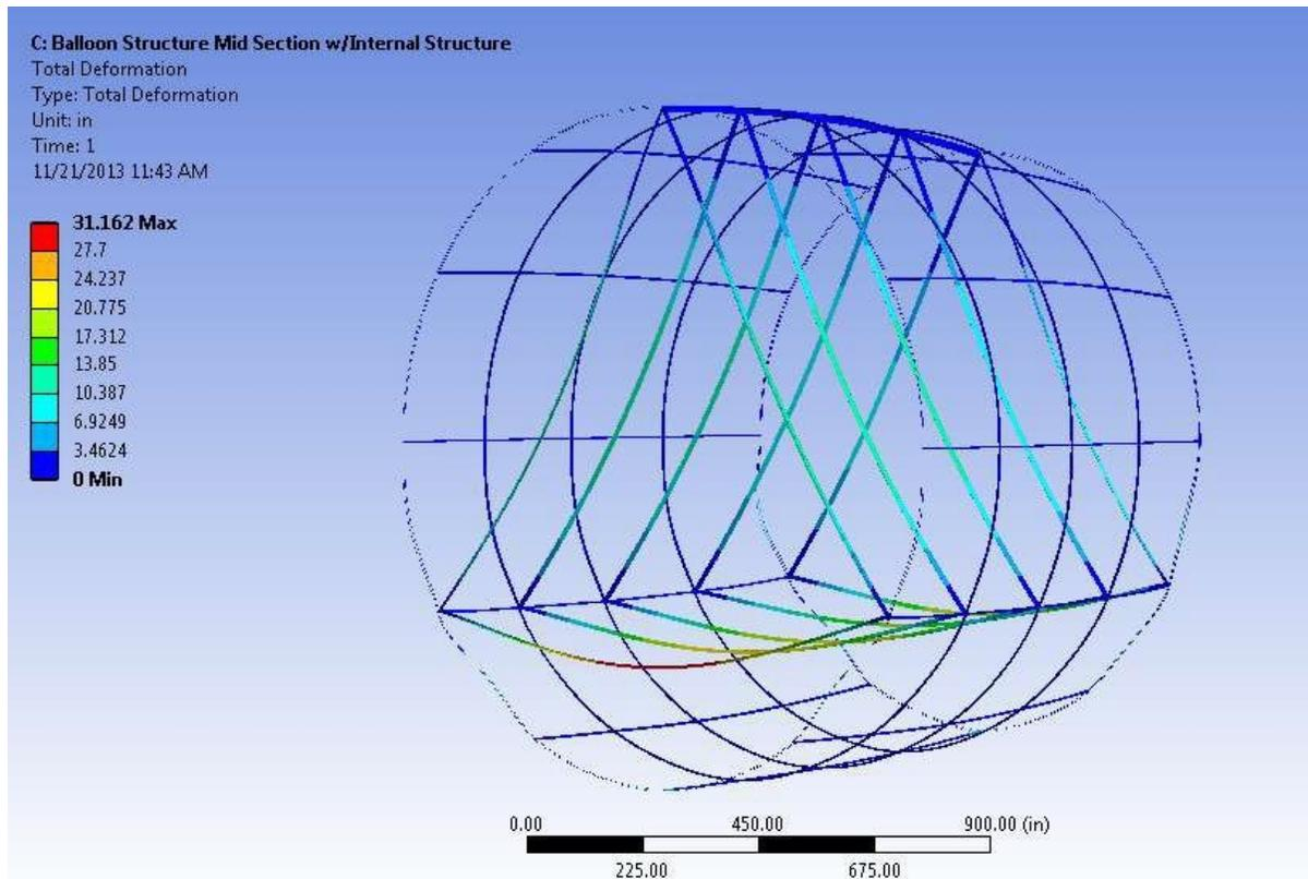
**Figure 23 Structural Deformation analysis with cabin mass**
