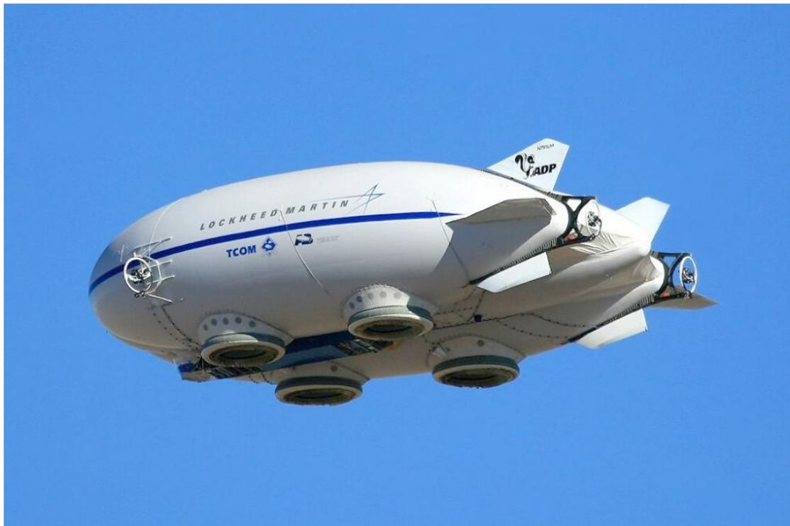
Figure 51 Lockheed Martin's P-791 with ACLS arrangement (Dietl, 2010)
