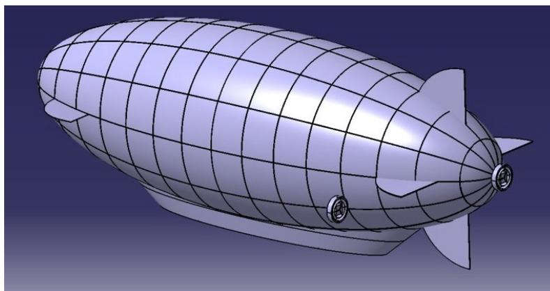
**Figure 28 Axisymmetric airship hull with four equally sized tailfins**
