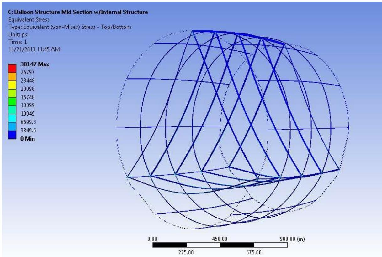
**Figure 22 Structural stress analysis with cabin mass**
