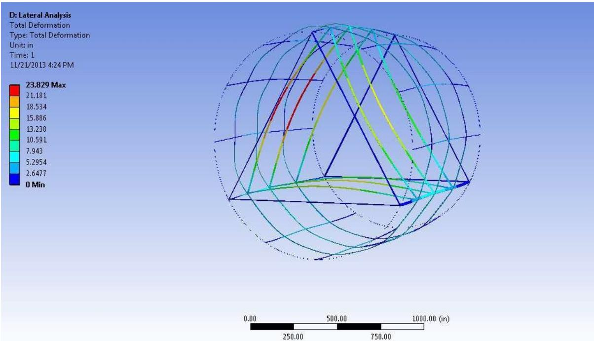
Figure 25 structural deformations due to lateral gusts
