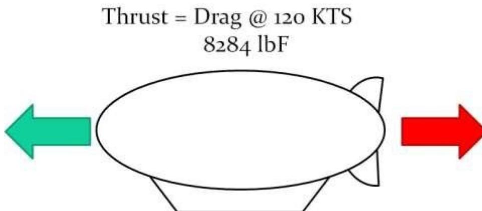
Figure 44 Thrust equals drag analysis
