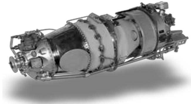
**Figure 41 Power-plant selection: PT6A-60AG**
