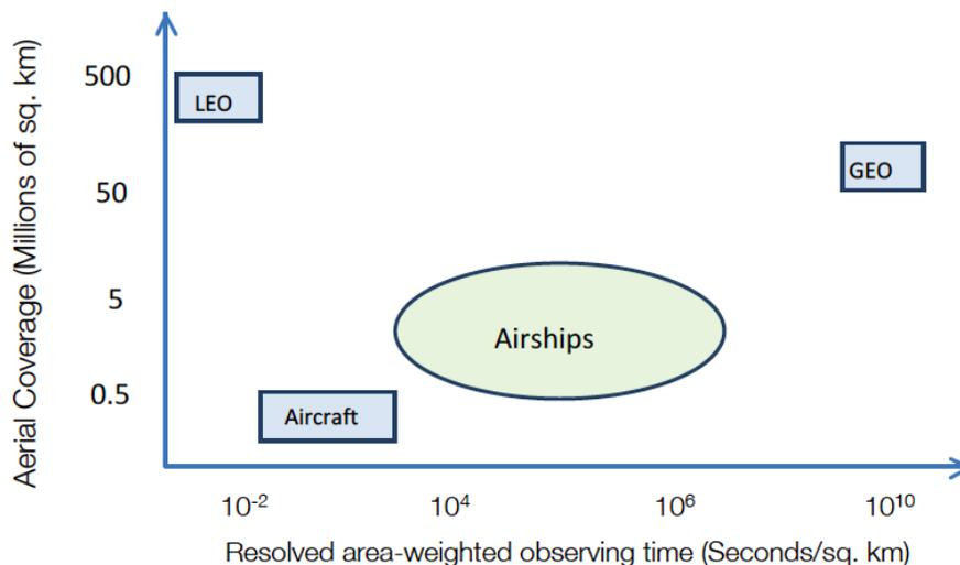
**Figure 11 Comparison of observational attributes of airships to other platforms. (Keck, 2014)**
