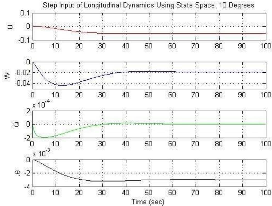
**Figure 37 Step input of longitudinal Dynamics using state space for 10-degree elevator input**
