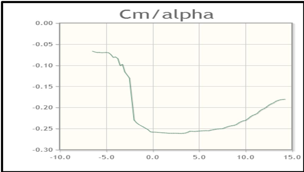
Figure 32 Moment Coefficient of the airfoil
