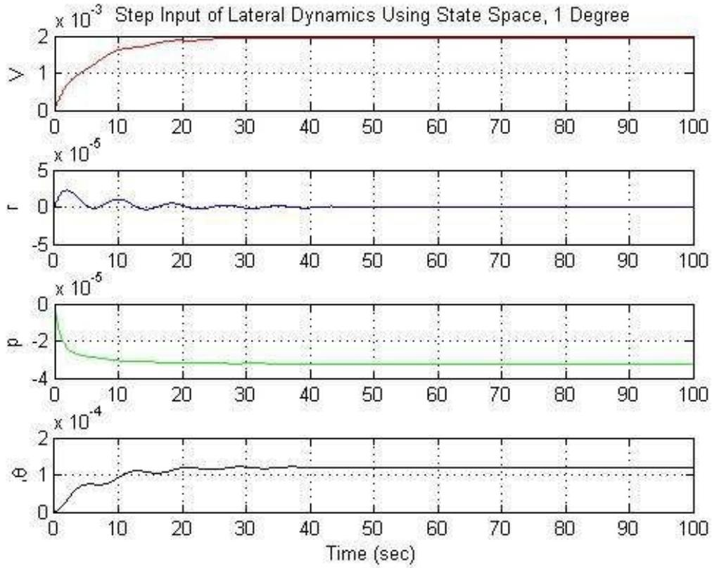
Figure 38 Step input of Lateral Dynamics using state space representation for 1-degree input
