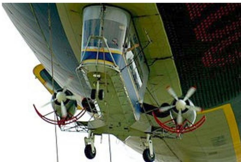
Figure 49 Classical Tri-wheel landing gear arrangement. (Dietl, 2010)
