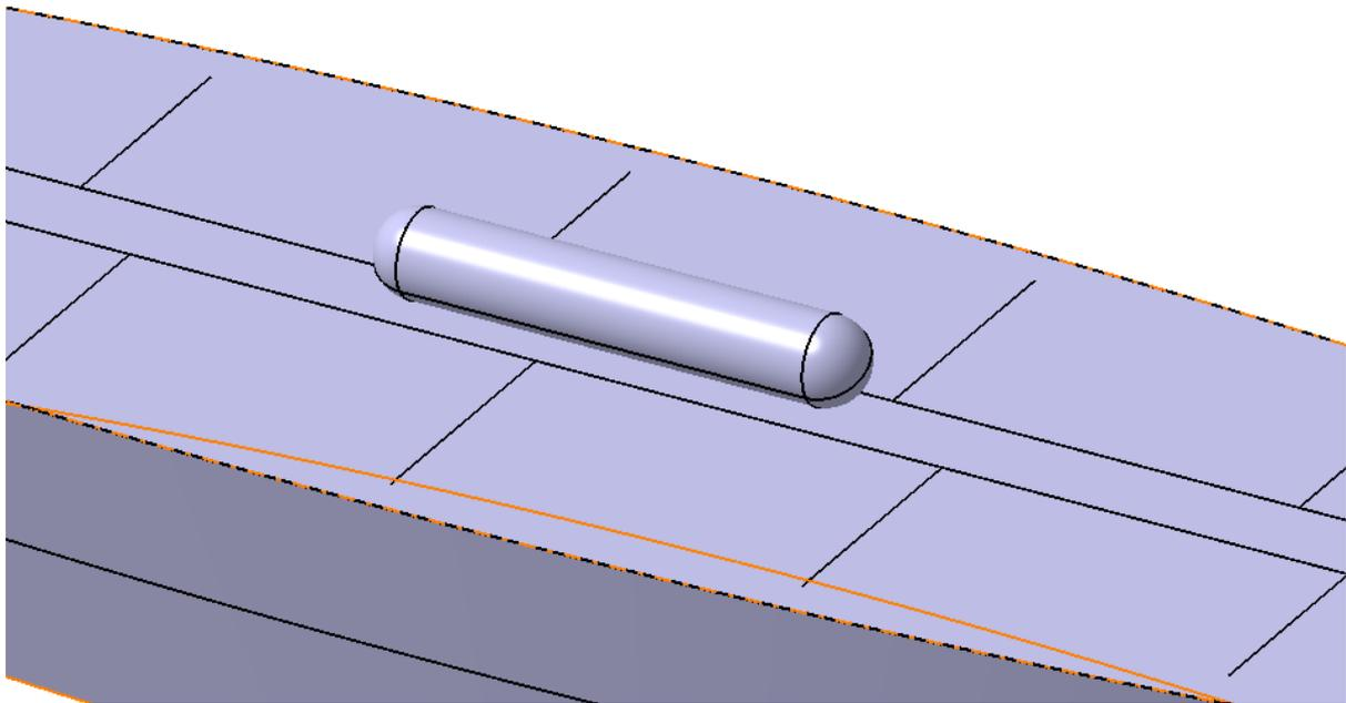
**Figure 47 Fuel-tank placement**
