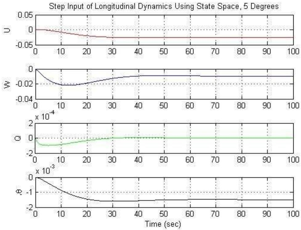
Figure 36 Step input of Longitudinal Dynamics using state space for 5-degree elevator input
