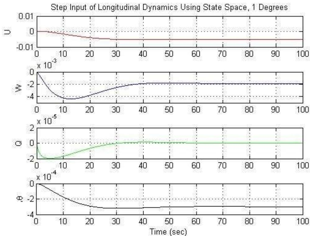
**Figure 35 Step input of Longitudinal Dynamics using state space for 1-degree elevator input**
