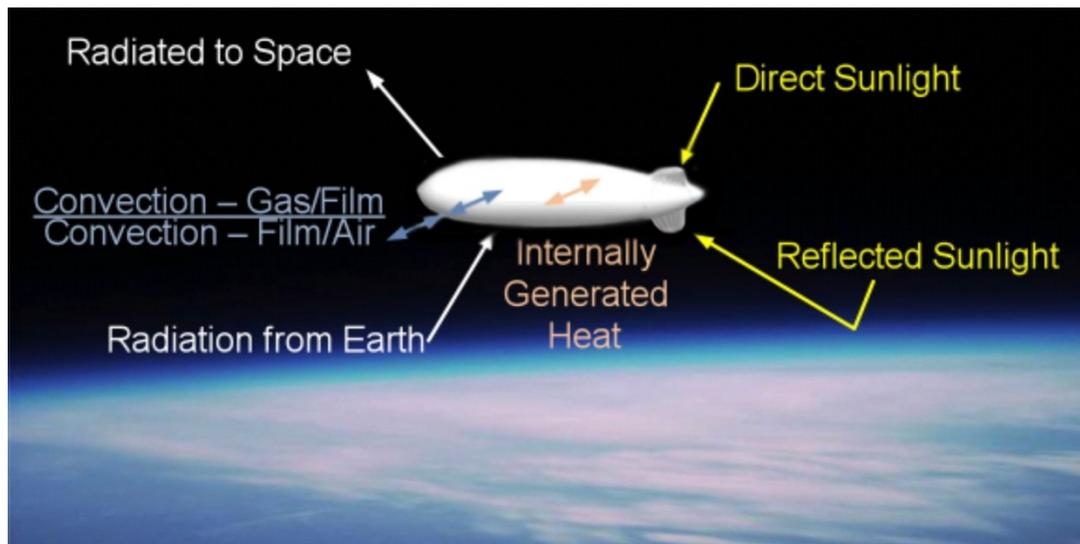
Figure 26 Heat loads on an airship. (Keck, 2014)
