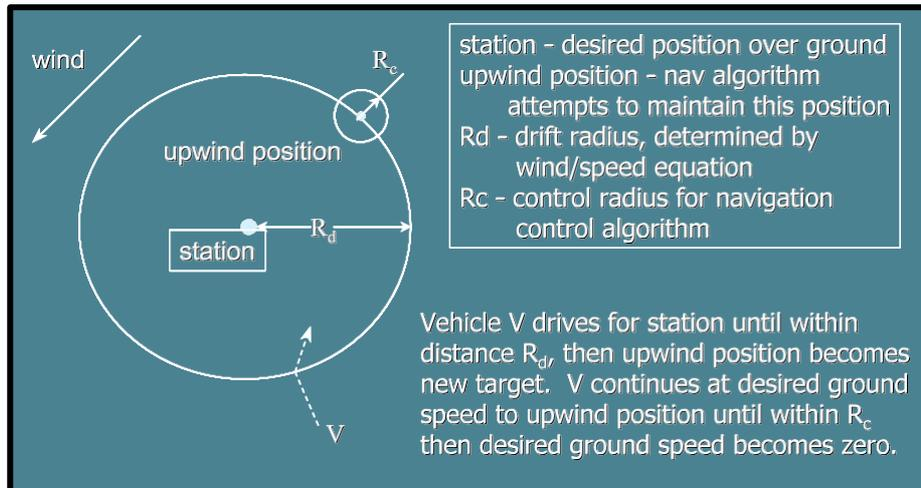
Figure 45 "Sprint and Drift" method of navigation
