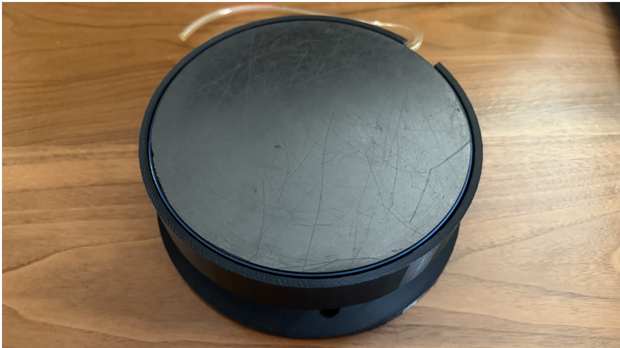
Figure 6.1: Air bearing & 3D printed shell
