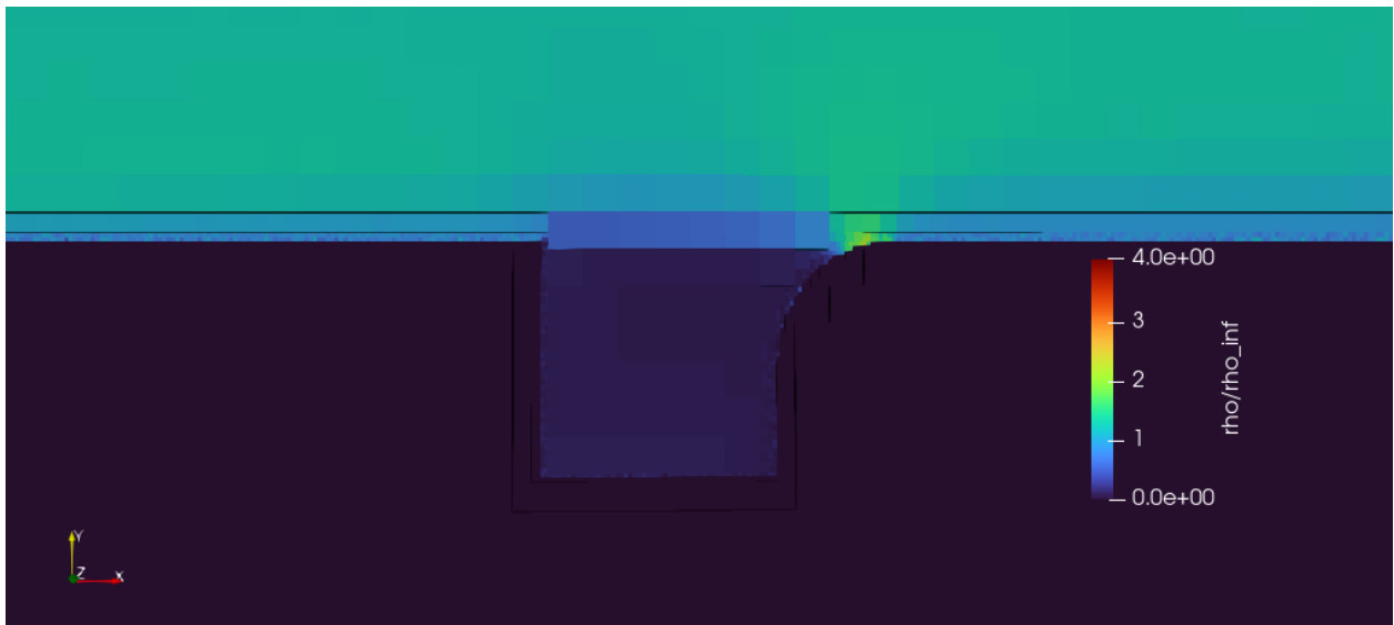
Fig. 5.9: Closeup of mass density ratio contour for case 2
