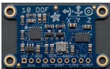
Figure 3. Adafruit 10 DOF IMU
