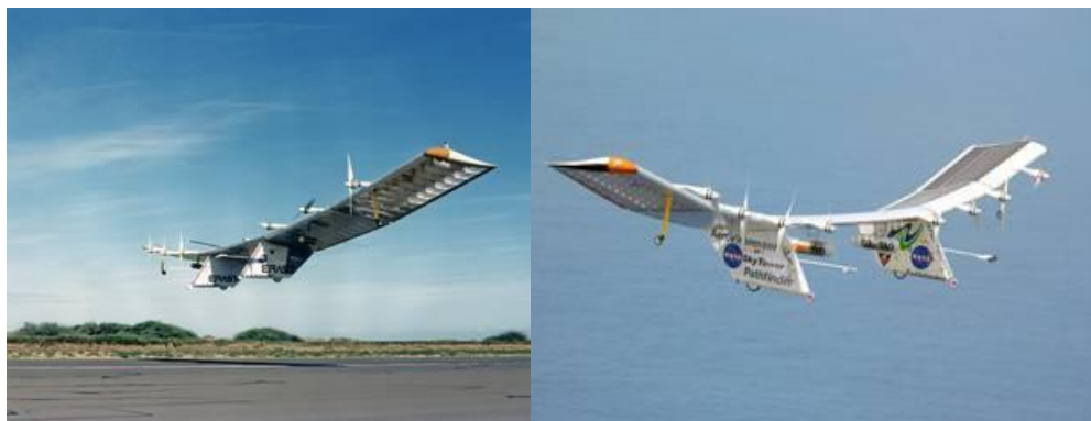
Picture 5. NASA Pathfinder (L) and NASA Pathfinder Plus (R). [6] [7]
