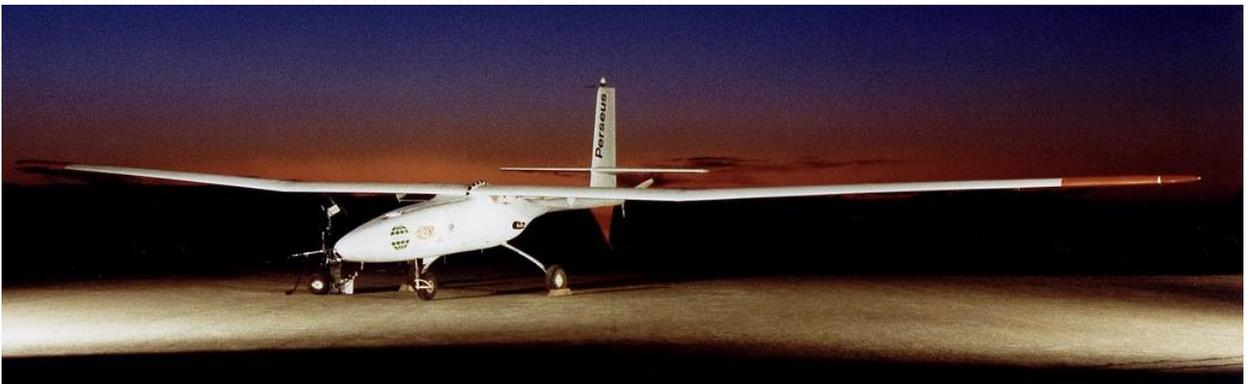
Picture 8. Perseus B Remotely Piloted Aircraft <sup>22</sup>
