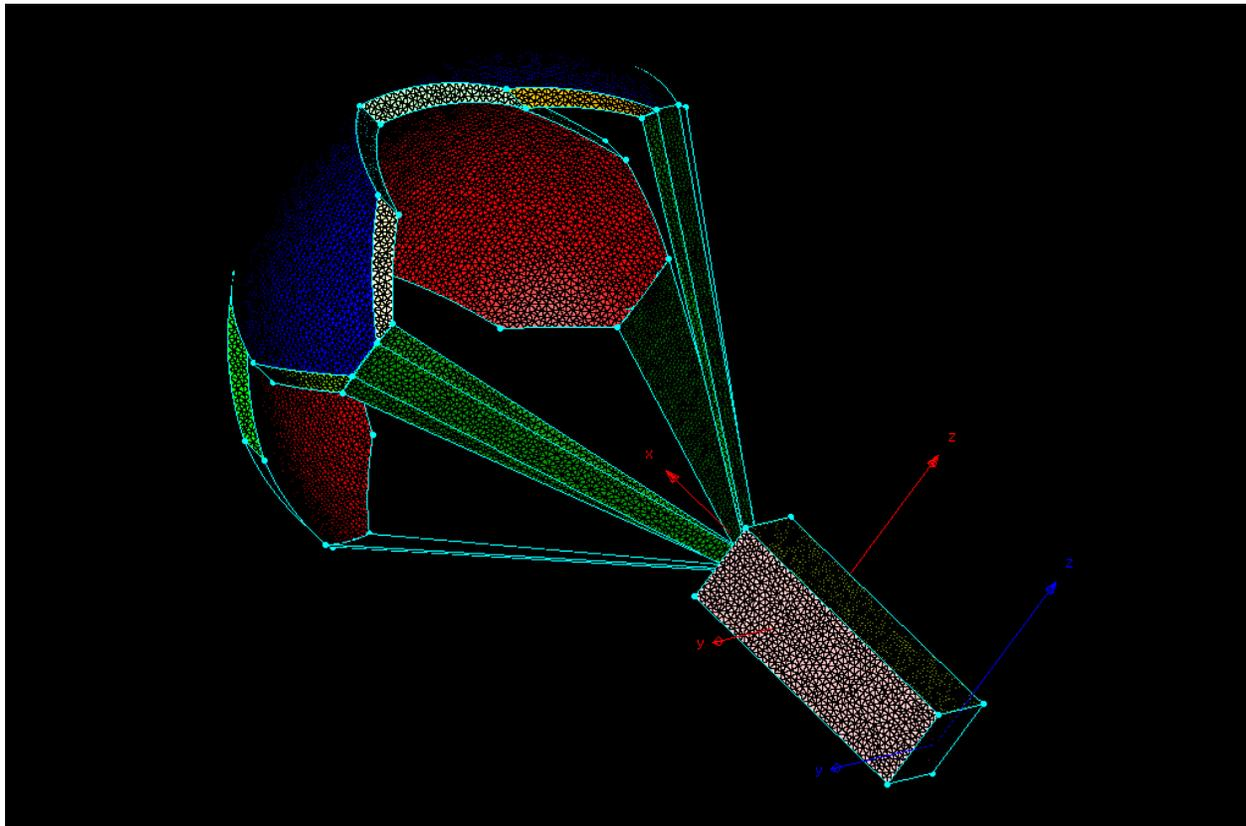
*Figure 31 Full TES-3p Mesh Created in Pointwise by Ben Nikaido*
