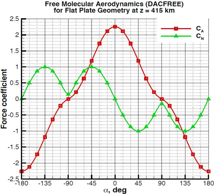
Figure 13 DACFREE for Flat Plate
