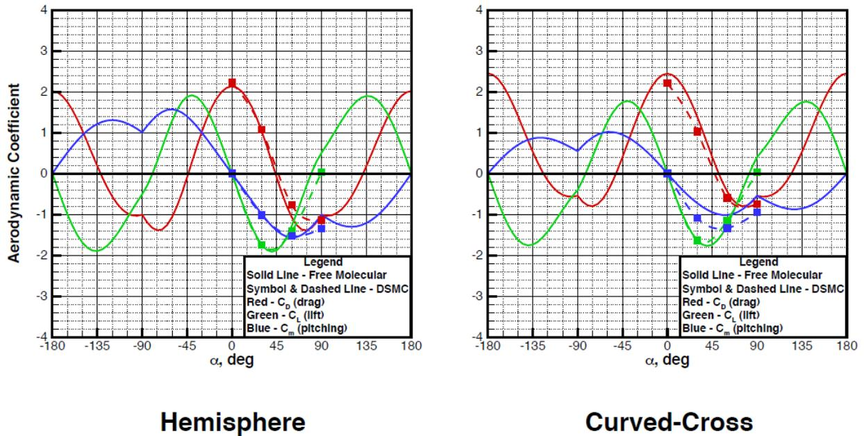
Figure 19 Aerodynamics at 200 km
