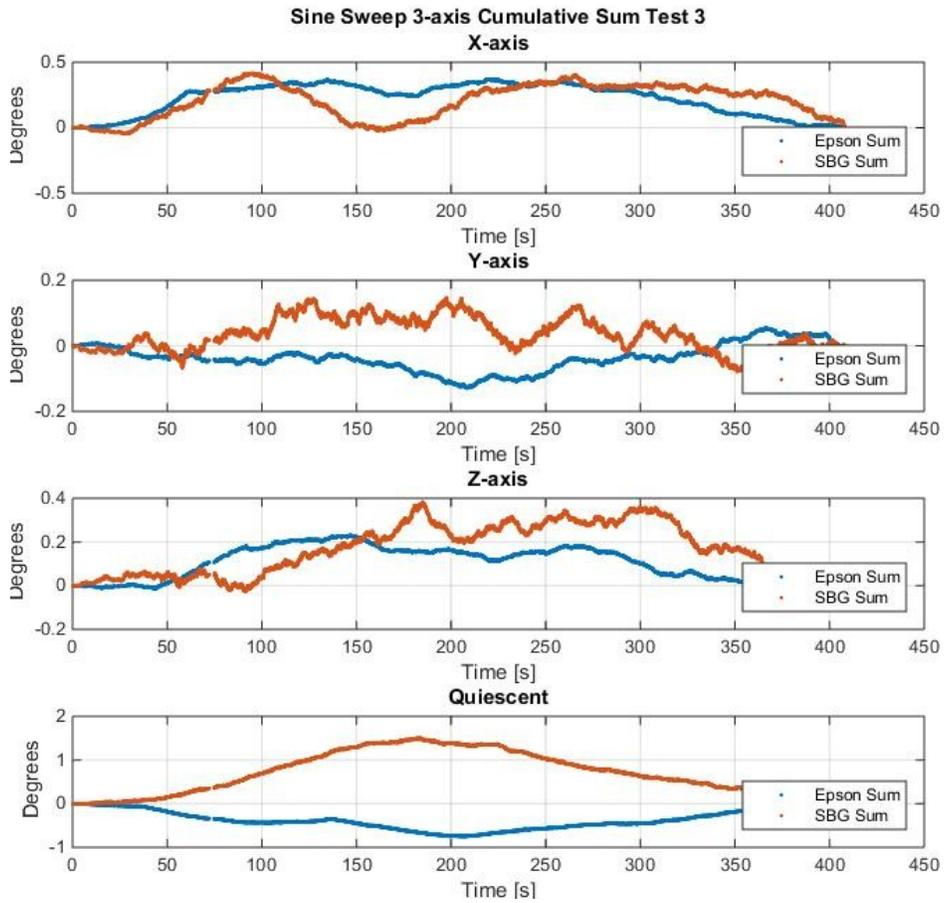
Figure C6: Integrated cumulative sum plots shown for both gyroscopes. The four plots here contain data from all three axes for the 3<sup>d</sup> Sine sweep test along with the quiescent data for comparison.
