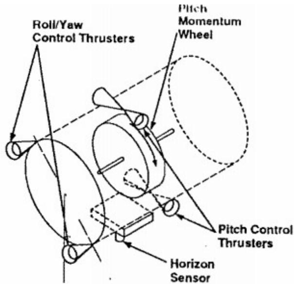
Figure 9: Single momentum-wheel and control thruster configurations can provide full 3-axis stabilization of a satellite.<sup>21</sup>
