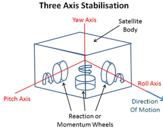
Figure 6: Illustration showing basic 3-axis stabilisation using momentum wheels<sup>19</sup>.
