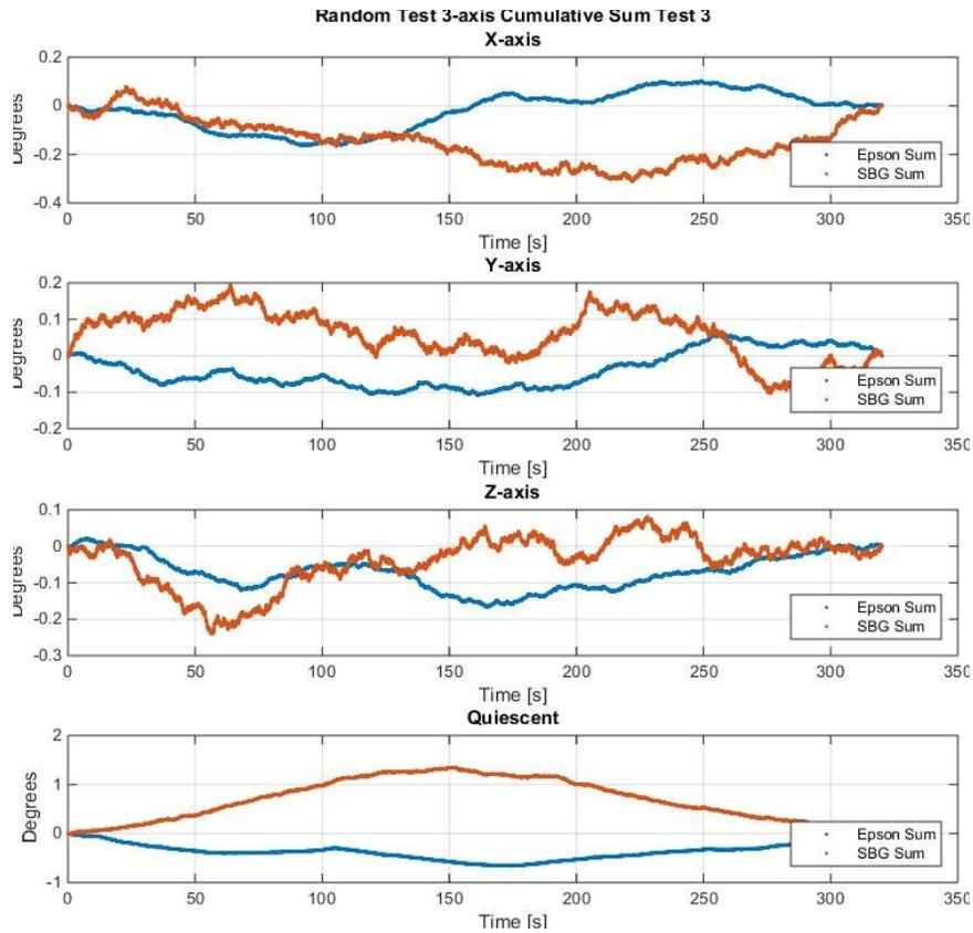
Figure C8: Integrated cumulative sum plots shown for both gyroscopes. The four plots here contain data from all three axes for the 3<sup>rd</sup> Random vibration test along with the quiescent data for comparison.
