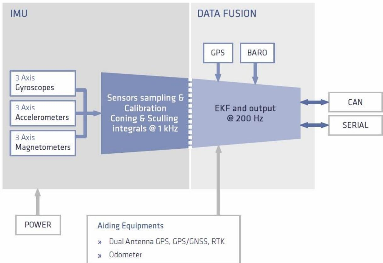
Figure 21: Simplified block diagram showing the internal filtering of the SBG Ellipse IMU.
