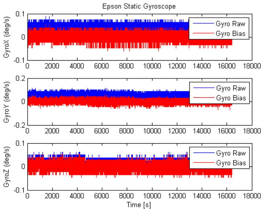
Figure 22: Static measurements from Epson gyroscope over a five hour test.
