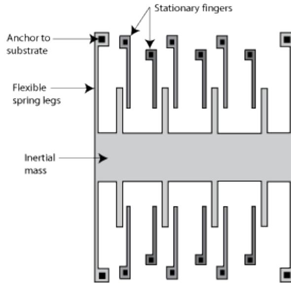
Figure 16: Illustration showing multiple masses aligned with parallel plates. More plates provide a higher degree of accuracy.<sup>26</sup>
