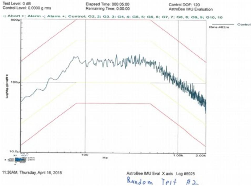
Random test of amplitude 0.21  $g_{rms}$
