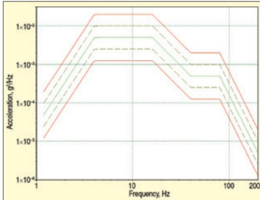
Figure 33: Sample random vibration PSD spectrum.<sup>26</sup>
