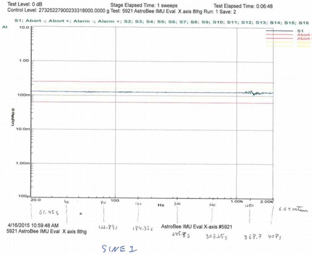
Figure 37: Sine sweep Test 1 of amplitude  $\frac{1}{8}$  grms
