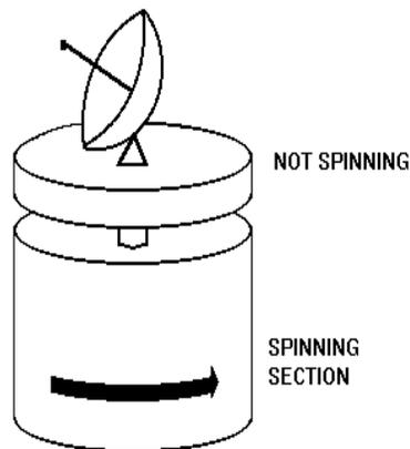
*Figure 1: Basic setup of a spin-stabilized satellite.*
