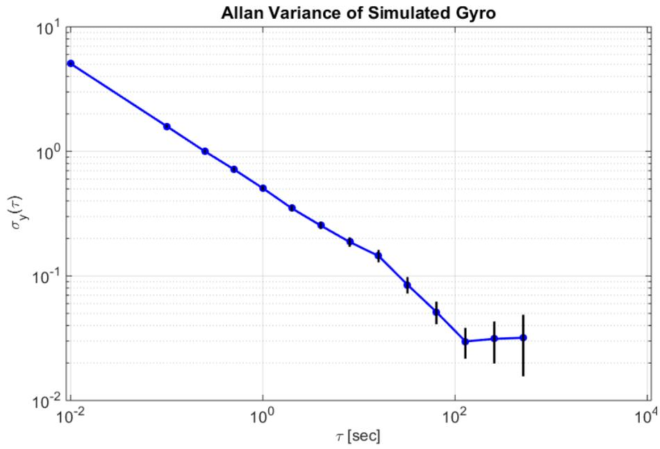
Figure 31: Allan Variance plot of the simulated gyroscope.
