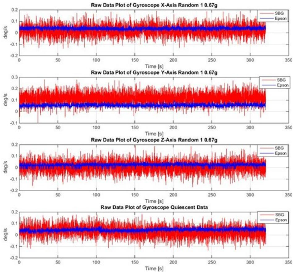
Figure 46: Raw data showing the results of the first Random Test for the Epson and SBG gyroscope across all three axes.
