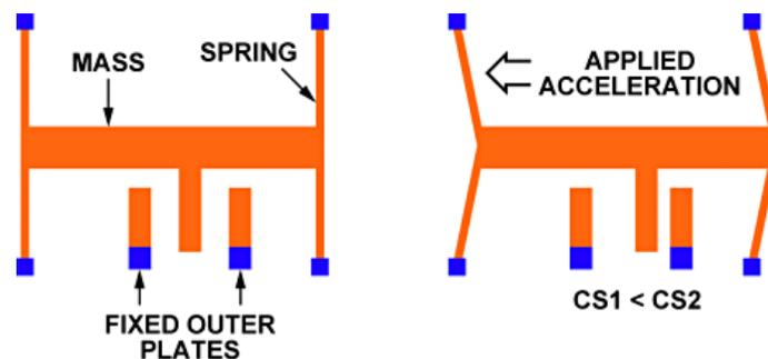
Figure 15: Illustration showing mass displacement in an accelerometer.<sup>26</sup>
