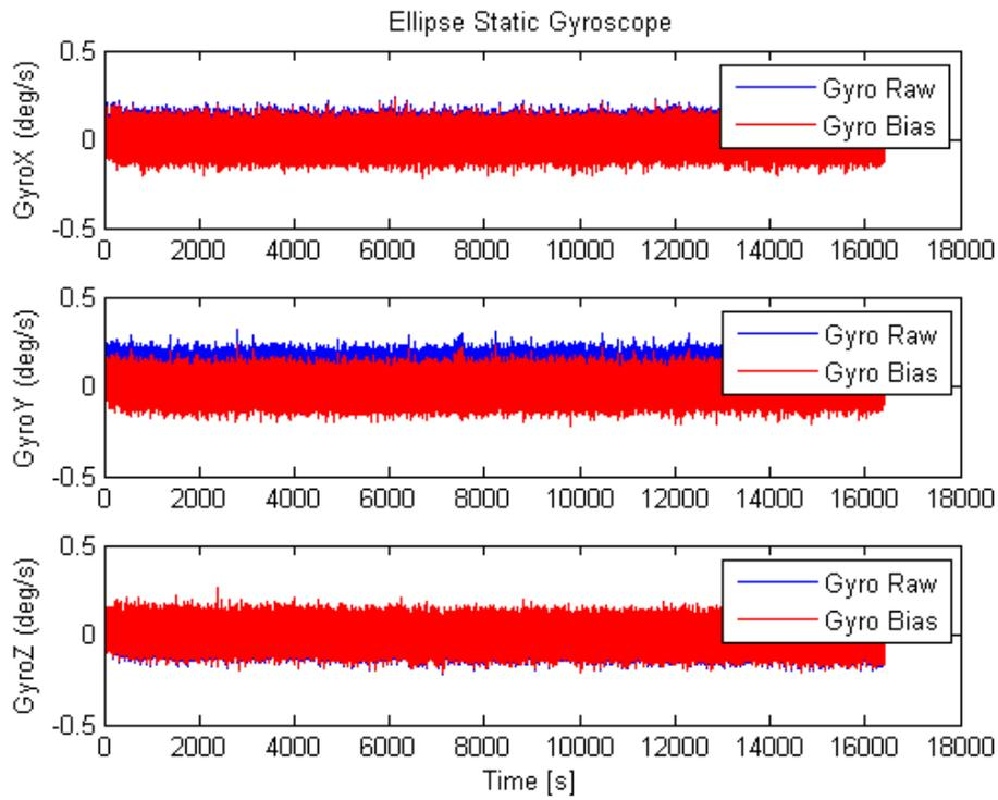
Figure 23: Static measurements from Ellipse gyroscope over a five hour test.
