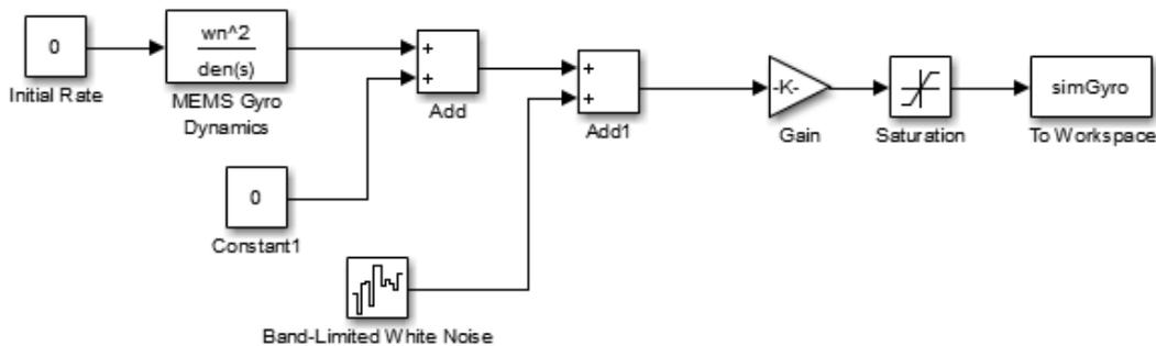
Figure 29: Simulink block diagram of the Epson gyroscope.
