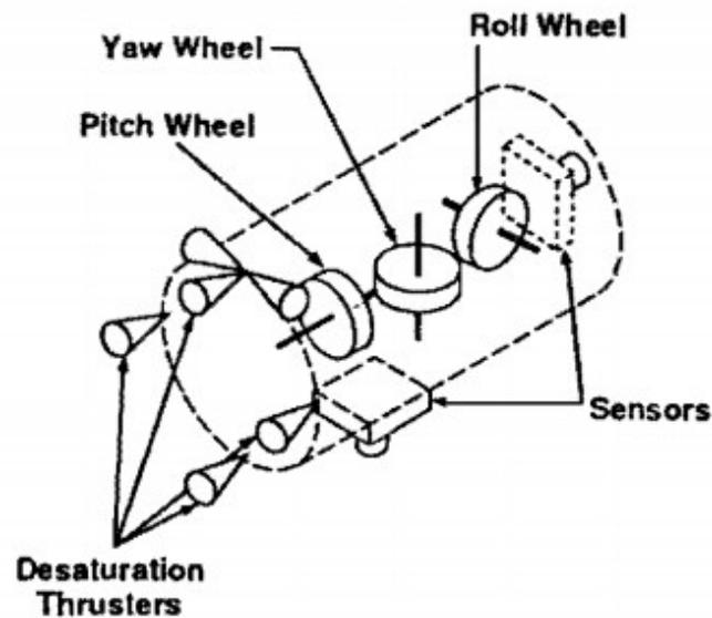
Figure 13: Three-wheel setup to provide full three-axis control and stabilization.<sup>21</sup>
