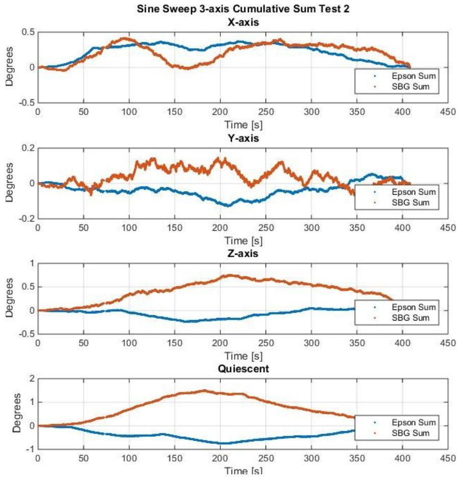
Figure C5: Integrated cumulative sum plots shown for both gyroscopes. The four plots here contain data from all three axes for the 2<sup>nd</sup> Sine sweep test along with the quiescent data for comparison.
