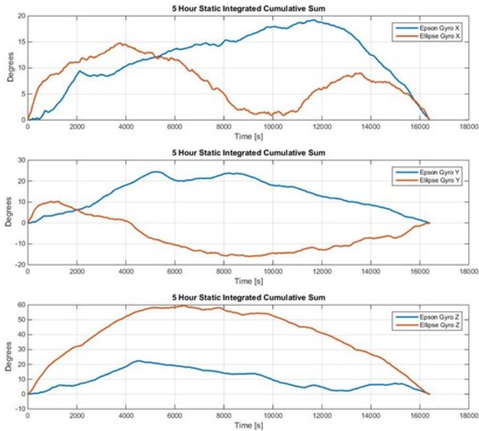
Figure 28: Cumulative sum from previous 5 hour static test.
