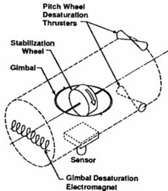
Figure 11: Single-gimbal configuration for a satellite.<sup>21</sup>
