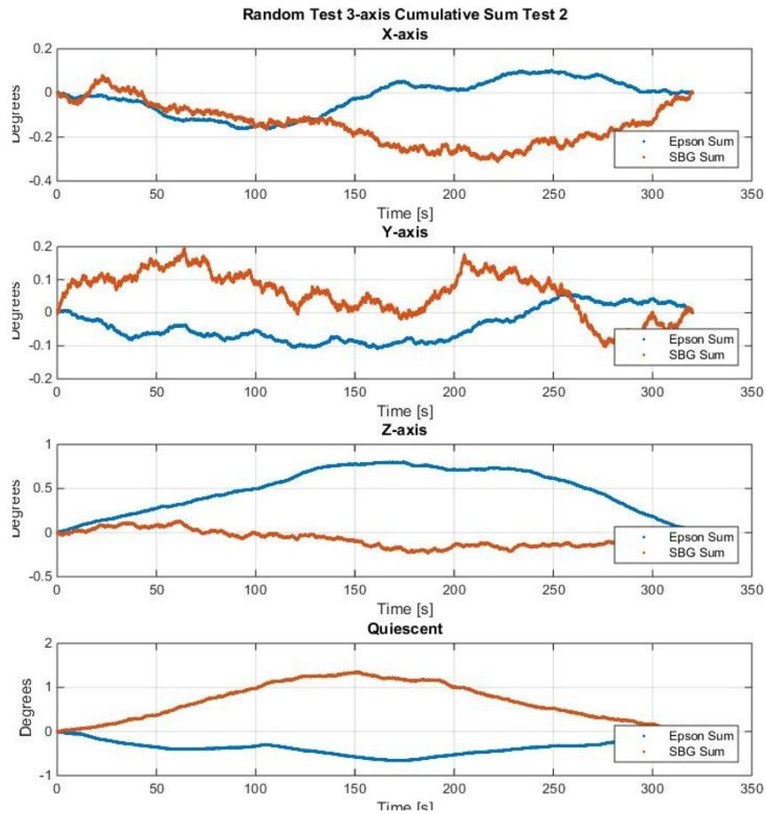
Figure C7: Integrated cumulative sum plots shown for both gyroscopes. The four plots here contain data from all three axes for the 2<sup>nd</sup> Random vibration test along with the quiescent data for comparison.
