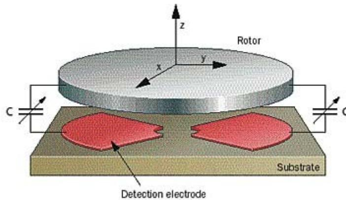
Figure 19: Rotating gyroscope configuration. Any external, off-axis force will result in a capacitance change detected by the electrode.<sup>26</sup>
