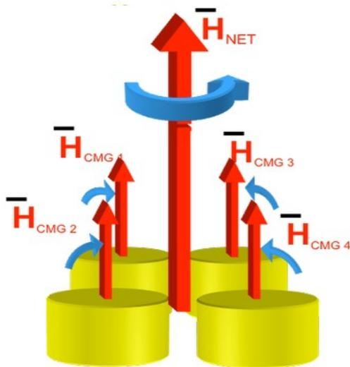
Figure 8: Once all CMGs are facing upwards, saturation is reached as no more torque can be generated.<sup>19</sup>
