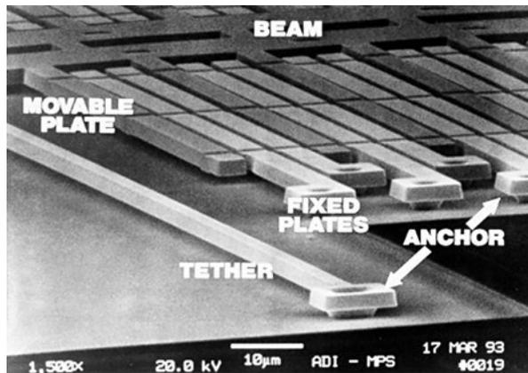
Figure 17: Zoomed-in picture of an actual accelerometer showing the plates and masses.<sup>26</sup>
