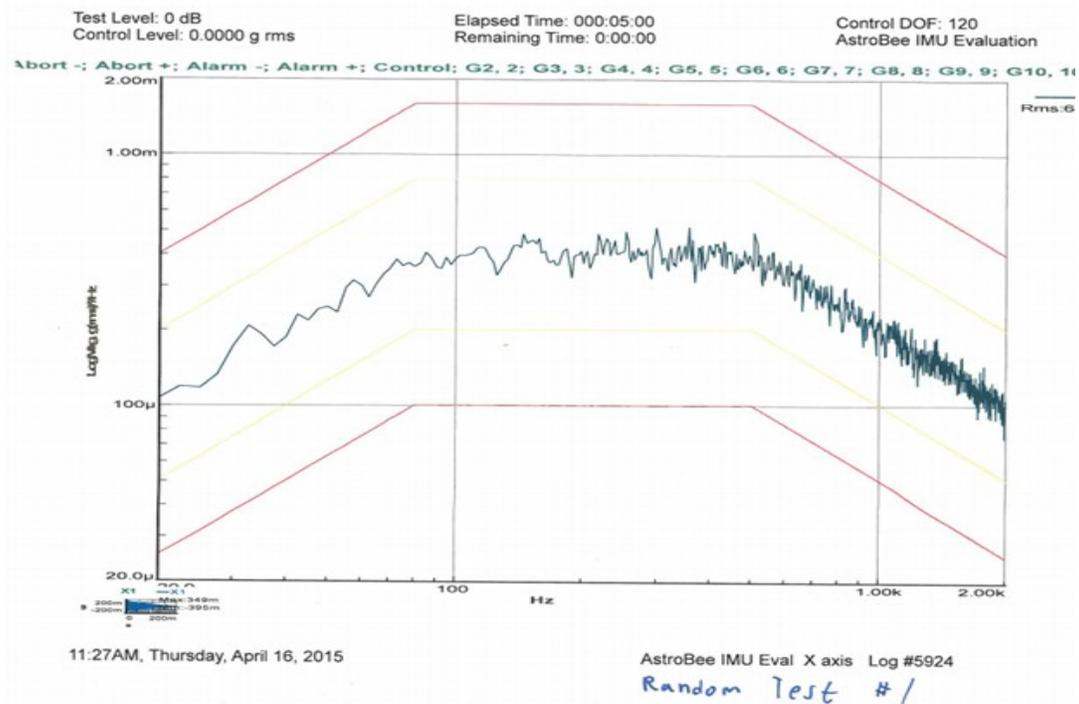
Figure 38: Random test of amplitude 0.67 grms.
