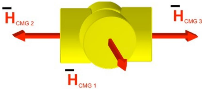
Figure 7: Null position of CMGs aboard the International Space Station.<sup>19</sup>
