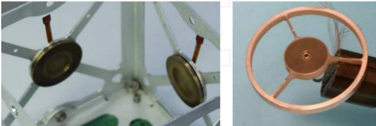
*Figure 4: Two types of reaction wheels can be see here, inside (left) and outside (right) of a satellite.*
