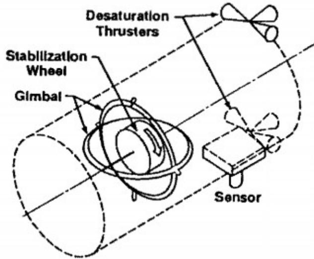
Figure 12: Double-gimbal setup with one momentum wheel.<sup>21</sup>
