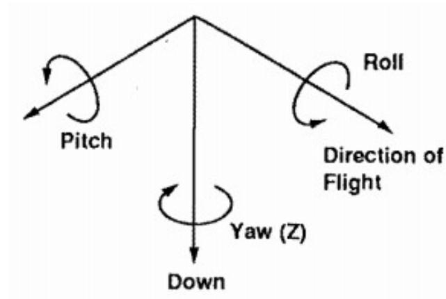
Figure 10: Simple illustration showing how the axes are aligned for the above configuration.<sup>21</sup>
