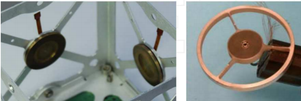
Figure 4: Two types of reaction wheels can be seen here, inside (left) and outside (right) of a satellite.
