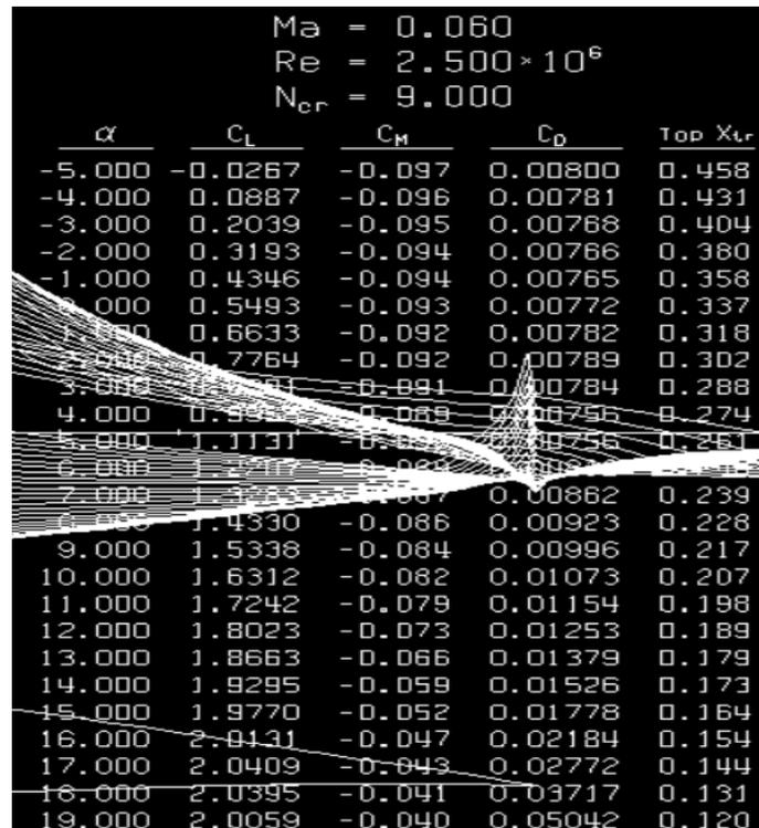
Figure 25. Eppler 1210 Xfoil Results
