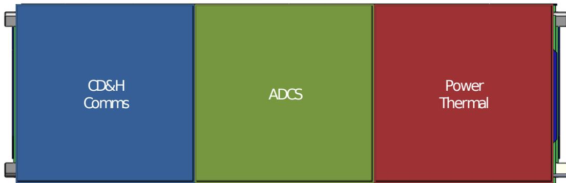
**Figure 10: RS Subsystem Volume Allocation**
