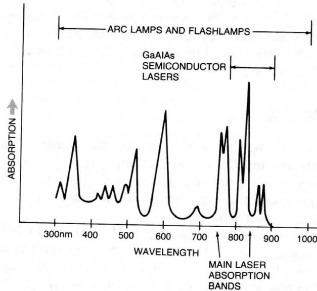
**Figure 3: Absorption spectrum of Nd 3+ ion** <sup>[5]</sup>
