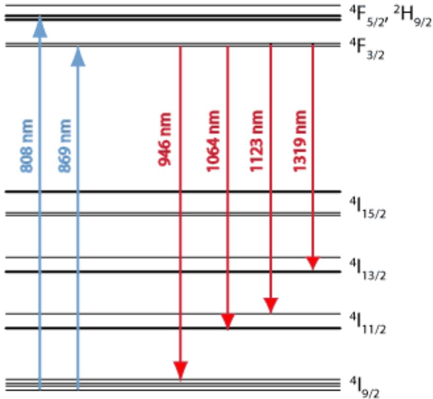
Figure 5: Energy level diagram of a Nd:YAG crystal<sup>[14]</sup>
