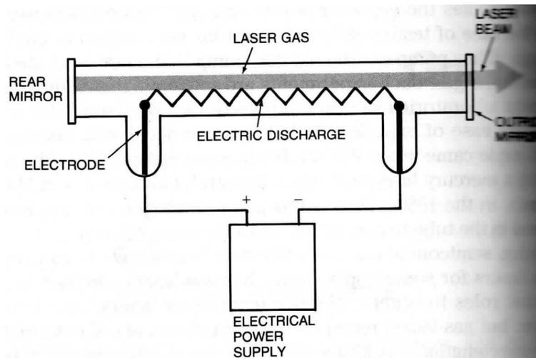
Figure 2: General Gas Laser design <sup>[5]</sup>
