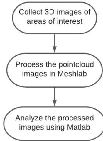
Figure 5.1: Flowchart of major steps in dent detection process
