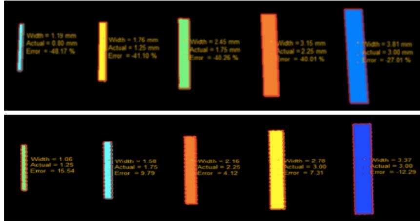
Figure 1.5: (Top) Results from edge detection method. (Bottom) Results from neural network method [40]
