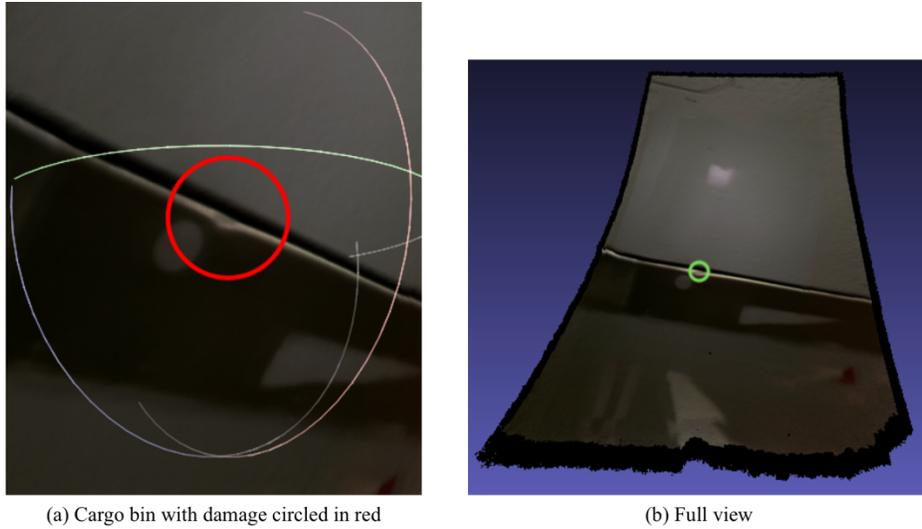
Figure 4.4: Damaged B737 cargo bin door
