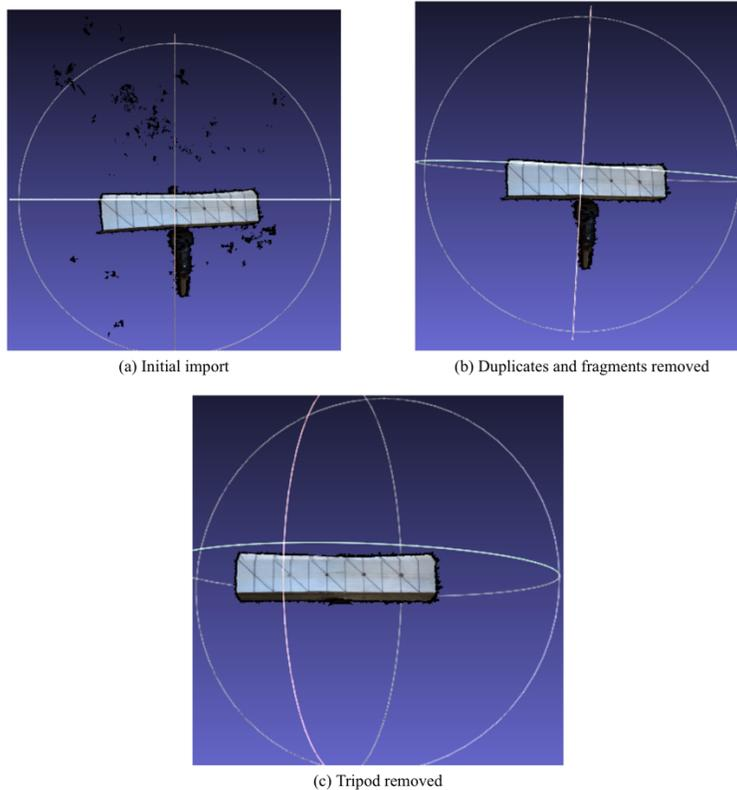
Figure 3.7: Example of image processing steps
