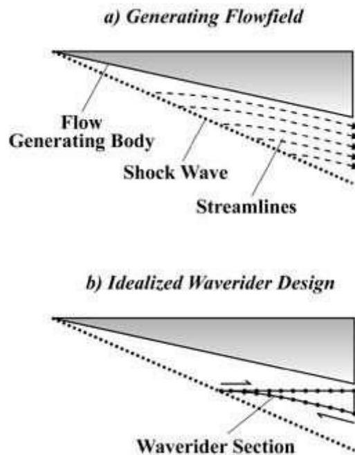
Figure 8: Waverider Creation from a Generating Flowfield [11]
