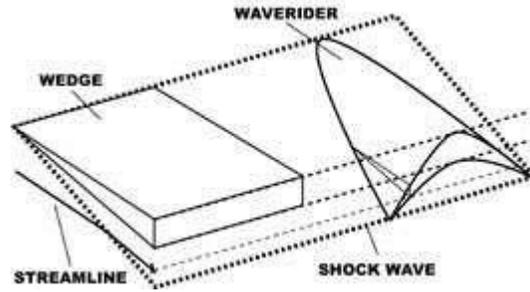
Figure 7: Wedge-Derived Waverider [11]
