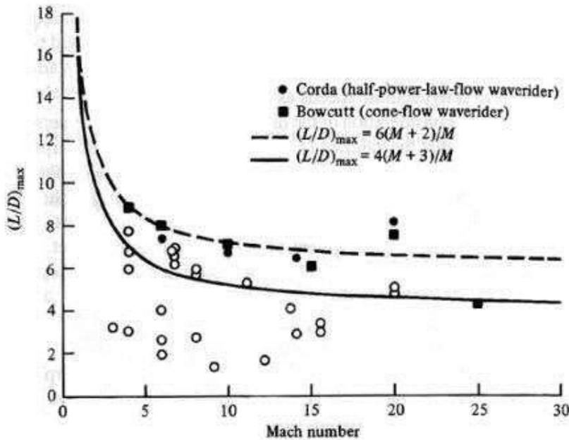
Figure 1: Maximum L/D Ratio Comparison for Various Hypersonic Configurations [4]
