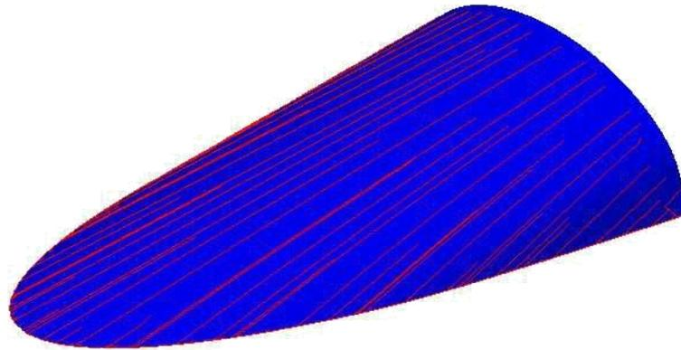
Figure 25: Waverider Streamlines
