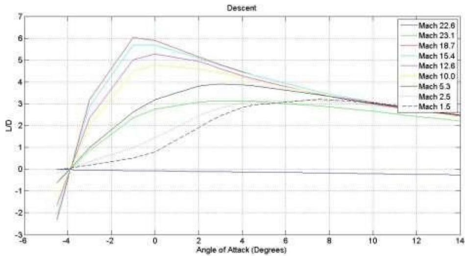
Figure 27: Descent L/D vs. Angle of Attack
