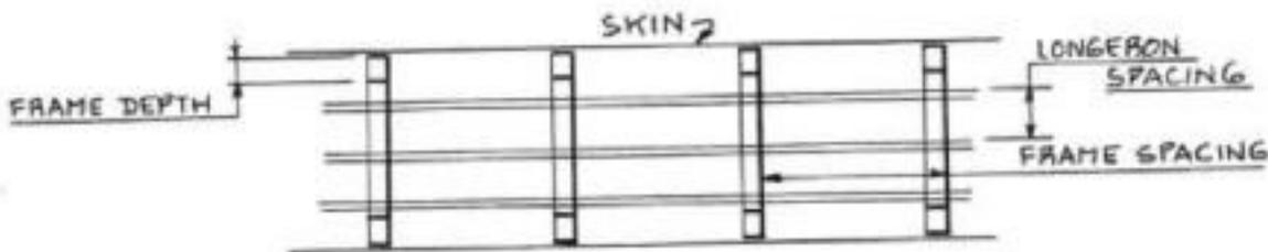
**Figure 12: Frame Depth, Frame Spacing, Longeron Spacing Diagram**
