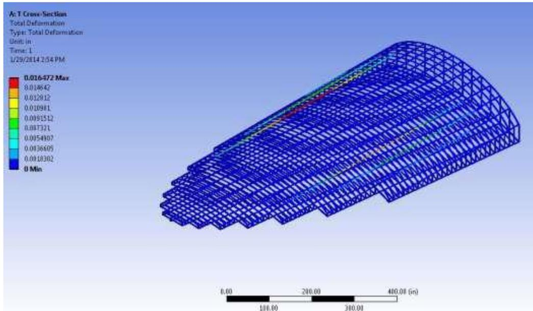
Figure 17: Total Deformation Structural Analysis From Hand Calculated Pressure.
