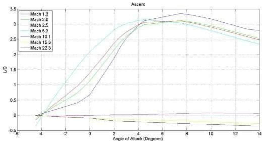
Figure 26: Ascent L/D vs. Angle of Attack
