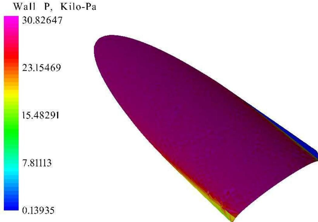
**Figure 29: Windward Pressure Visualization**
