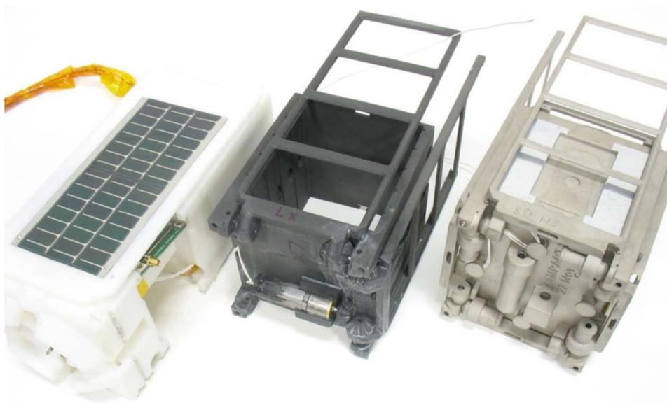
Figure 4: RAMPART CubeSat at Various Design Stages
