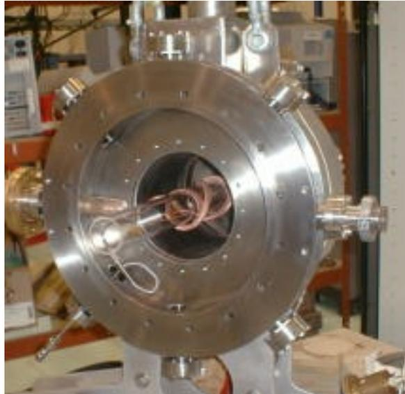
Figure 17 Actual Helicon antenna Source: Baity, 2003
