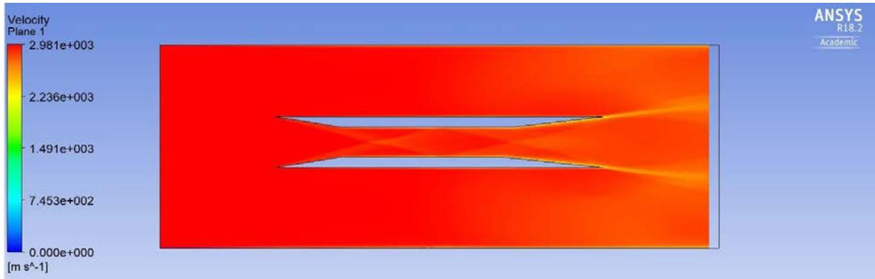
Figure 43: Internal inlet velocity contour at M=8
