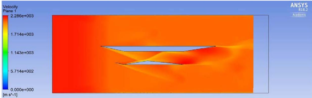
Figure 34: External inlet velocity contour at M=6
