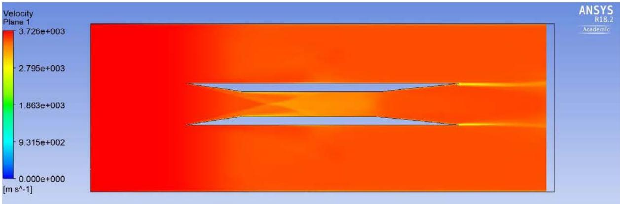
Figure 44: Internal inlet velocity contour at M=10
