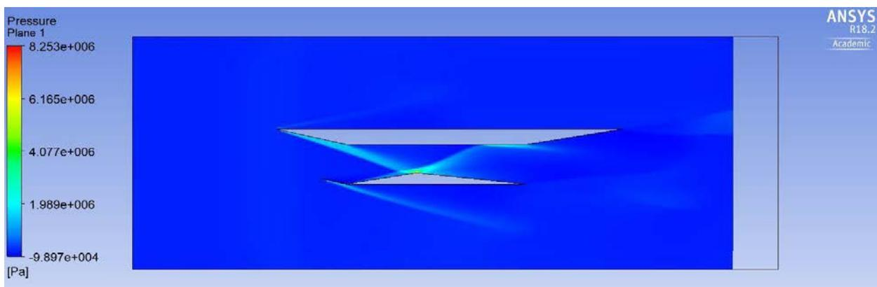
Figure 23: External inlet pressure contour at M=8
