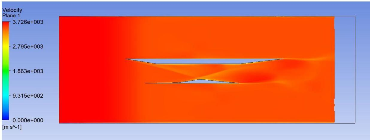
Figure 40: Internal and external inlet velocity contour at M=10
