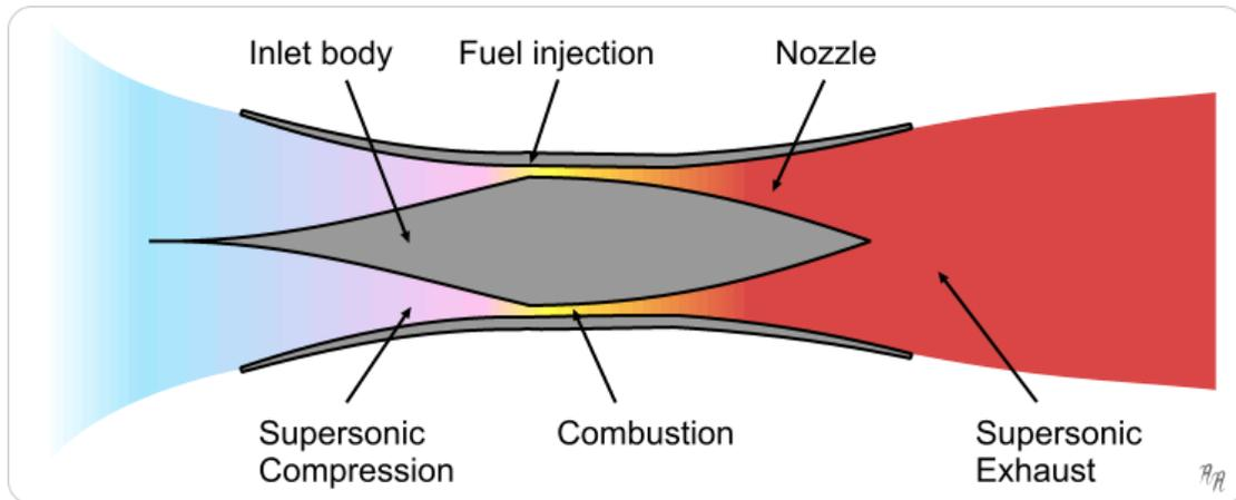
*Figure 1: Scramjet engine model*
