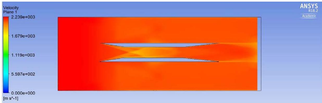
Figure 42: Internal inlet velocity contour at M=6
