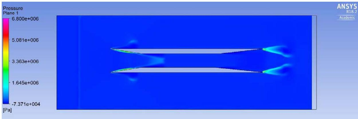
Figure 33: Internal inlet pressure contour at  $M=12$
