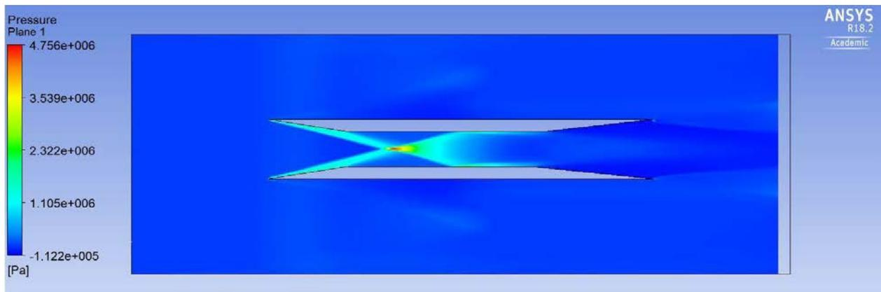
Figure 32: Internal inlet pressure contour at  $M=10$
