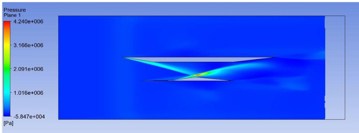
Figure 28: Internal and External inlet pressure contour at M=10
