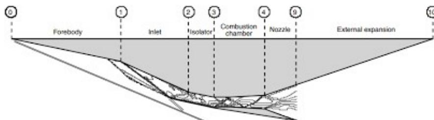
Figure 19: Flow stations in a Scramjet engine
