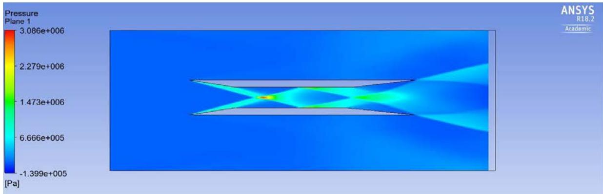
Figure 31: Internal inlet pressure contour at  $M=8$
