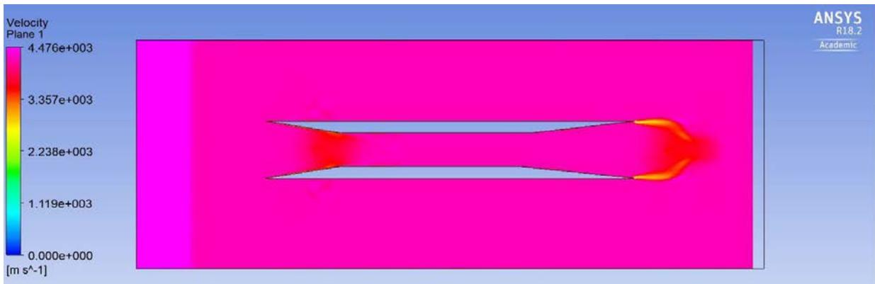
Figure 45: Internal inlet velocity contour at M=12
