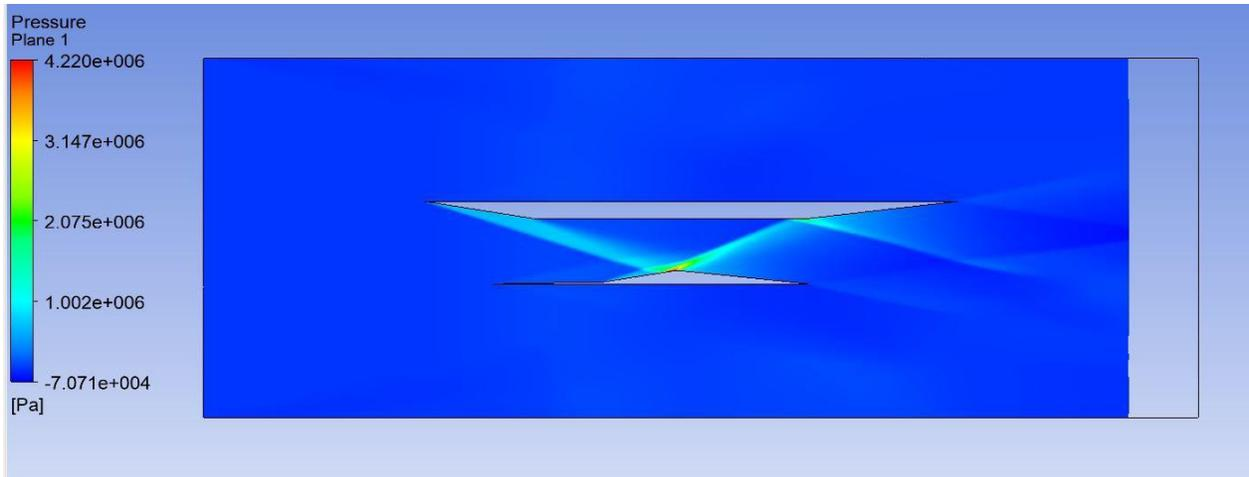
Figure 26: Internal and External inlet pressure contour at M=6
