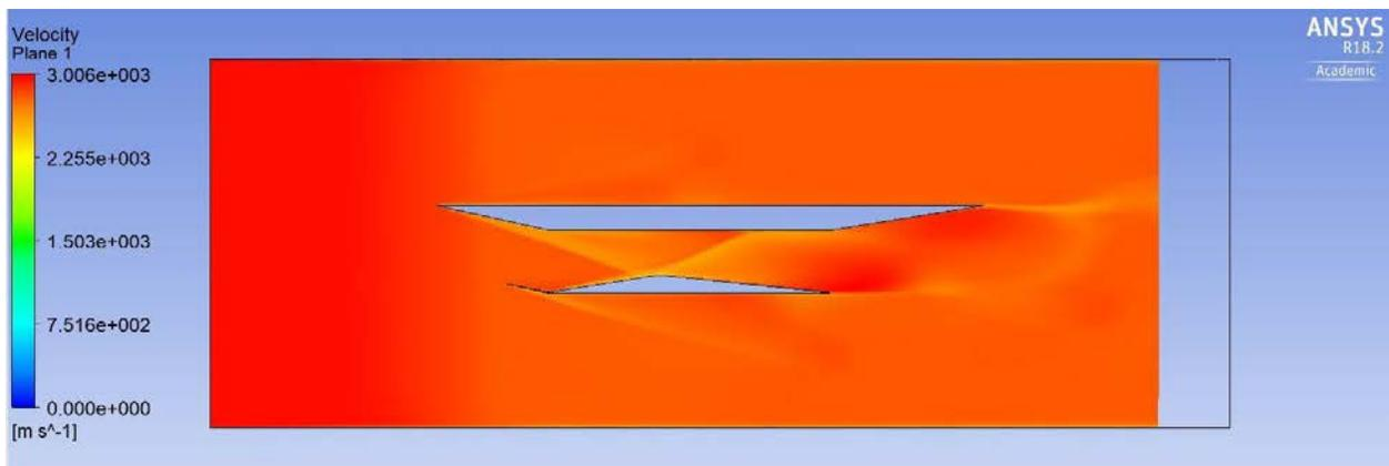
Figure 35: External inlet velocity contour at M=8
