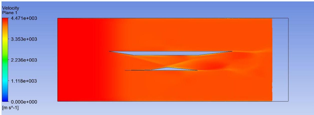
Figure 41: Internal and external inlet velocity contour at M=12
