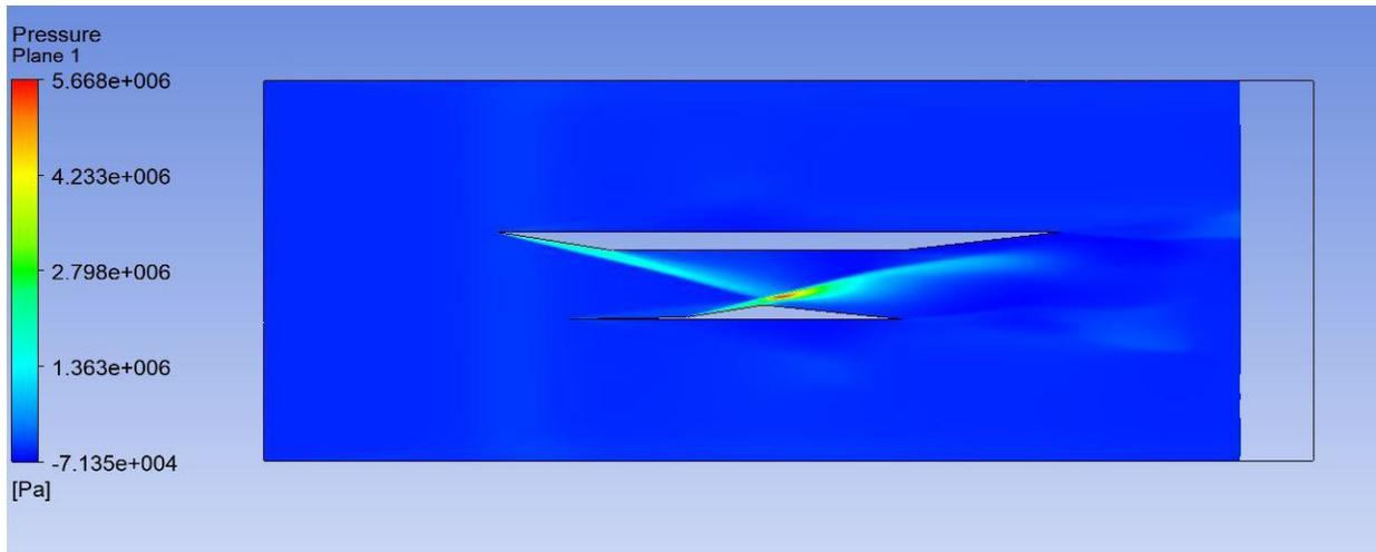
Figure 29: Internal and External inlet pressure contour at  $M=12$
