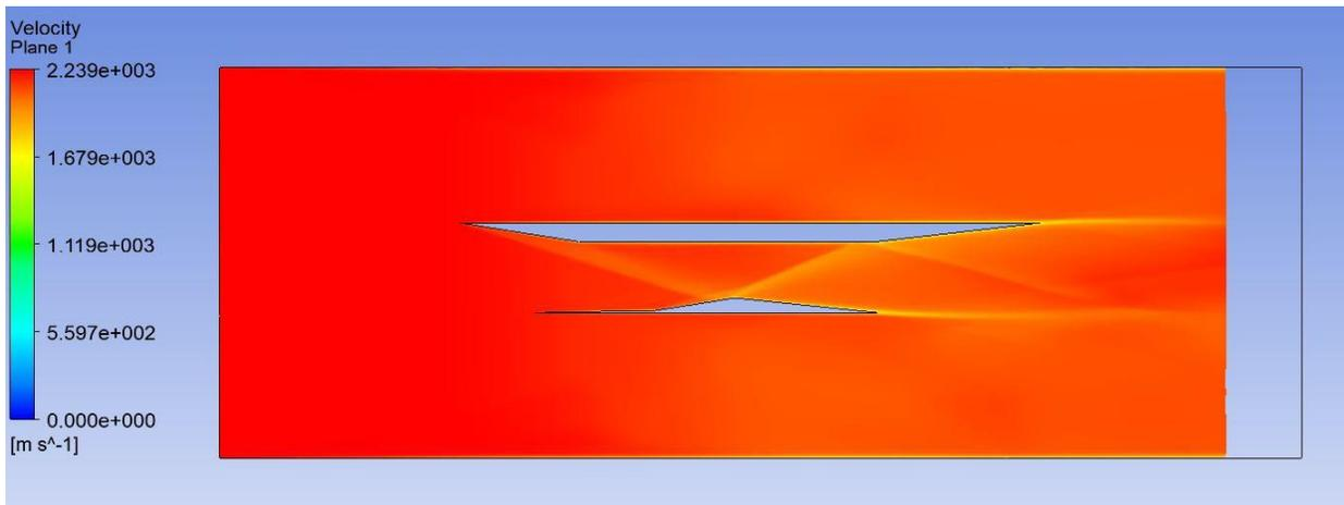
Figure 38: Internal and external inlet velocity contour at M=6
