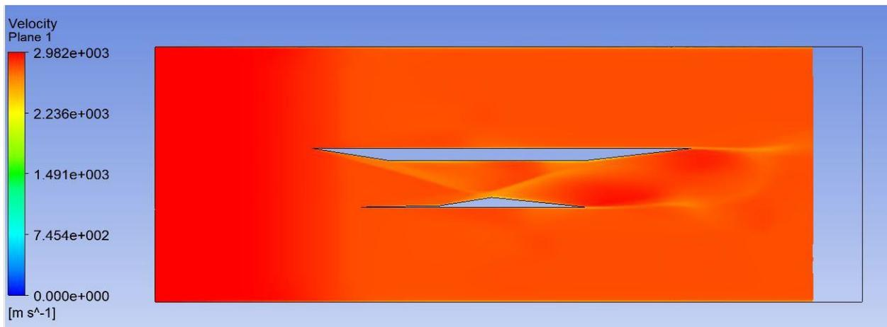
Figure 39: Internal and external inlet velocity contour at M=8
