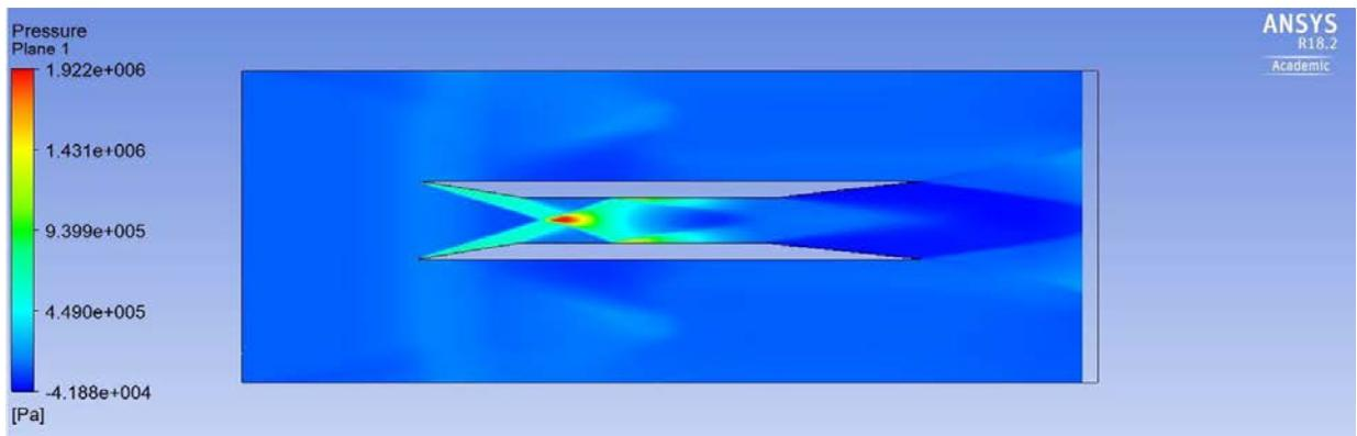
Figure 30: Internal inlet pressure contour at  $M=6$
