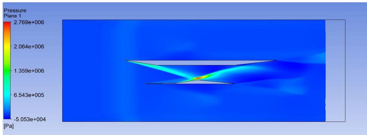
Figure 27: Internal and External inlet pressure contour at M=8
