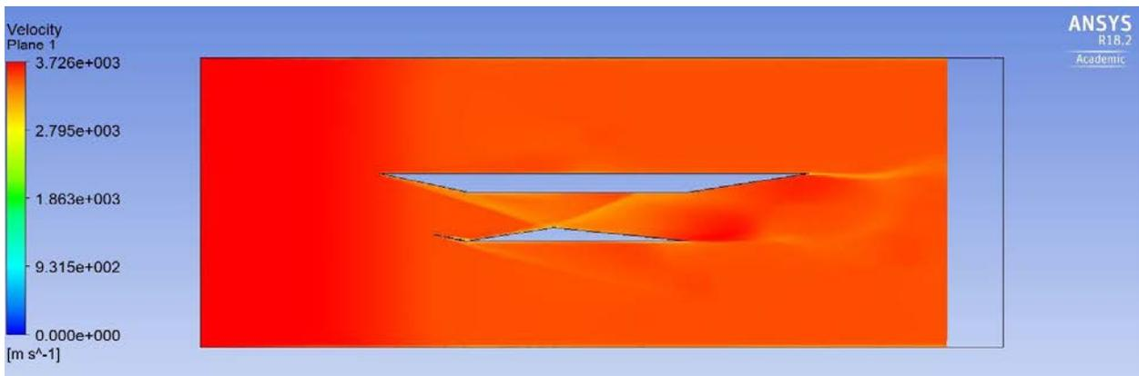
Figure 36: External inlet velocity contour at M=10
