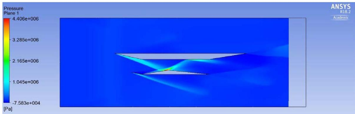
Figure 22: External inlet pressure contour at M=6
