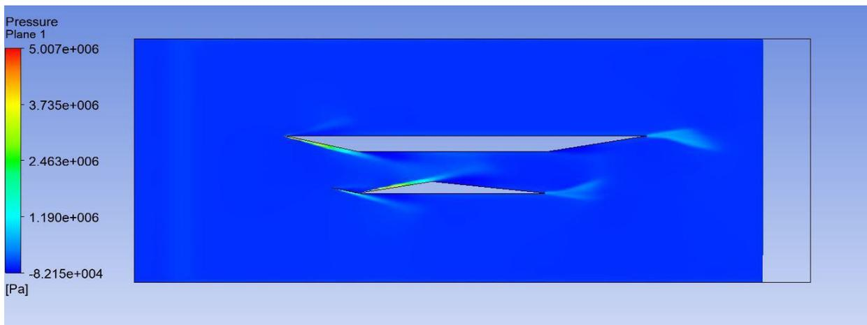
Figure 25: External inlet pressure contour at M=12
