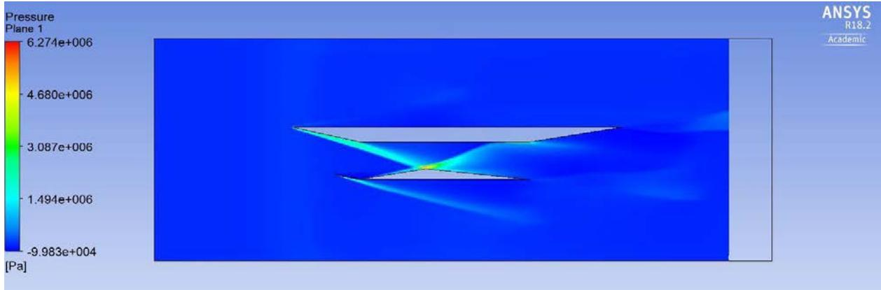
Figure 24: External inlet pressure contour at M=10
