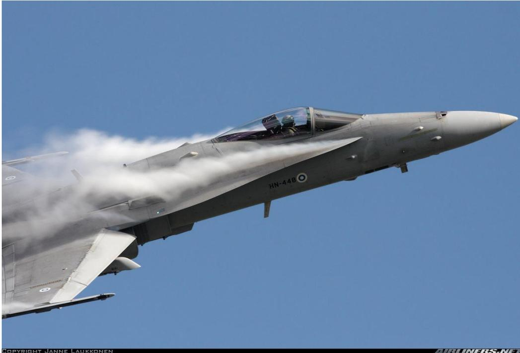
Figure 2.3: Vortex Generated by LERX on a F/A-18.
