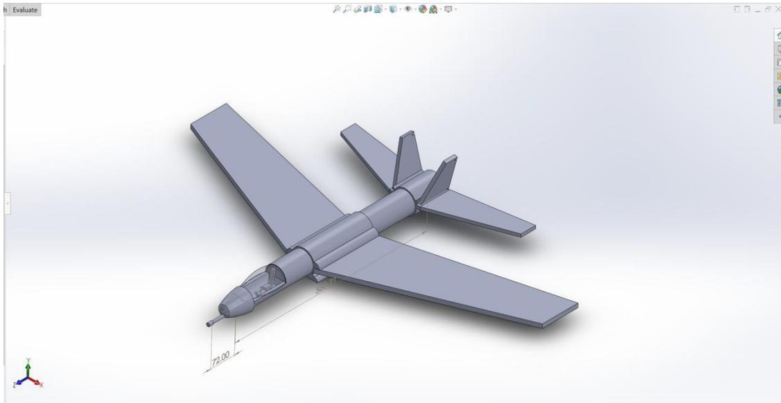
Figure 2.7g: CAD Drawing of Fuselage, Wing, and Empennage.
