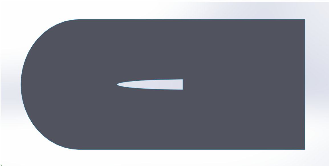
Figure 3.12 – Geometry and domain of long ellipsoid 7:1.
