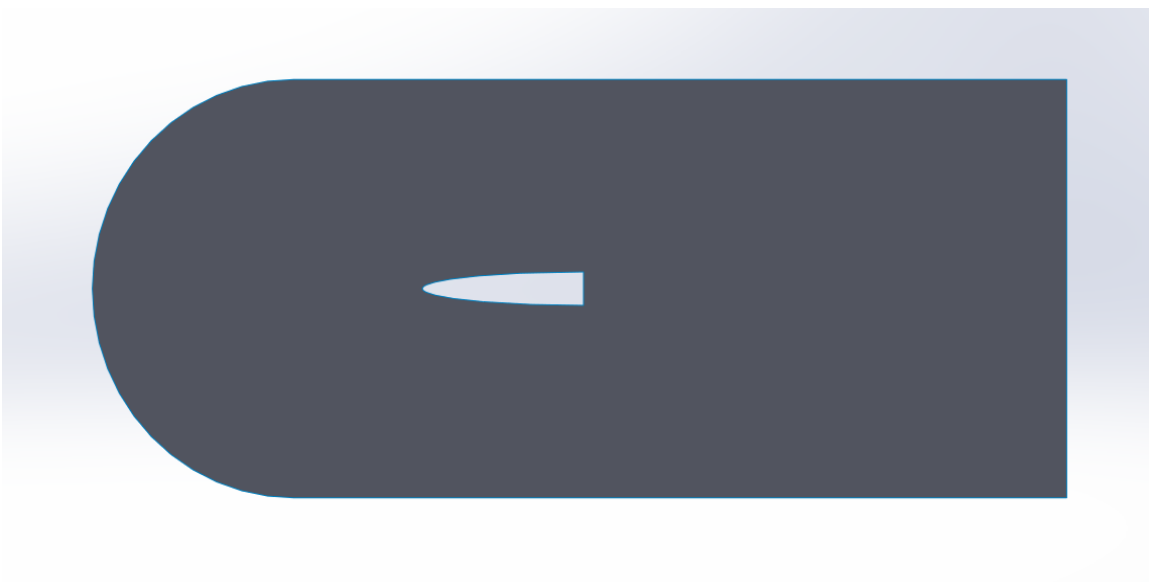
Figure 3.10 – Geometry and domain of long ellipsoid 5:1.
