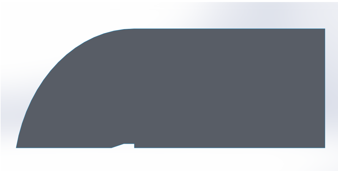
Figure 3.14 – Geometry and domain of clipped delta fin at 15 degrees.
