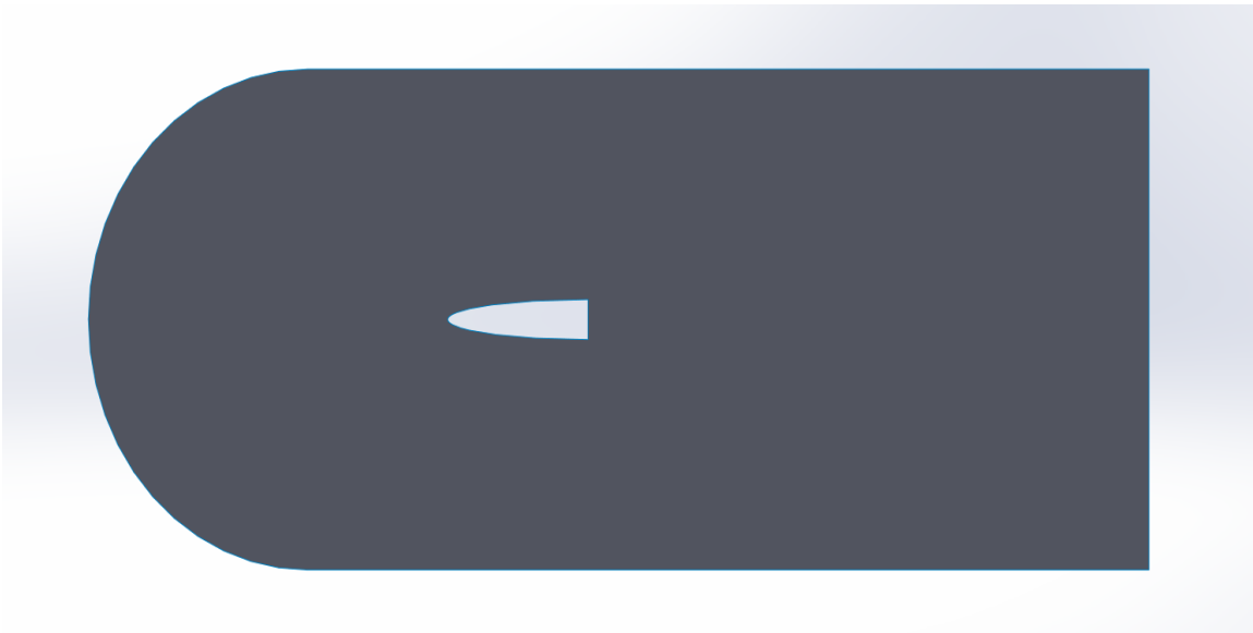
Figure 3.9 – Geometry and domain of long ellipsoid 4:1.
