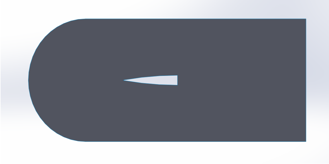
Figure 3.3 – Geometry and domain of ogive 6:1.
