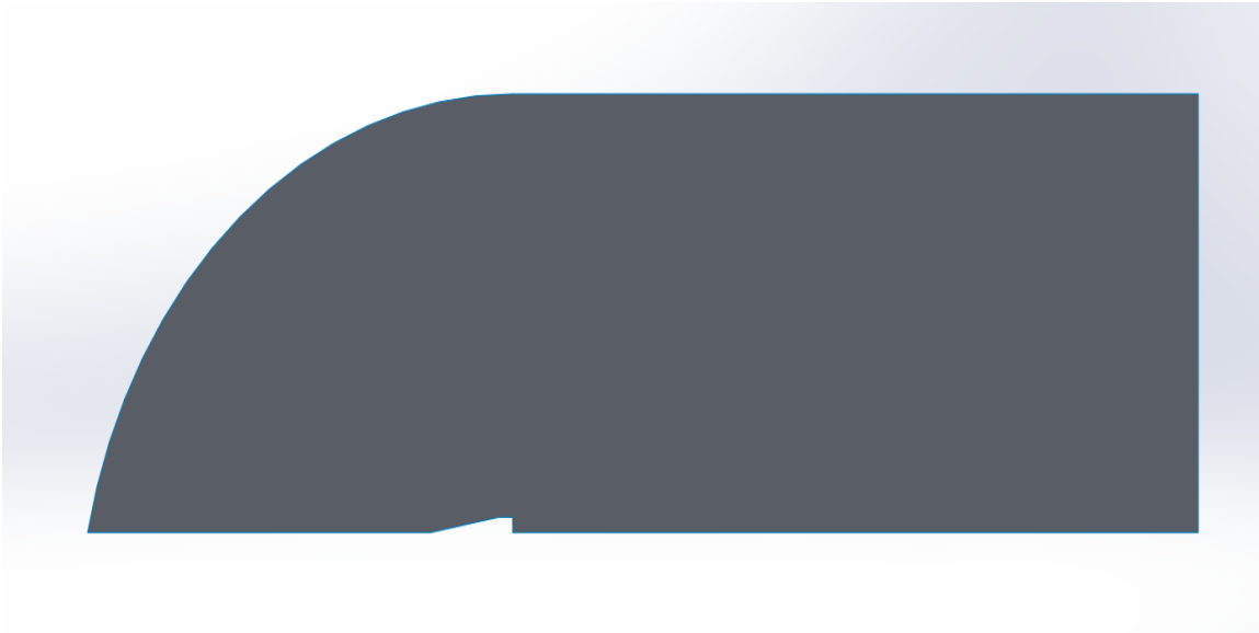
Figure 3.13 – Geometry and domain of clipped delta fin at 10 degrees.
