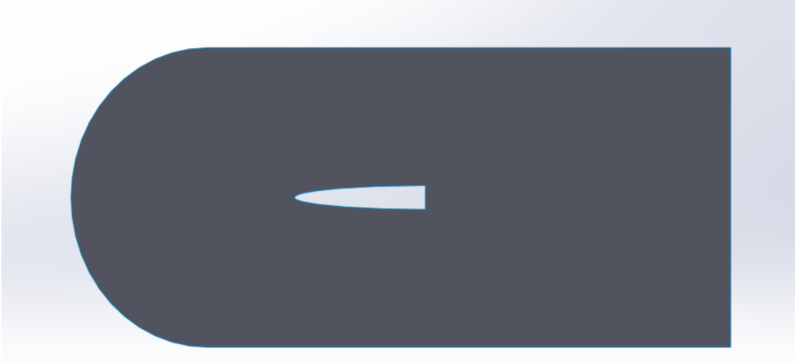
Figure 3.11 – Geometry and domain of long ellipsoid 6:1.
