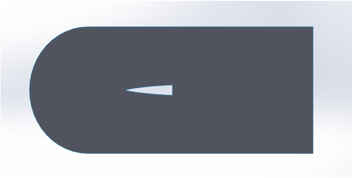
Figure 3.7 – Geometry and domain of von Karman 5:1.
