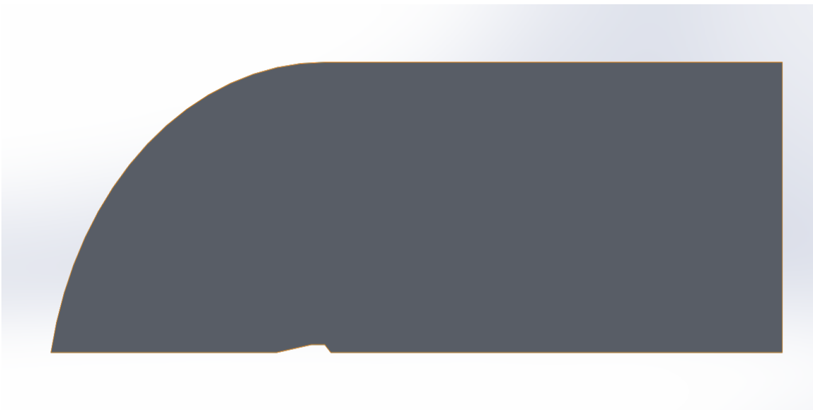
Figure 3.15 – Geometry and domain of trapezoidal fin at 10 degrees.
