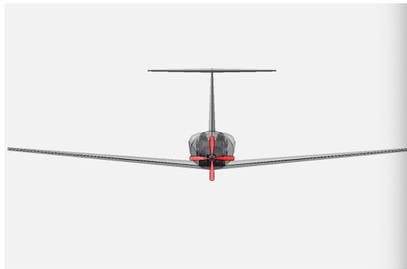
Figure 4.5: Low-wing design of the proposed aircraft
