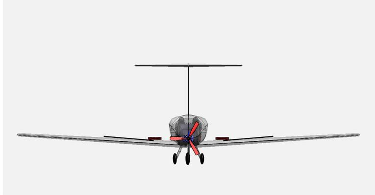
Figure 8.14: Front view of the proposed aircraft with landing gear disposition
