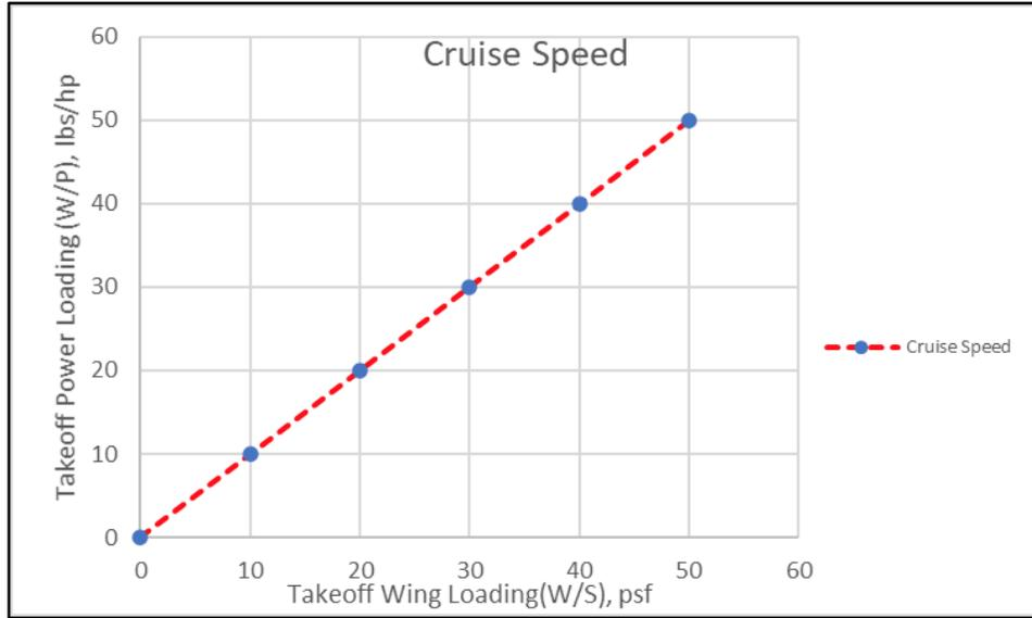
Figure 3.14: Allowable W/S and W/P to meet a given cruise speed
