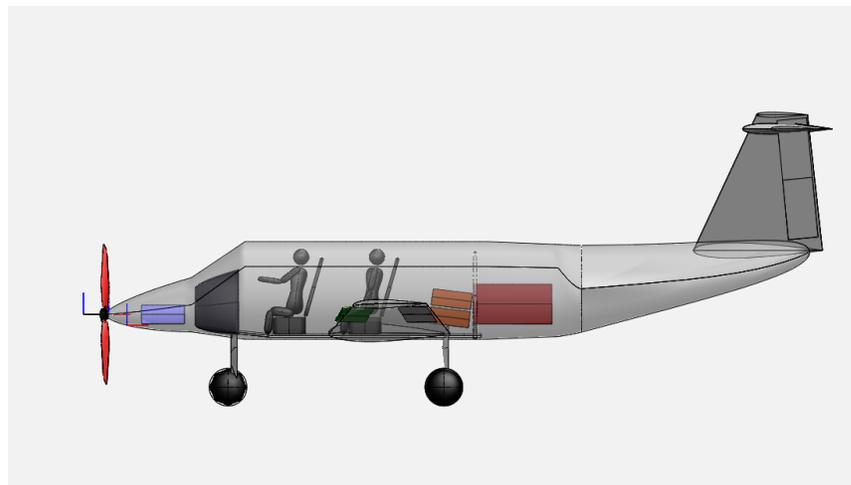
Figure 8.15: Side view of the proposed aircraft
