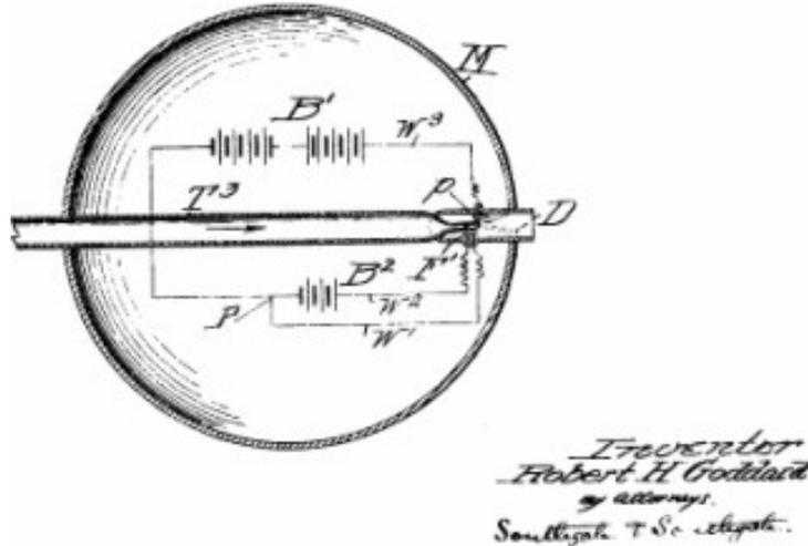
Figure 1: The figure shows the third variation of Goddard’s electrostatic ion accelerator from 1917.
