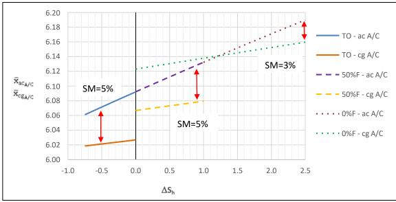
Figure 98. X-plot for change in horizontal area
