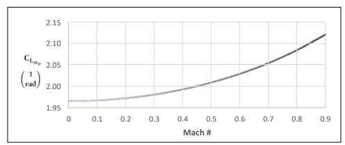
Figure 101. Mach number effect on vertical fin lift-curve slope
