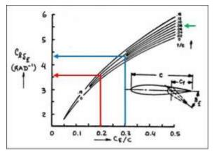
Figure 63. Effect of thickness ratio and flap chord ratio on  $c_{l,\delta f}$  [19]
