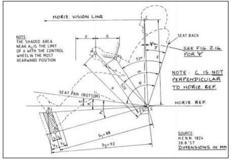
Figure 42. Recommended seat arrangement [20]
