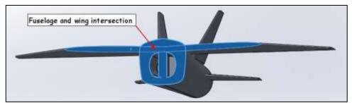
Figure 123. AMT, cut at wing-fuselage intersection
