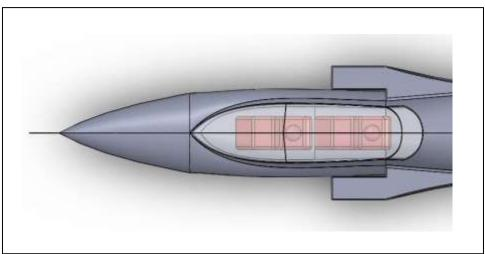
Figure 44. Cockpit cutaway top view
