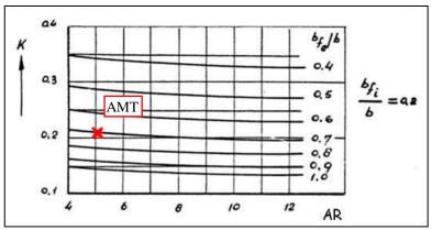
Figure 109. Interrupted flap induced drag factor [24]
