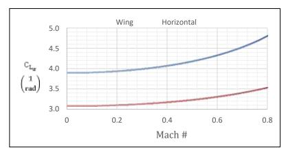
Figure 94. Change in wing and horizontal lift-curve slope due to Mach number
