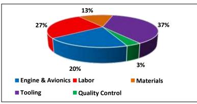
Figure 134. Prototype test airplanes cost percentages
