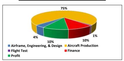
Figure 137. Manufacturing and acquisition cost percentages
