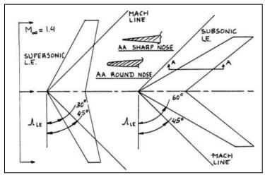
Figure 112. Definition of supersonic and subsonic leading-edge [24]
