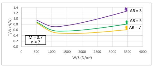
Figure 20. Maneuvering performance sizing graph
