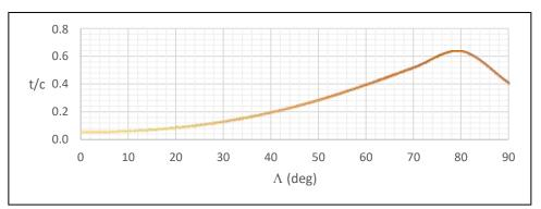
Figure 52. Wing sweep versus airfoil thickness ratio
