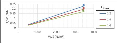
Figure 13. Takeoff distance performance sizing graph
