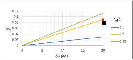
Figure 66. Effect of  $\delta_{nf}$  and  $c_{nf}/c$  on  $\Delta c_{l}$
