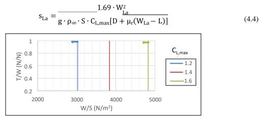
Figure 14. Landing distance performance sizing graph
