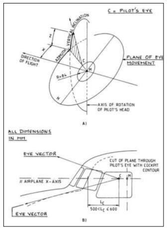
Figure 41. Definition of radial eye vectors [20]
