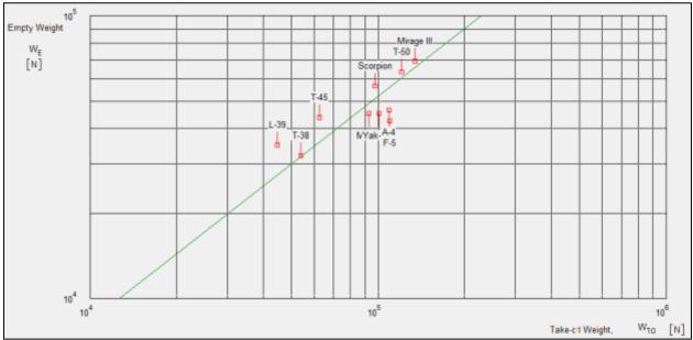
Figure 7. AAA – LogLog plot of comparable aircraft for  $W_{\rm E}$  and  $W_{\rm TO}$
