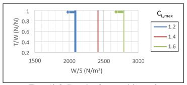
Figure 12. Stall speed performance sizing graph
