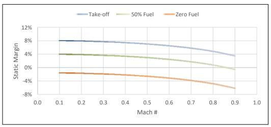
Figure 96. Effect of Mach number on static margin
