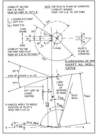
Figure 40. Port and starboard visibility requirements [20]
