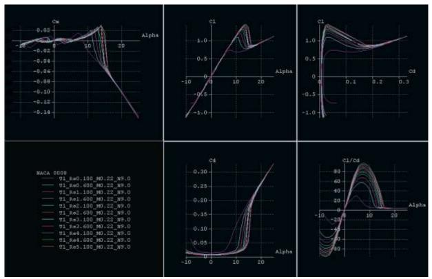
Figure 57. NACA 0008 coefficient polars from XFLR5
