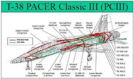
Figure 140. T-38 structure upgrades [44]
