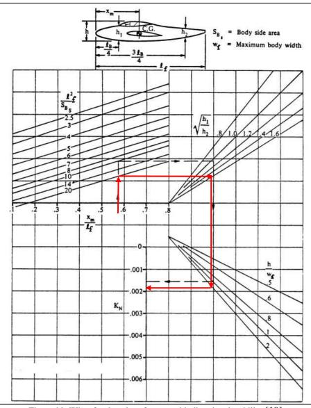
Figure 99. Wing-fuselage interference with directional stability [19]
