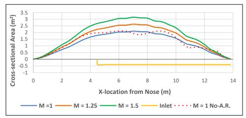
Figure 126. AMT's cross-sectional area distributions
