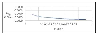
Figure 102. Mach effect on change in yawing moment wrt sideslip angle
