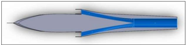
Figure 50. Preliminary engine intake ducts
