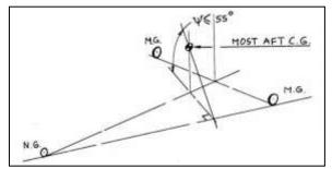
Figure 84. Tricycle gear lateral tip-over criterion [19]
