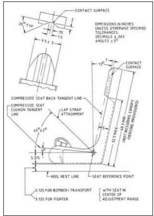
Figure 38. Typical ejection seat dimensions [20]
