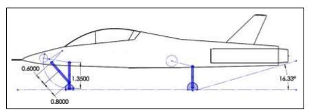
Figure 87. Side view of landing-gear
