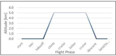
Figure 4. Basic flight profile
