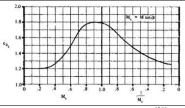
Figure 120. Steady-state cross flow drag coefficient [29]
