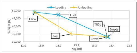
Figure 82. X<sub>cg</sub> travel from ref. point for different loading scenarios
