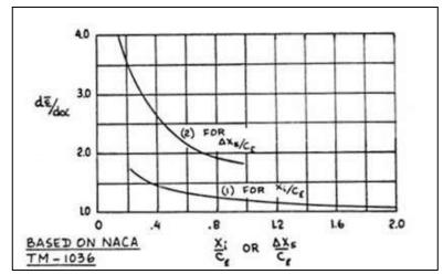
Figure 91. Effect of fuselage (or nacelle) segment location on upwash gradient [24]
