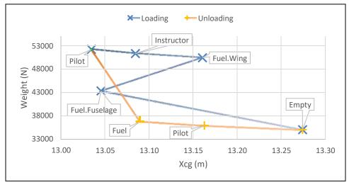
Figure 130.  $X_{cg}$  travel for Class II W&B from reference point for different loading scenarios
