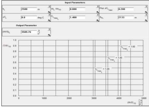
Figure 23. AAA – Landing distance T/W versus W/S
