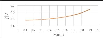
Figure 95. Change in tail downwash due to Mach number
