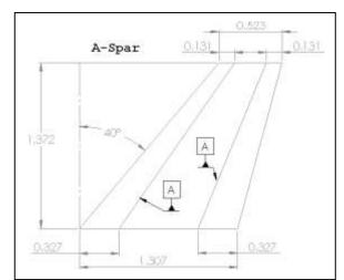
Figure 74. Horizontal stabilizer geometry drawing, units in meters
