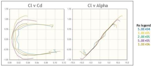
Figure 55. NACA 0008 aerodynamic polars
