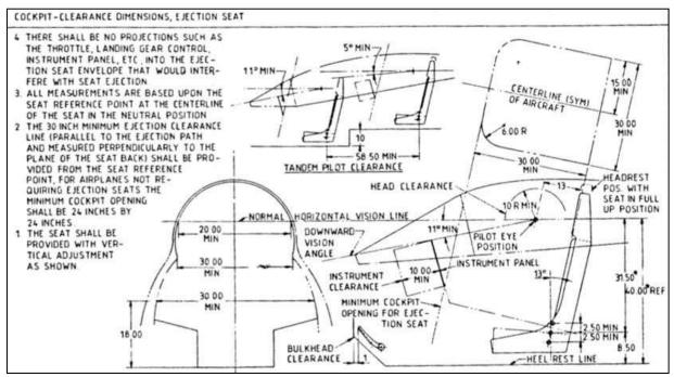
Figure 37. Recommended clearances for ejection seats [20]
