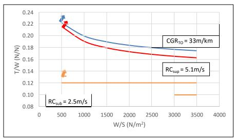
Figure 18. Climb requirement performance sizing graph
