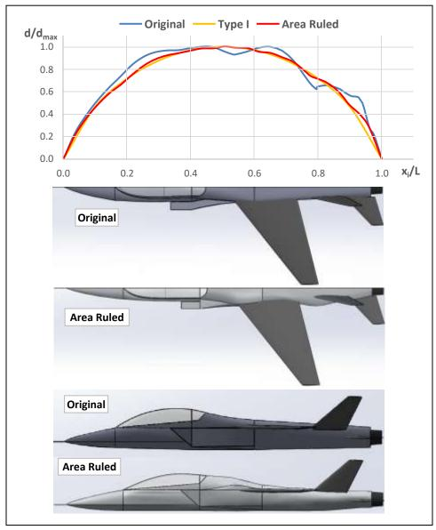
Figure 125. AMT non-dimensional diameter comparison to Sears-Haack type-I
