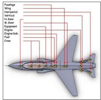
Figure 80. Top view with component center of gravity
