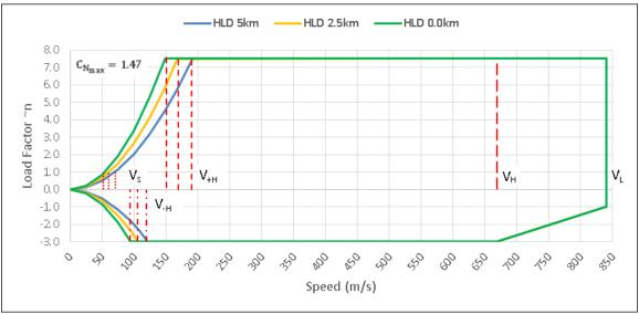
Figure 129. AMT deployed HLD configuration V-n diagram
