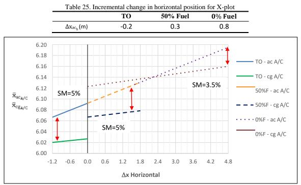
Figure 97. X-plot for change in horizontal position
