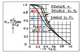
Figure 62. Relation of flap chord ratio and K factor [19]
