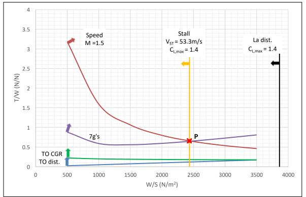
Figure 30. Hand calculation performance sizing graph
