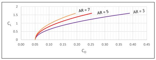
Figure 15. Takeoff and landing drag polar
