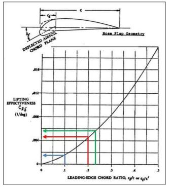
Figure 65. Effect of leading-edge flap chord ratio on  $c_{l,\delta}$  [24]
