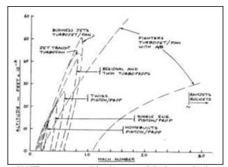
Figure 31. Mach altitude plot [19]To create an altitude versus Mach or velocity graph, equation (4.12) [18] is used. The relationship is derived from the thrust = drag equation, but neglecting wave drag. Using the
