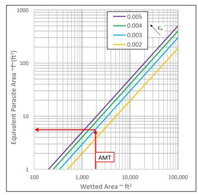
Figure 107. Effect of equivalent skin friction on wetted and parasite area reproduced from [17]
