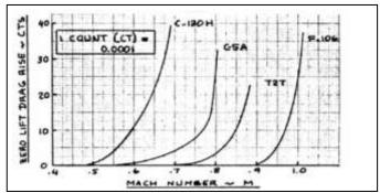
Figure 110. Zero-lift drag rise versus Mach number for various aircraft [19]
