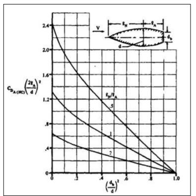
Figure 118. Interference drag of pointed forebody with truncated aftbody [29]
