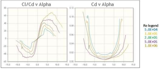
Figure 56. NACA 0008 aerodynamic polars
