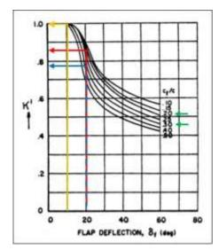
Figure 64. Effect of trailing-edge flap deflection and flap chord ratio on K' [19]
