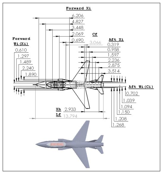
Figure 92. Layout of AMT's fuselage for Monk's method
