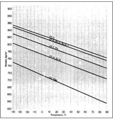
Figure 68. Aviation jet fuel densities versus temperature [25]
