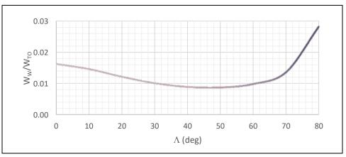
Figure 53. Wing weight percent of takeoff weight versus wing sweep angle
