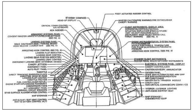
Figure 39. Fighter/attack cockpit arrangement [3]
