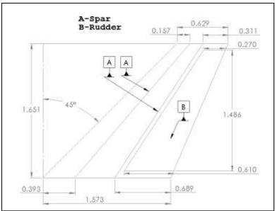
Figure 75. Vertical stabilizer geometry drawing, units in meters
