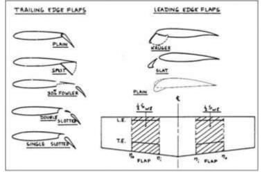
Figure 61. Wing flapped area [24]
