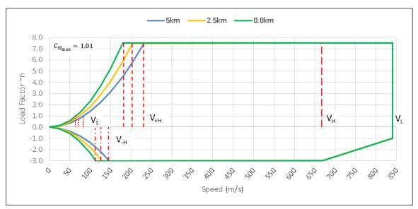
Figure 128. AMT clean configuration V-n diagram
