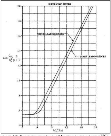
Figure 115. Supersonic drag due to lift for straight tapered wings [29]
