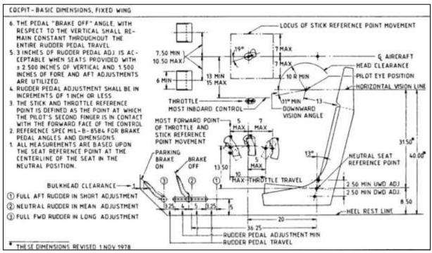
Figure 36. Recommended seat arrangement for military [20]
