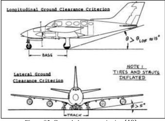
Figure 85. Ground clearance criterion [19]
