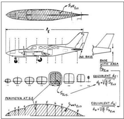
Figure 116. Fuselage parameters defined [24]
