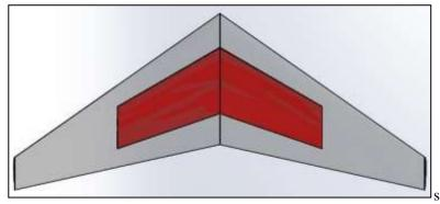
Figure 131. AMT wing fuel cell
