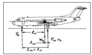
Figure 86. Landing-Gear position and symbols [19]
