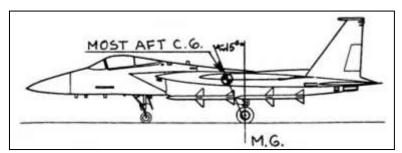
Figure 83. Tricycle gear longitudinal tip-over criterion [19]
