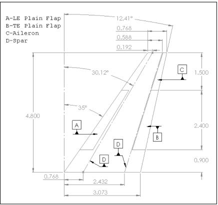
Figure 67. Proposed wing geometry, dimensions in meter
