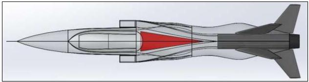
Figure 132. AMT fuselage fuel cell
