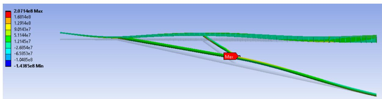
Figure 57 - Maximum stress on the connection is lowered to 2.01E8 pascals
