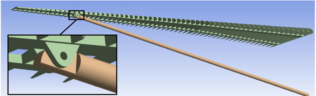
Figure 42 - Assembly of strut supported wing with pinned strut-wing connection
