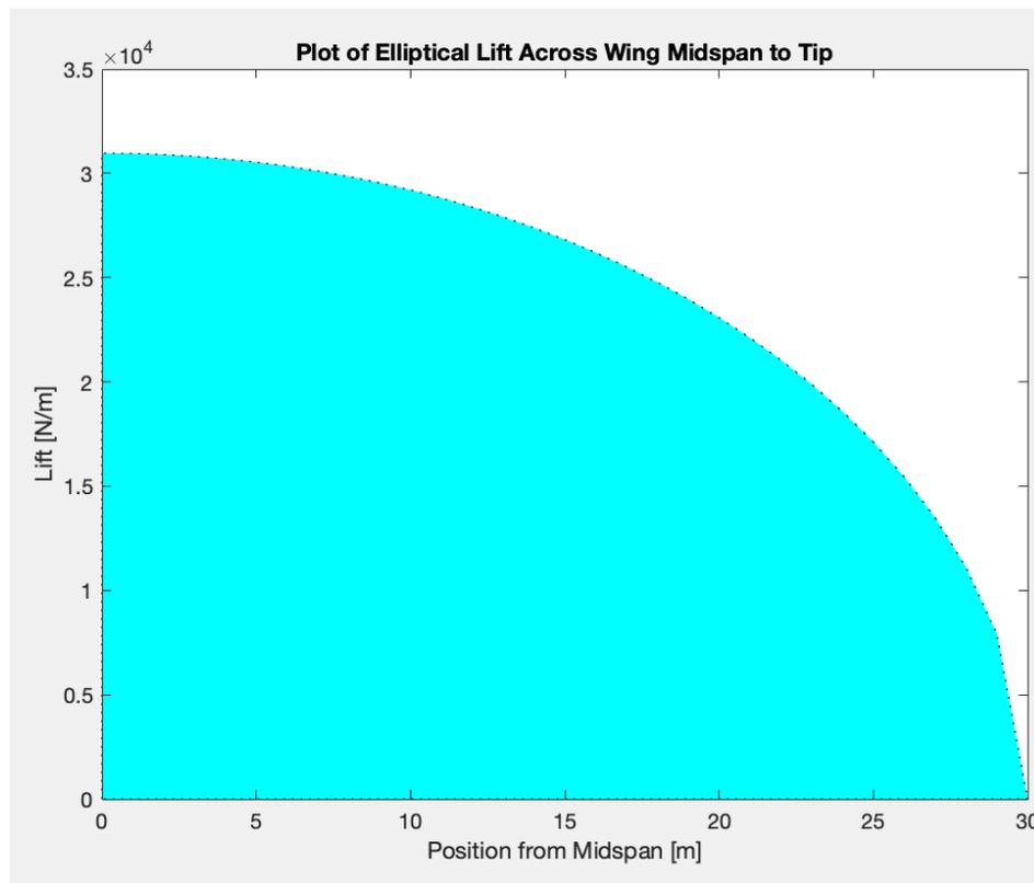
Figure 10 - Plot of elliptical loading over a half span of Boeing 777-200ER wing
