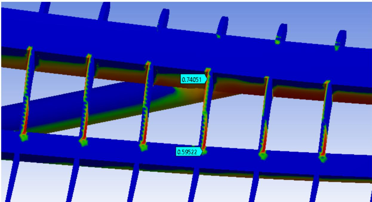
Figure 32 - Ribs shearing due to main and secondary spar moving in opposite directions
