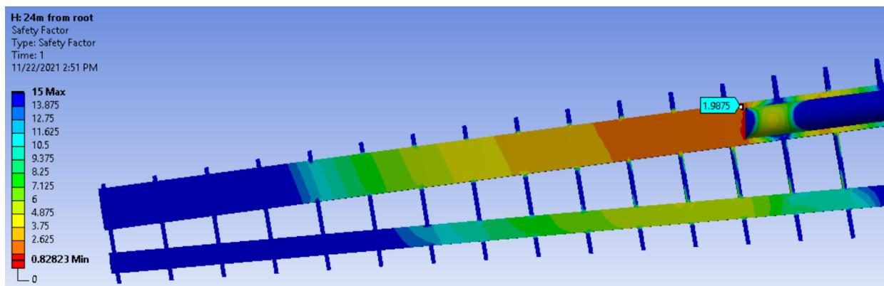
Figure 39 - Strut connected 24m from root results is stress within design specification
