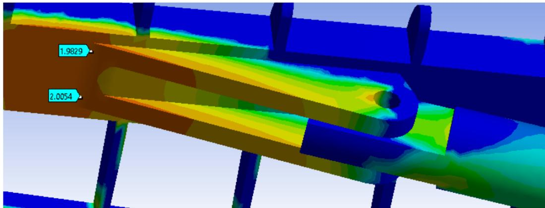
Figure 47 - Stress FOS at on modified bracket within stress parameters
