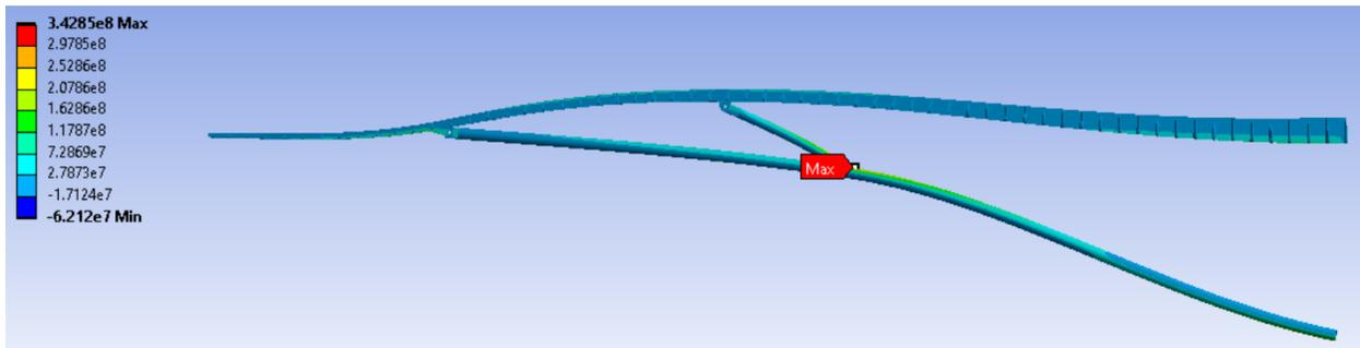
Figure 58 - Maximum principle stress with angled jury and pinned on all wing connections
