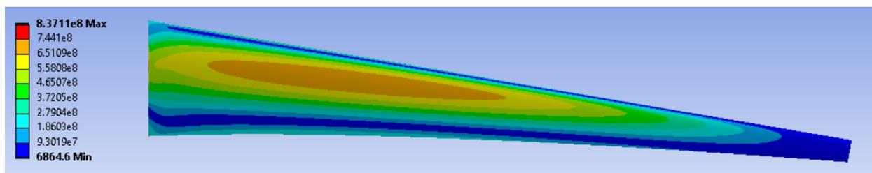
Figure 27 - Maximum principle stress shows behavior of tapered wing [pascals]
