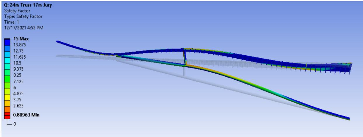
Figure 53 - 6.3x Deformed stress FOS contour of jury brace wing [pascals]
