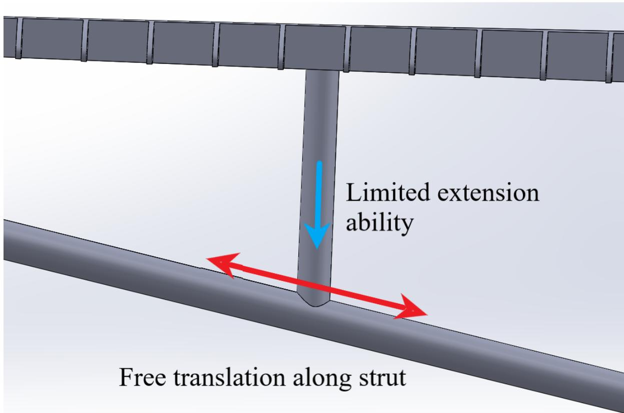
Figure 59 - Potentially feasible strut jury connection design
