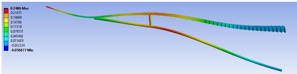
Figure 52 - 6.3x Deformed displacement contour of jury braced wing [meters]
