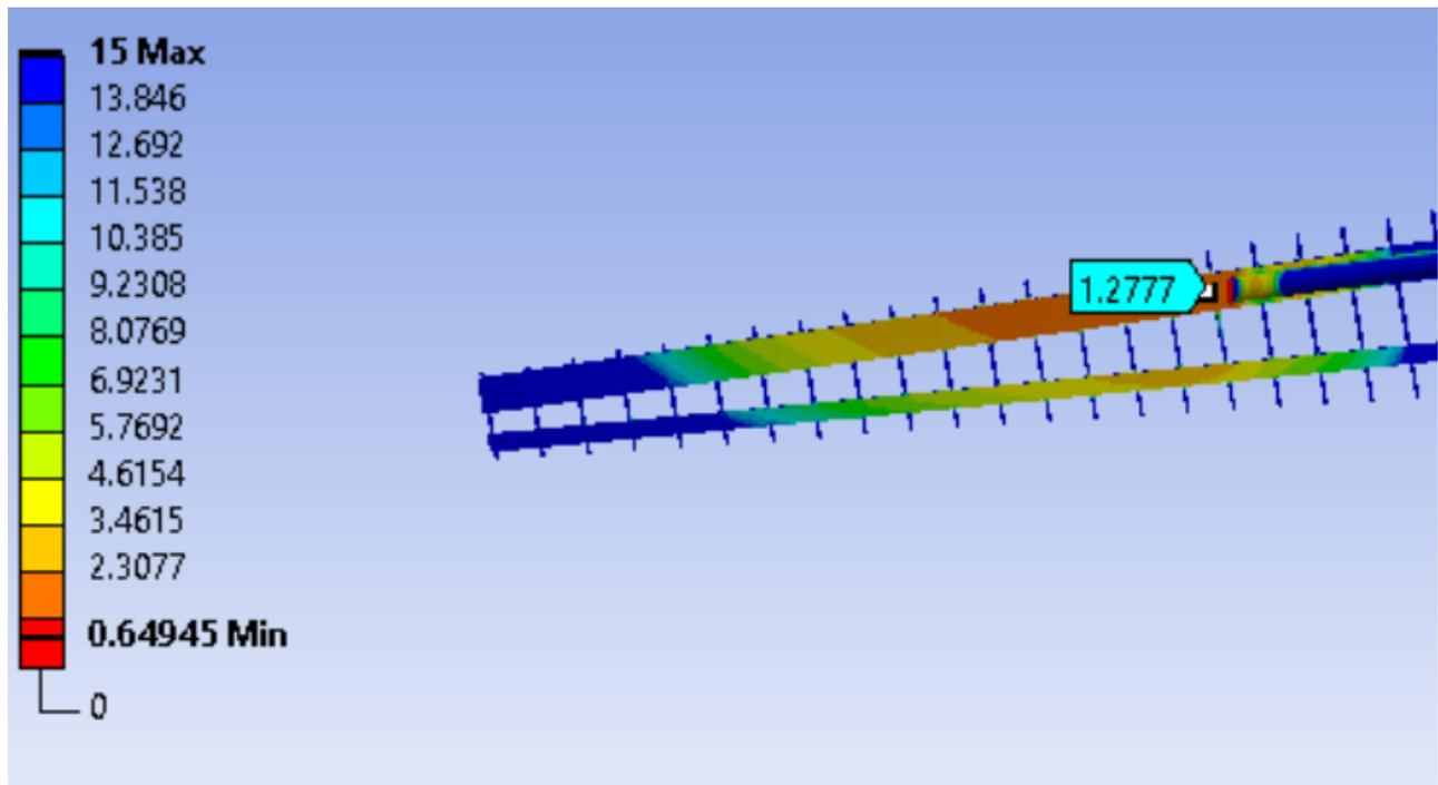
Figure 38 - Strut connected at 22m from root yields 1.28 Stress FOS
