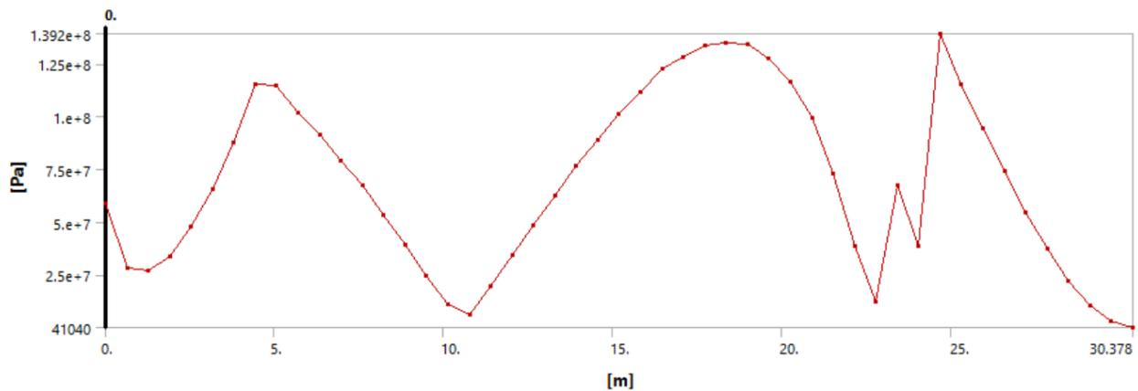
Figure 50 - Stress intensity along the main spar in a single strut configuration from wing root to tip
