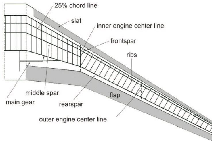
Figure 4 - F11 Megaliner internal bracing structure
