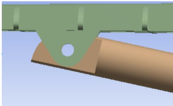
Figure 45 - Unmodified strut connection bracket
