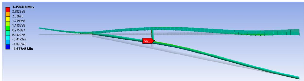
Figure 56 - Maximum stress on perpendicular connection is 3.46E8
