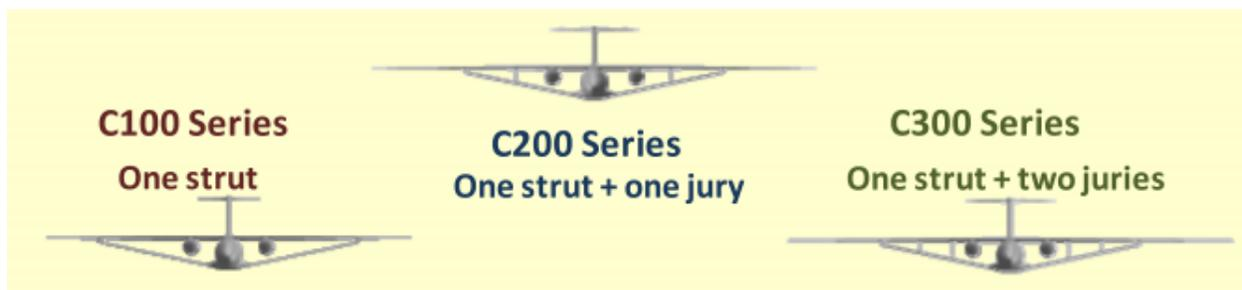
Figure 6 - Strut and truss braced wing designs tested in SUGAR project
