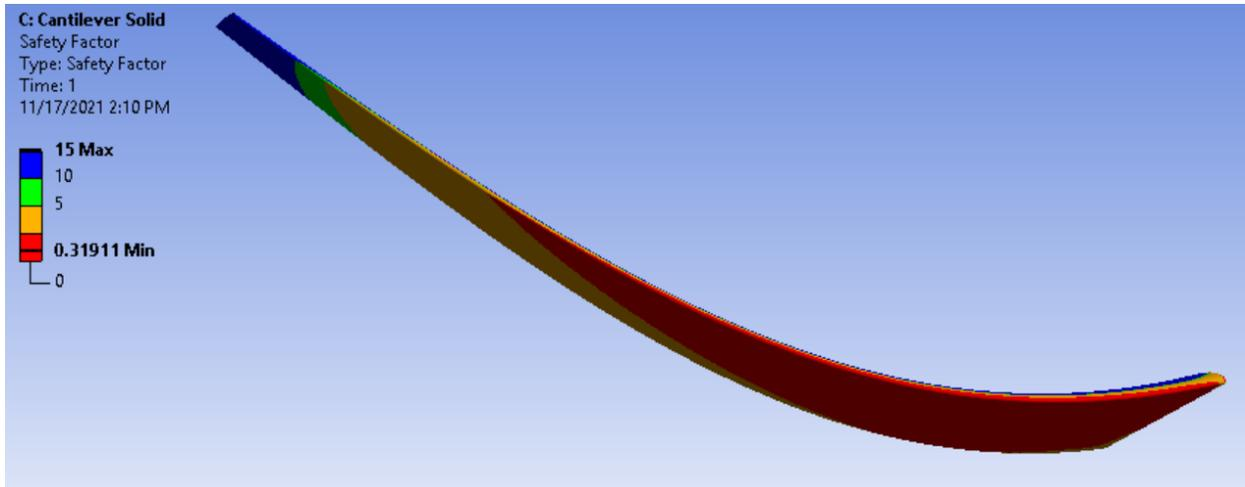
Figure 29 - 0.32 Factor of safety of stress on solid cantilever wing shows a failed result
