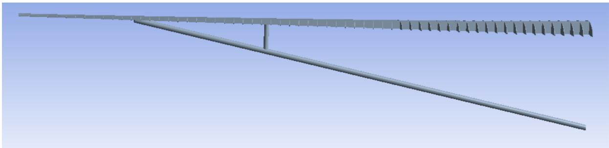
Figure 49 - Geometry of truss setup with vertical jury member at 17 meters from wing root
