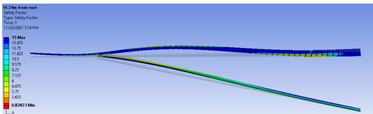
Figure 40 - 2.5x Deformed model of fixed strut configuration resulting in strut deflection as a result of wing deflection
