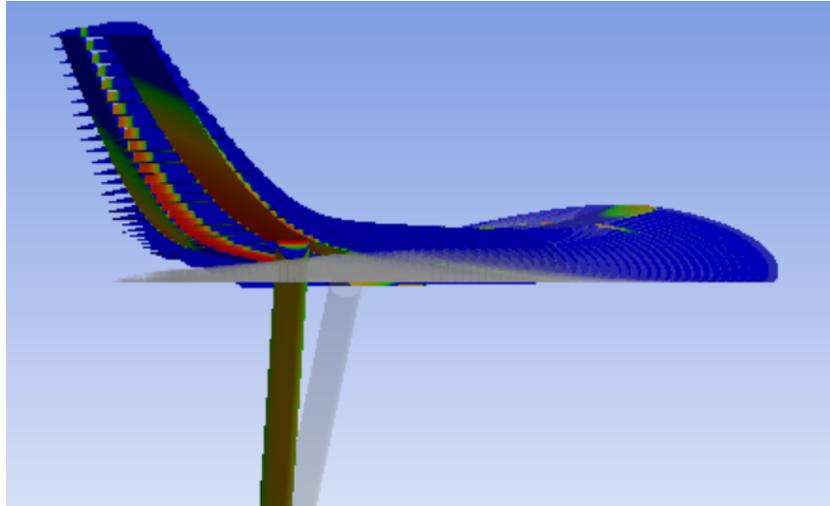
Figure 31 - Deflection in strut and translation in wing due to angle of strut with respect to wing
