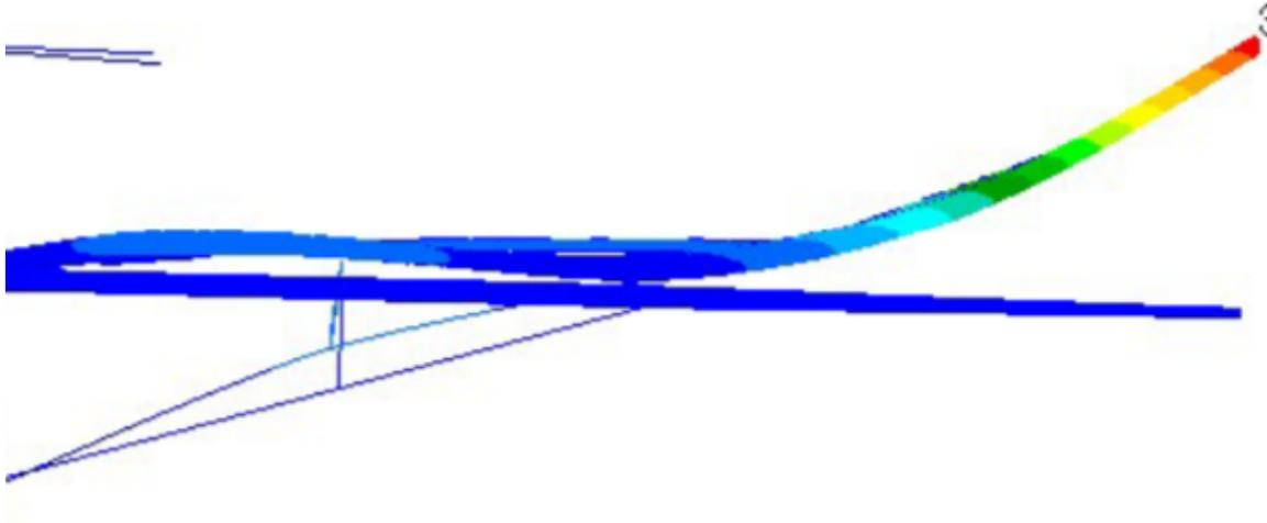
Figure 54 - Ultra Green aircraft jury braced model showing a similar high deflection at the strut to jury joint
