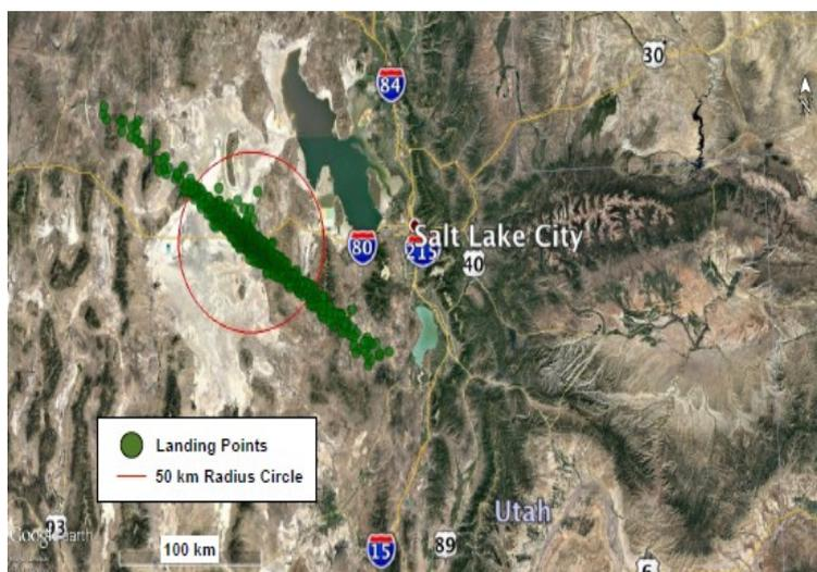
Figure 17: Landing points from a Monte Carlo simulation [3]
