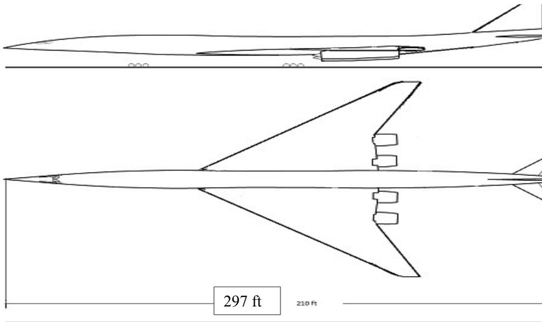
**Figure 12 Side view and Top view of the SST**
