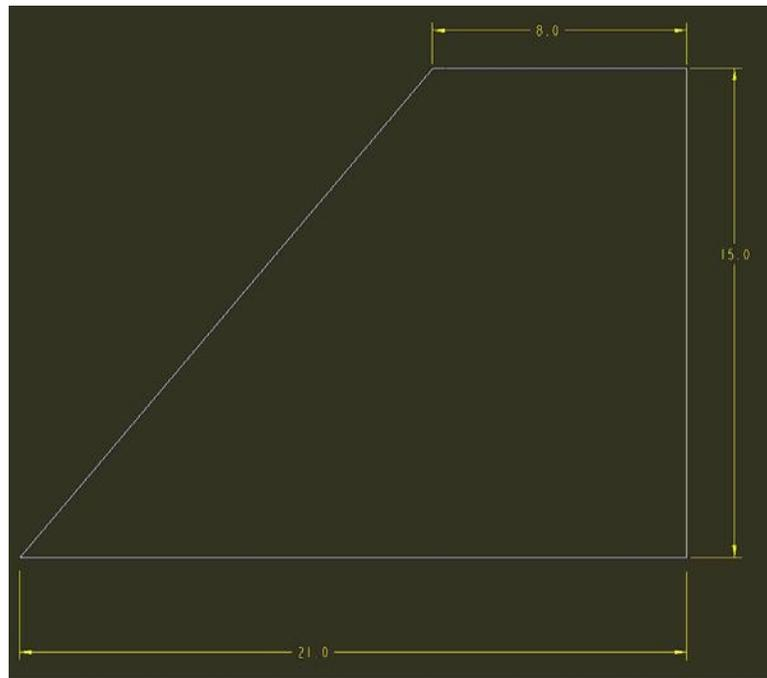
Figure 20. Geometry of a winglet
