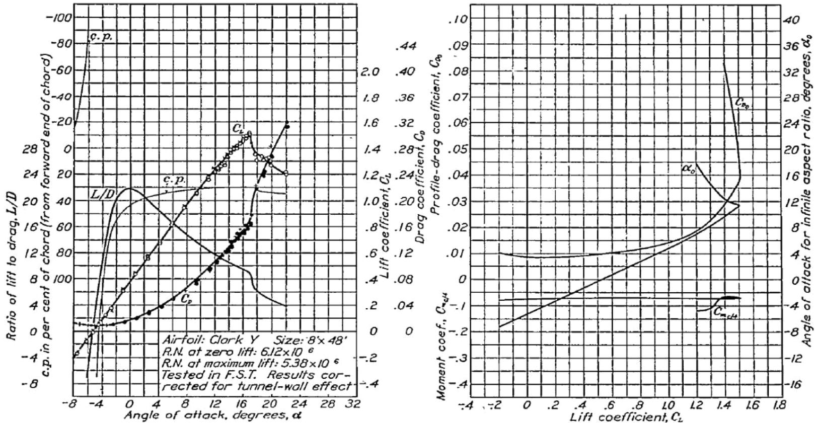
FIGURE 8.—Characteristics of the 8 by 48 Clark Y airfoil at a Reynolds Number of about 6,000,000.
