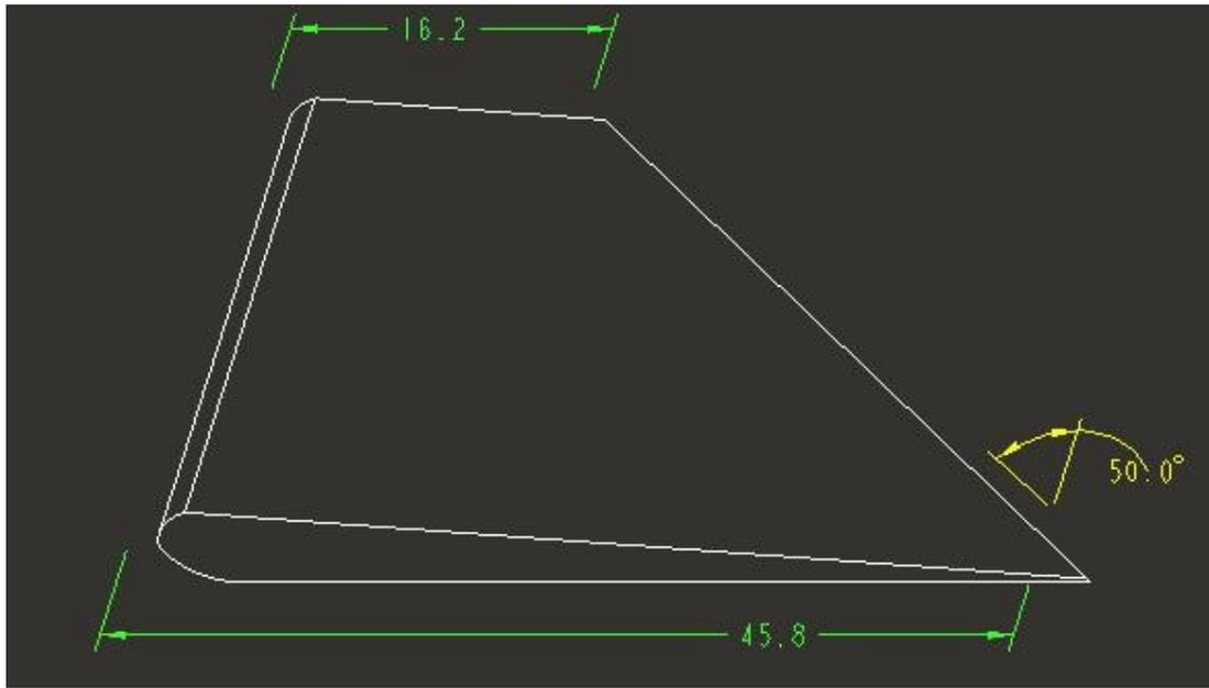
Figure 19. Geometry of a wing
