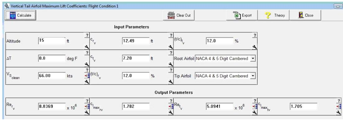
Figure 29. Lift coefficient for vertical tail of the hoverwing
