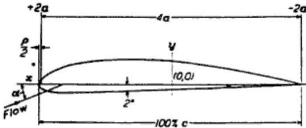
Figure 16. Geometry of Clark Y airfoil [6]
