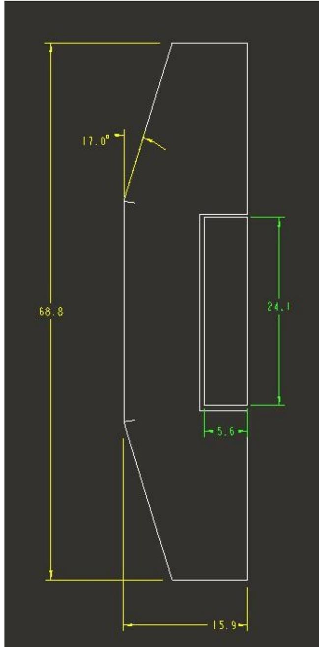
Figure 33. Geometry of a horizontal stabilizer
