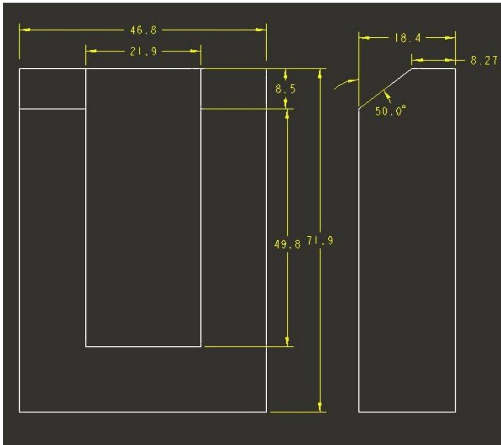
Figure 13. Design of the fuselage of hoverwing
