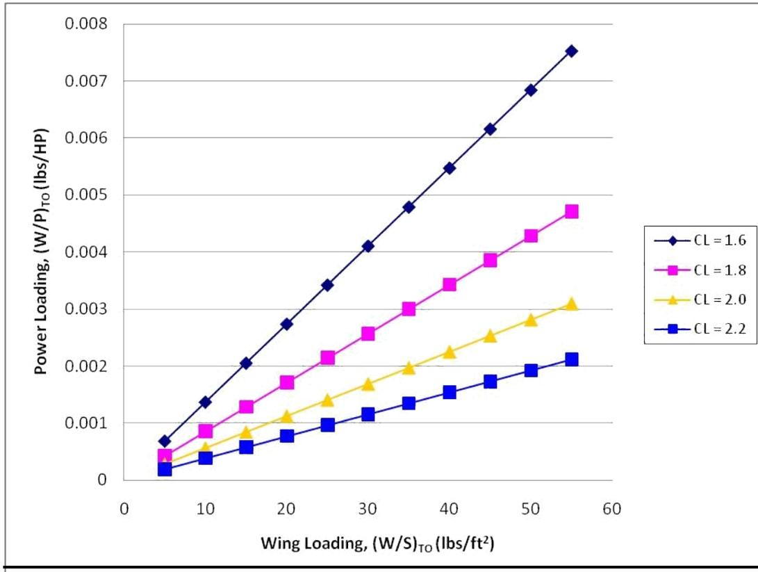
Figure 8. Power loading vs Wing loading as a function of varied lift coefficient
