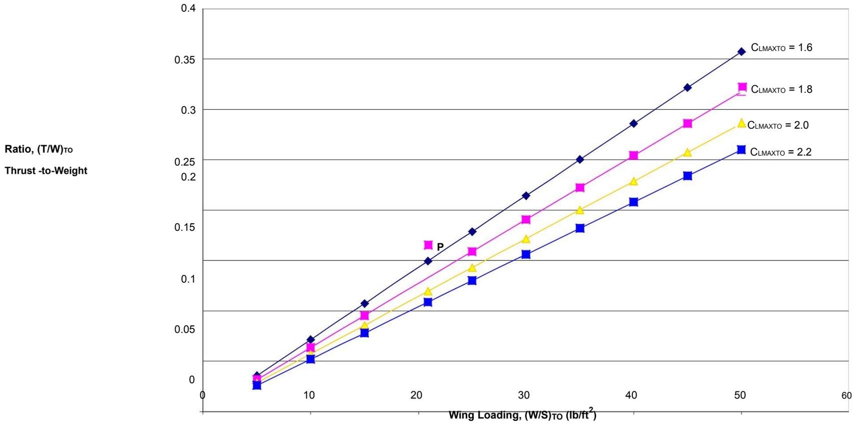
Figure 7. Thrust-to-weight ratio vs Wing loading as a function of varied lift coefficient
