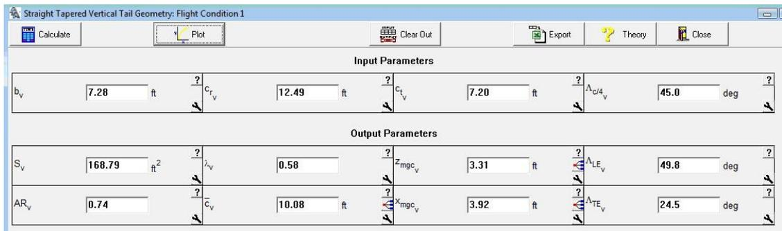
Figure 26. Vertical tail geometry using AAA
