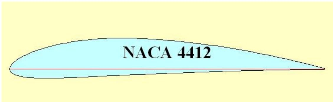
Figure 21. Shape of NACA 4412 airfoil
