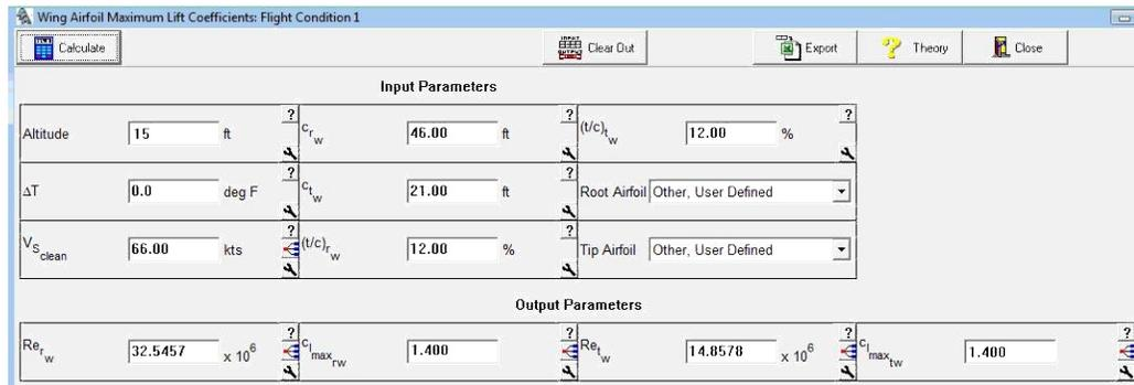
Figure 18. Calculation of lift coefficient using AAA program
