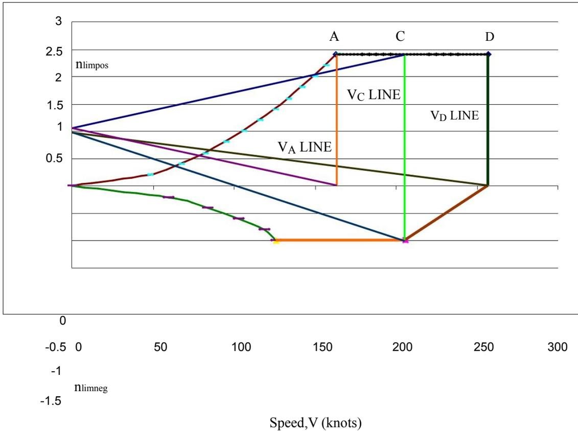
Figure 49. V-n Diagram
