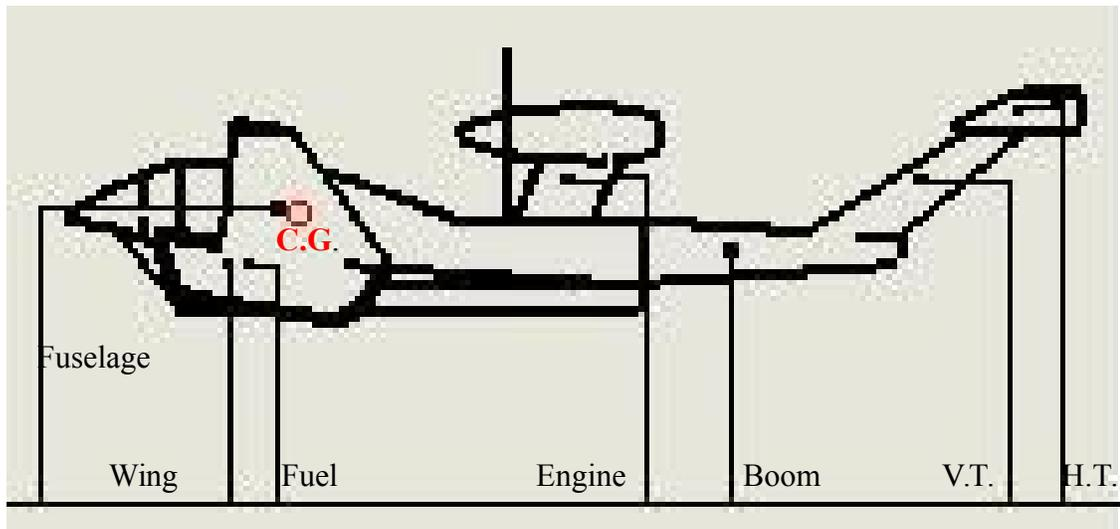
Figure 35. Location of centre of gravity in Y-direction
