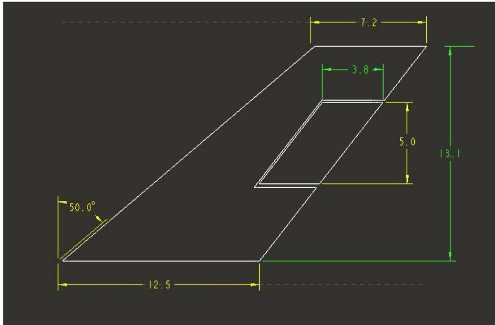
Figure 30. Geometry of a vertical stabilizer
