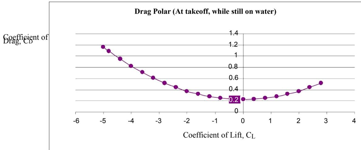
Figure 46 Drag Polar (At takeoff, while still on water)
