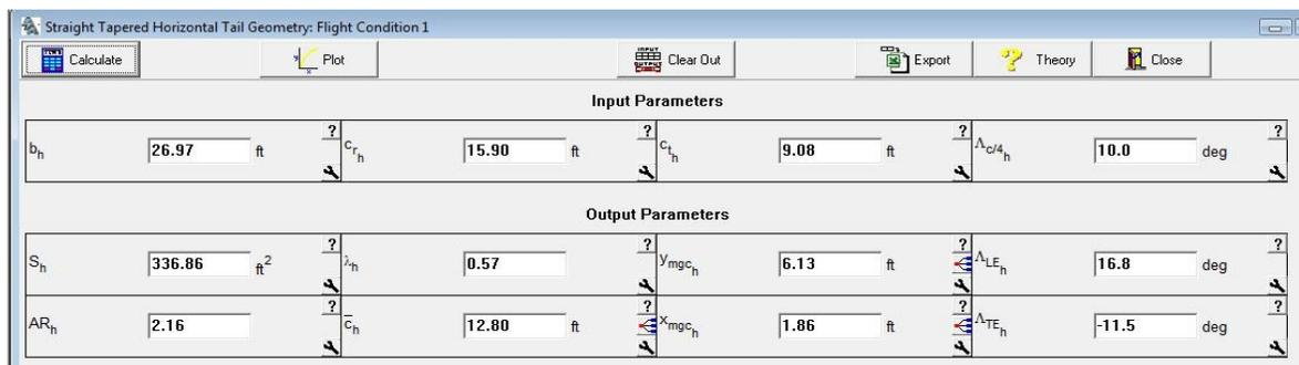
Figure 24. Horizontal tail geometry tapered using AAA
