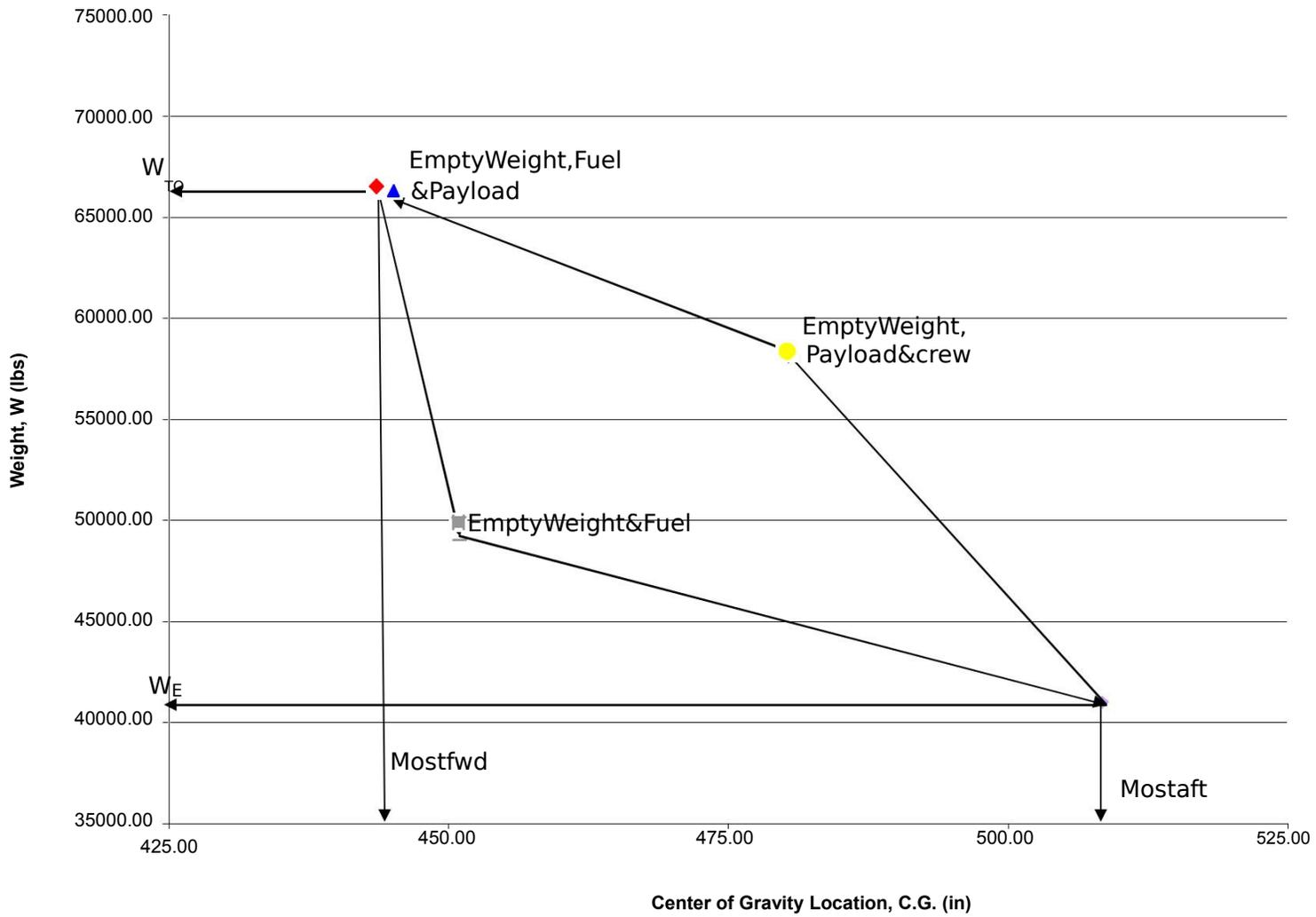
Figure 36. Center of Gravity excursion diagram
