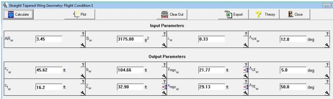
Figure 15. Straight tapered wing geometry
