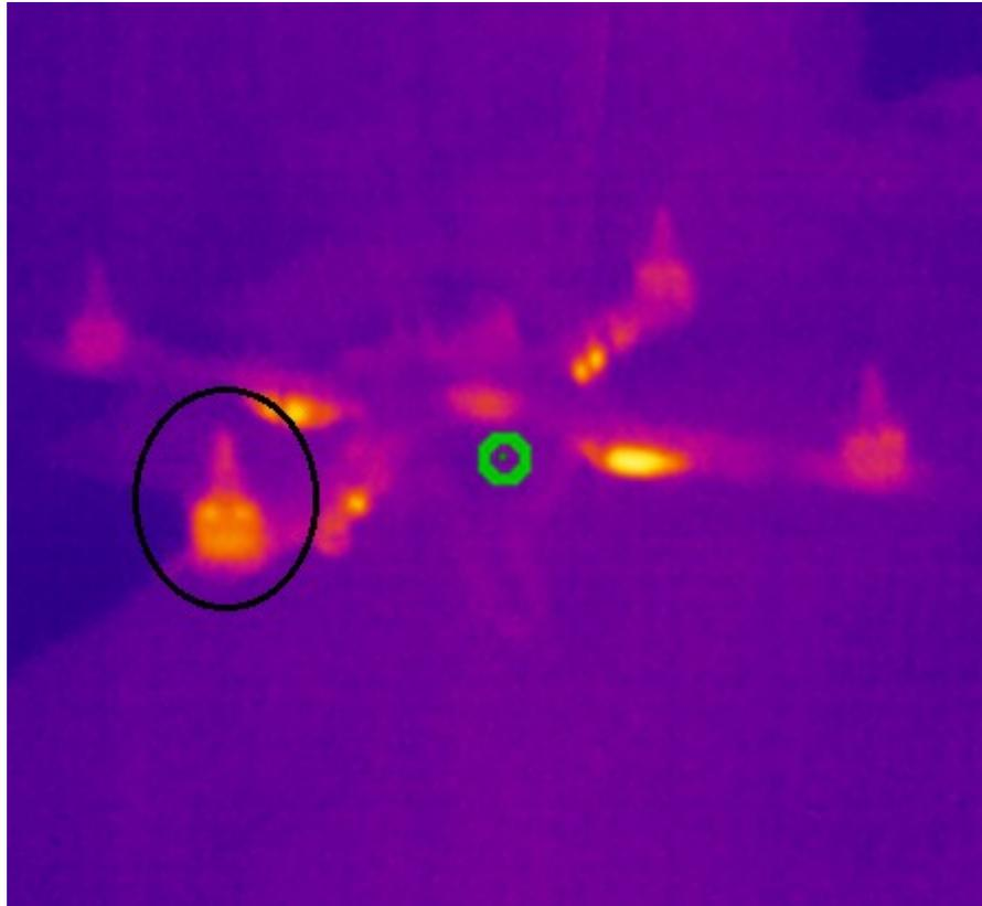
**Figure 10. Infrared view of stress test (Erroneous Motor Circled).**
