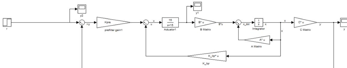
**Figure 5. Nominal linear quadratic regulator controller with a step input.**
