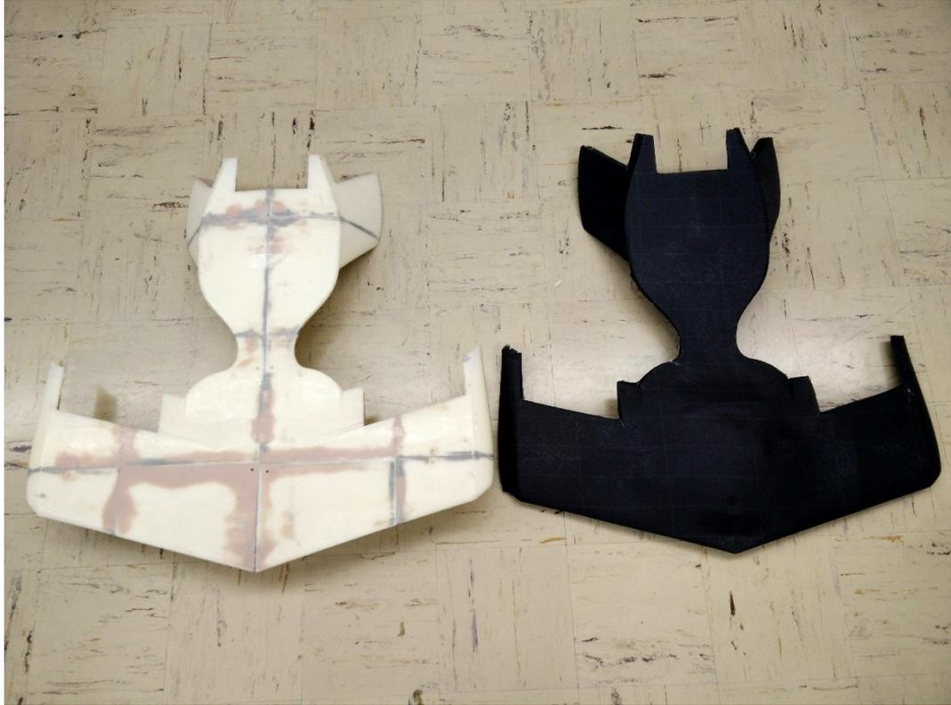
**Figure 9. Mold and airframe top section**
