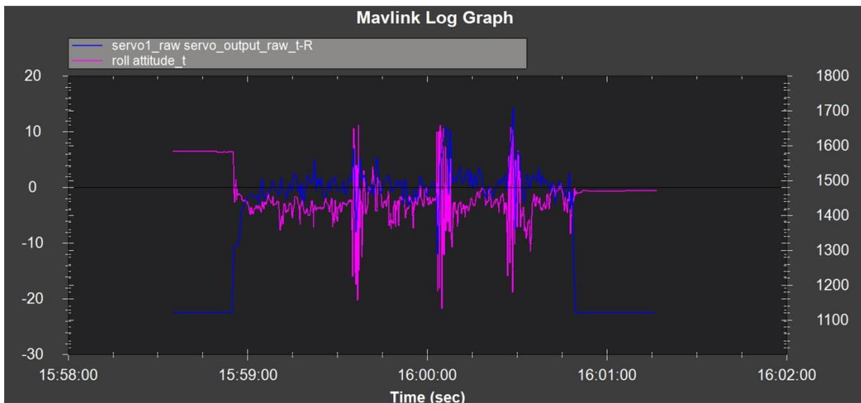
Figure 11. Input vs. Output Data for Roll Chirp
