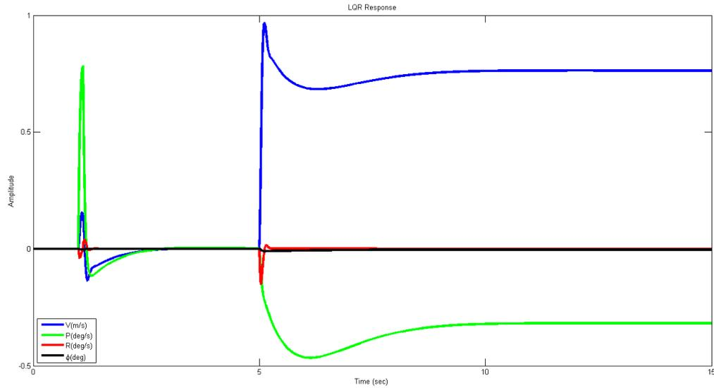
**Figure 6. Lateral directional responses to impulse and step inputs.**
