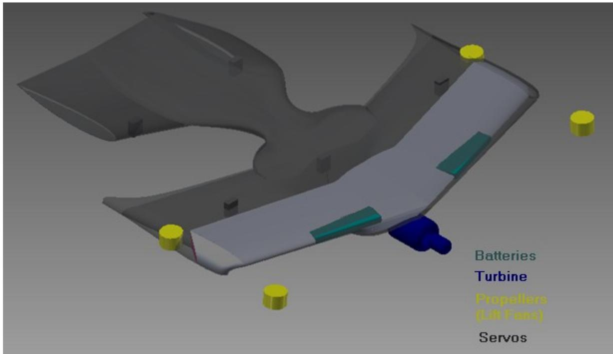
**Figure 1. General configuration of aircraft.**
