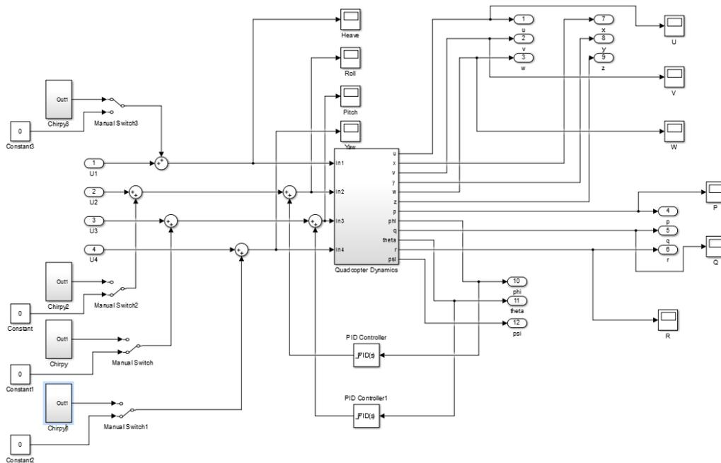
**Figure 7. MATLAB Simulink setup for quad-copter.**
