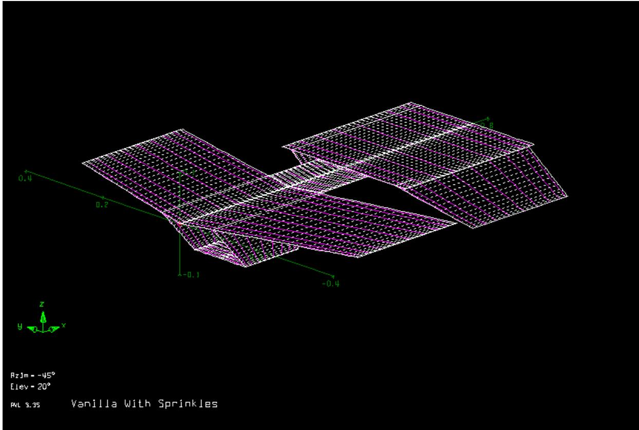
**Figure 2. Vortex lattice approximation of UAV model.**
