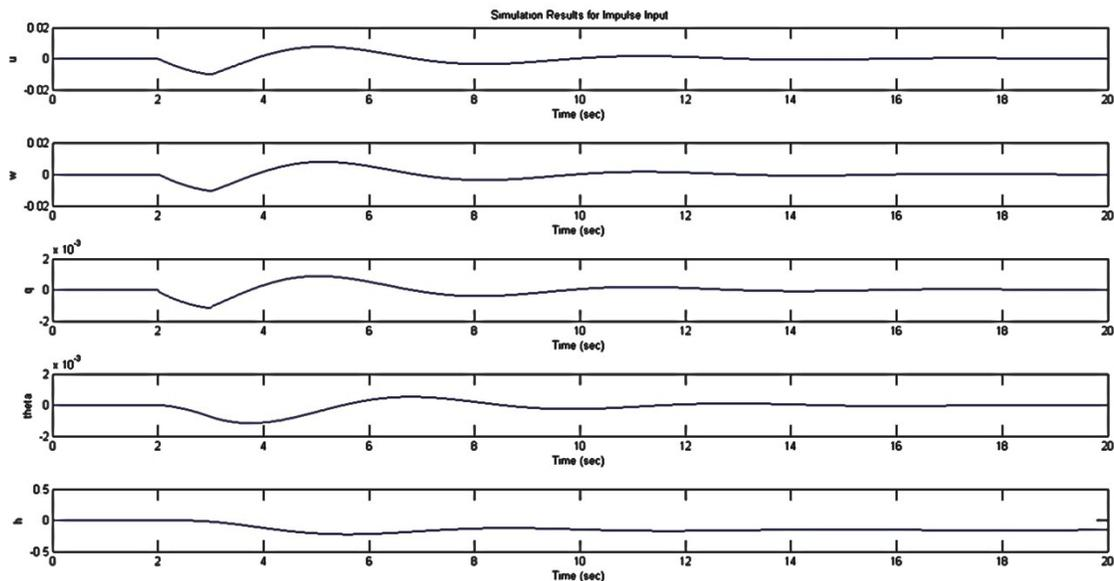
**Figure 4. Open-loop response of longitudinal dynamics.**
