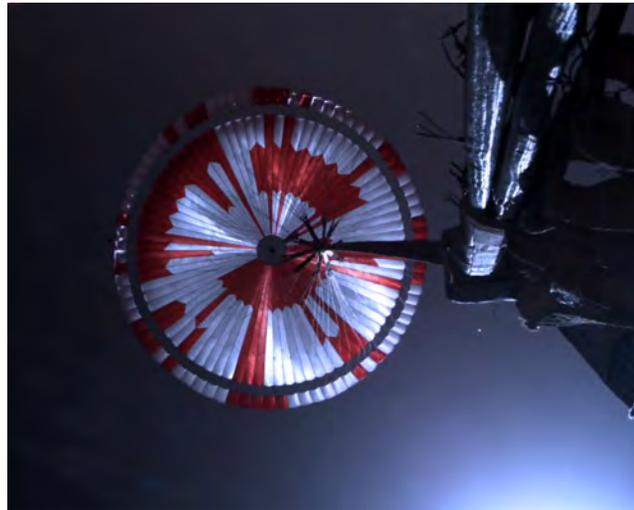
Figure 6.1: Disk-band-gap parachute of Mars 2020, fully inflated. The gap is clearly visible. While sacrificing on maximum drag, it is the only proven parachute design that deploys at supersonic speeds. Credit: NASA JPL/Caltech.
