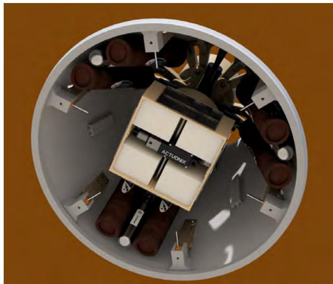
Figure 4.2: Internal render of Nines as an independent, 1U CubeSat mission of opportunity. Prominently shown is the 1U CubeSat, six solid rocket retropropulsion motors, and three gas thruster cartridges.
