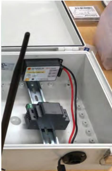
Figure 5.4: DIN rail mounting mechanism for power supplies and industrial Raspberry Pi. Credit: Stanley Krzeńskiak
