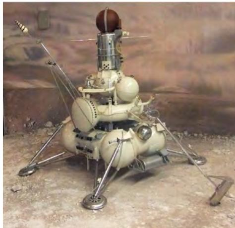
Figure 1.9: A model of the Roscosmos Luna 16 spacecraft. The scoop and spiral helical antenna are prominent. Credit: Asif Siddiqi.
