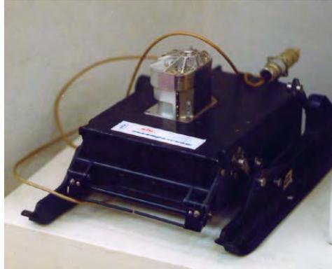
Figure 1.13: A model of the PrOP-M rover, a part of the Soviet Mars 2 mission. Credit: T. Varfolomeyev.
