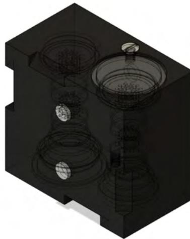
Figure 1.25: General purpose heat source CAD drawing, fully assembled and defined. Four plutonium fuel pellets are visible as silhouettes, with pairs encapsulated in their own silos contained in carbon-carbon sleeves. Credit: Stanley Krześniak.
