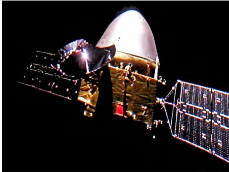
Figure 1.38: The Tianwen 1 cruise stage and orbiter. The upper part shows an oblong, white object - this is the Zhurong EDLS. It is apparent that the EDLS backshell is taller than U.S. designs. The reflective object off the left side is the high-gain dish antenna, and the gold rectangle is the cruise stage and orbiter. Credit: China National Space Administration.
