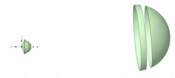
Figure 6.26: Off-axis parachute. No bridles are modeled to allow for computational simplicity.
