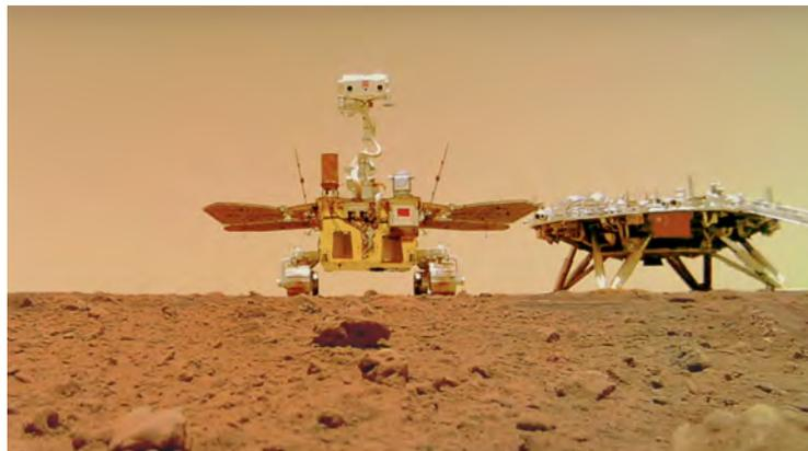
Figure 1.36: The Zhurong rover and lander system, imaged by a deployable remote imager. The imaging unit transferred data through a WiFi network. Credit: China News Service.
