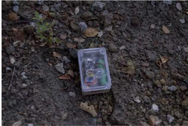
Figure 5.9: R2 node in a clear polycarbonate junction box in the test environment.
