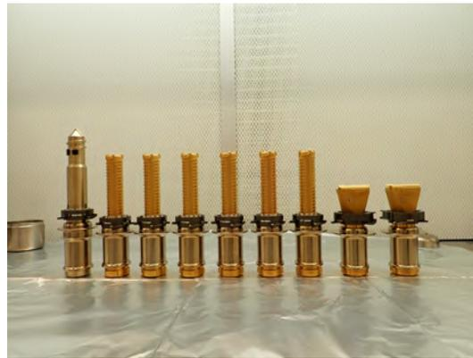
Figure 1.30: Perseverance's sample caching system drill bits. On the far left with a conical tip is a regolith drill, designed to drill into softer soil. The six drills in the middle are rock-coring drills, which have a cavity inside to allow rock to be deposited into a sample tube. On the right are two abrasion drills, which clean off a surface before measurements or a sample is taken. The gold color on all drills and abrasion tools are titanium nitride. Credit: NASA/JPL.
