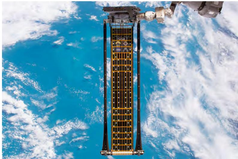
Figure 3.7: U.S. Air Force's Roll-out Solar Array (ROSA) mounted on Canadarm at the ISS for system validation and testing. Credit: NASA/Air Force Research Laboratory.
