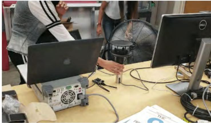
Figure 5.7: Completing a test of the Windsonic ultrasonic wind sensor with a standard room fan. Credit: Nataliya Grigoryan.
