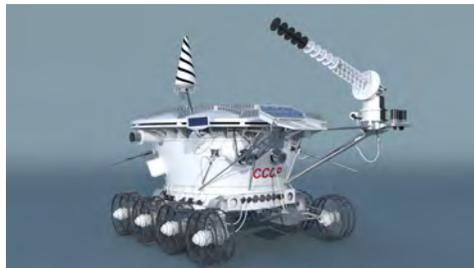
Figure 1.10: A high-resolution rendering of the Lunokhod 1 rover, part of the Luna 17 lander. To enable high-rate data return, a steerable Yagi was incorporated onto the rover. A conical helix antenna provided a low-gain link. Credit: NASA NSSDC.
