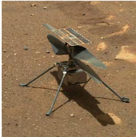
Figure 1.34: Ingenuity Helicopter sitting on the surface of Mars after being deployed by Perseverance. Credit: Jet Propulsion Laboratory.
