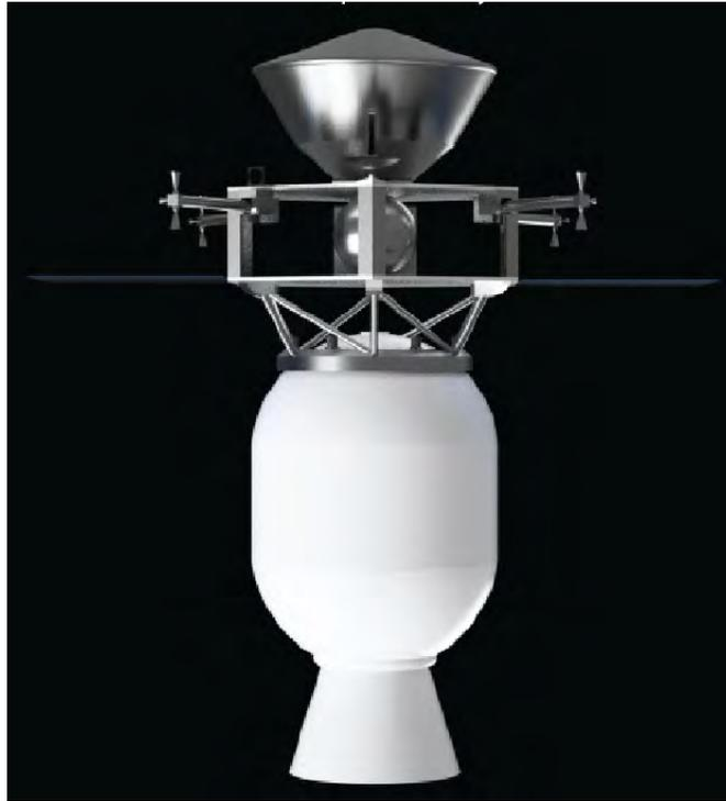
Figure 4.13: Initial revision of a free-flyer version of Wavefront. The white engine is a Star 37D solid rocket kick motor.
