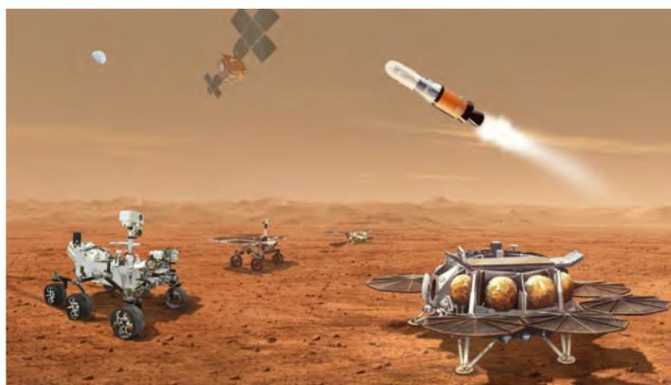
Figure 1.3: Concept of operations for NASA’s Mars Sample Return mission, including all assets. From bottom left to top left counterclockwise: NASA Mars 2020/Perseverance, ESA Sample Fetch Rover, ESA Sample Fetch Lander, NASA Sample Retrieval Lander, NASA Mars Ascent Vehicle, and ESA Earth Return Orbiter. Credit: NASA/-Caltech Jet Propulsion Laboratory
