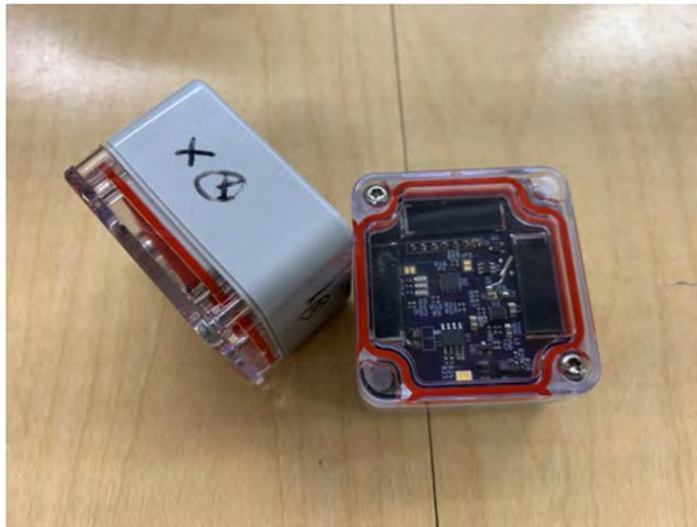
Figure 5.10: Two R3 Nines nodes. The containers are off-the-shelf and contain two custom PCBAs stacked internally.
