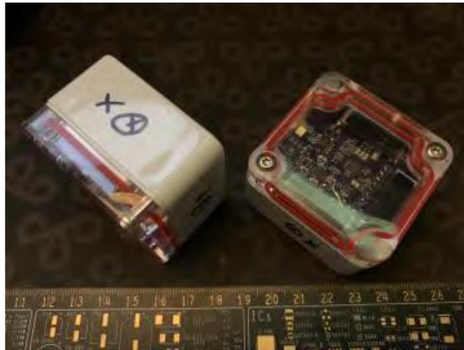
Figure 4.7: Nines probes, version 2, with ruler for scale. The polycarbonate boxes held a complete Internet of Things node inside, fabricated on two stacked PCBs.
