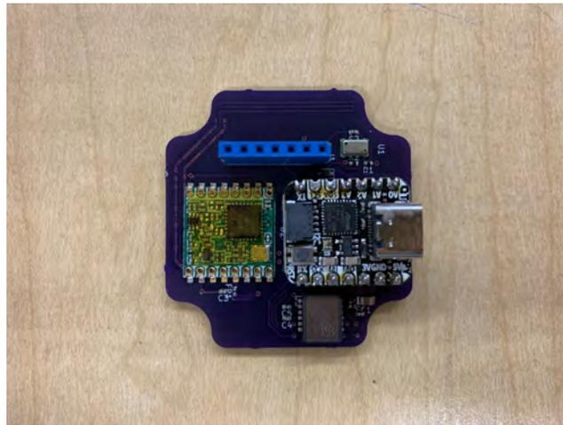
Figure 5.13: Lower stack. This contains a LoRa modem under Kapton tape, an off-the-shelf microcontroller, precision inclinometer, and pressure/temperature/humidity sensors. The blue header is a board-to-board connector, which contains 3.3V, I<sup>2</sup>C data, and three GPIO control lines.
