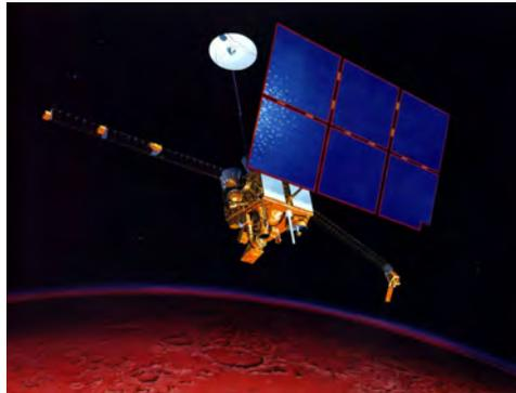
Figure 1.17: A rendering of the ill-fated Mars Observer. Featured prominently are the large solar panels, long instrument booms, and steerable dish antenna. Credit: NASA.
