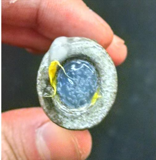
**Figure 16: Gel with air pockets clogging outlet**
