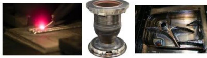
Figure 1.6 - Electron beam deposition [4]
