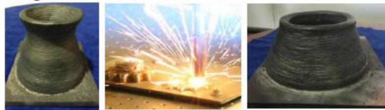
Figure 1.5 - Arc-based deposition [4]
