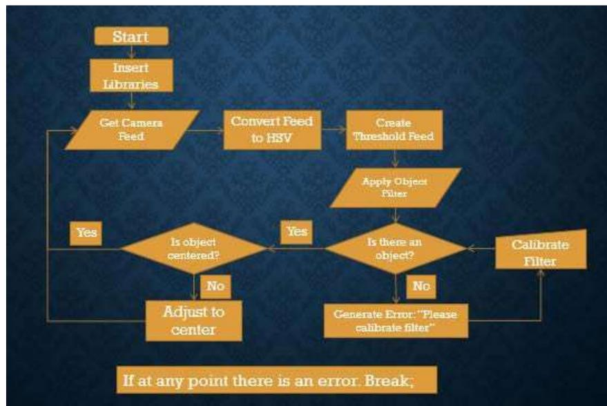
Figure 4.1: Color Blob HSV Programming Flow
