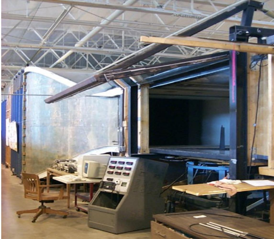
Figure 31- Example test section door for a 4x6 wind tunnel. (Purdue University)
