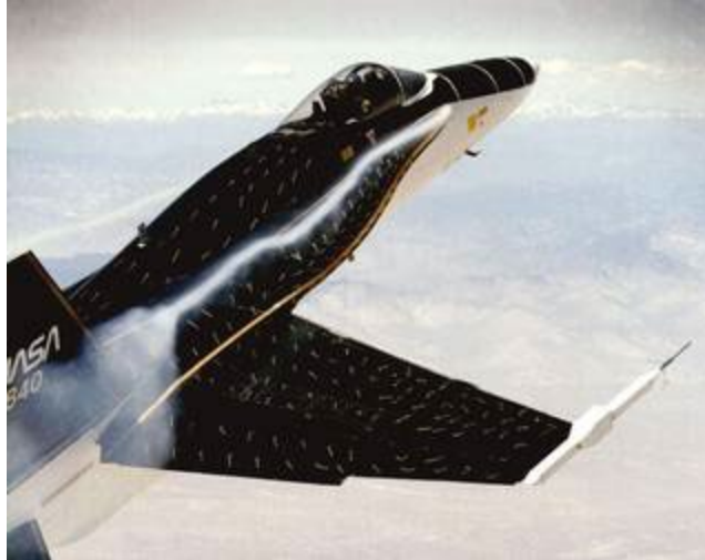
Figure 1.1 - F-18 HARV flow visualization during phase one testing. [2]
