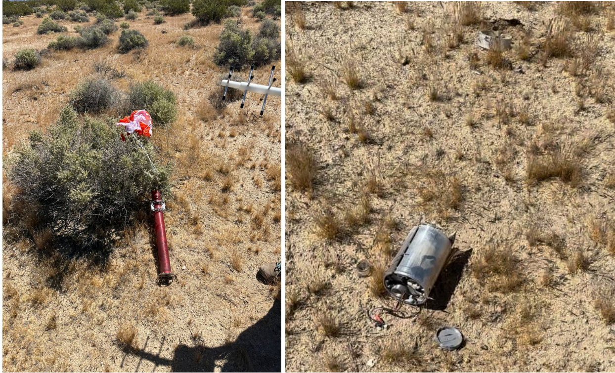
Figure 1.6 - On the left is the aft section with a working GPS after the crash landing. On the right, the forward section is crushed into a few pieces near the round crater, a few meters away from the aft section.
