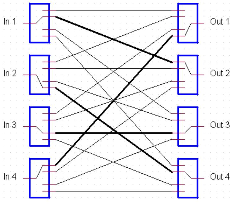
**Figure 1.2-1: 4x4 Switch Matrix Function View**
