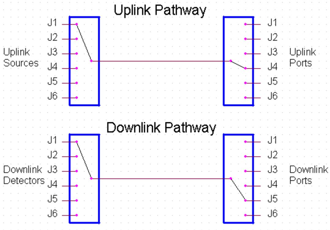
**Figure 11.3-2: Switch Position Block Diagram**
