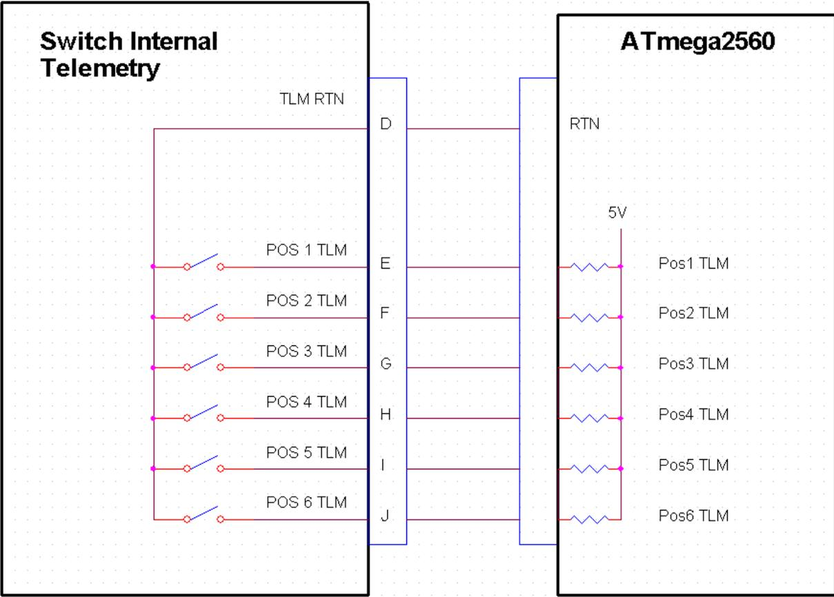
**Figure 6.1-1: Switch Telemetry Diagram**
