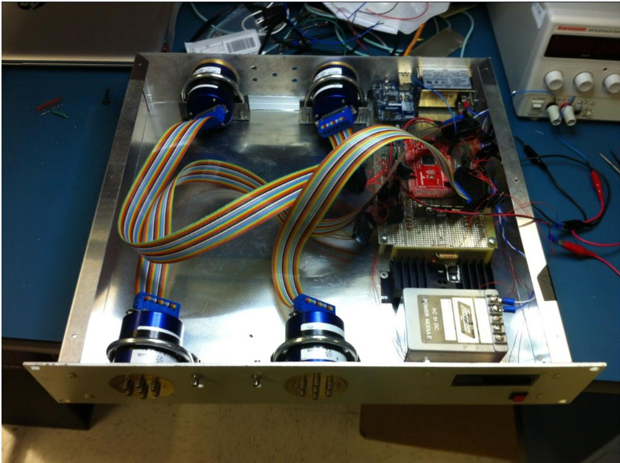
**Figure 12.3-1: Switch Matrix Fully Integrated**
