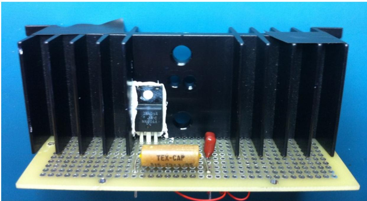
**Figure 8-2: Built 9 Volt Power Regulation Circuit with Heat sink**
