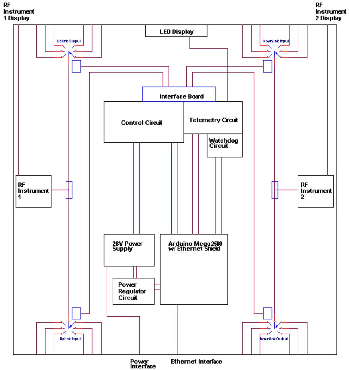
**Figure 3-3: Switch Matrix System Overview**
