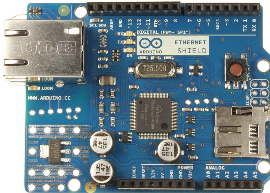
**Figure 4.3-1: Arduino Ethernet Shield**
