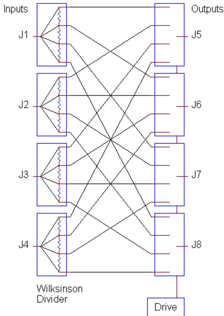
**Figure 1.2-5: Full Access (Non-Blocking) Design**
