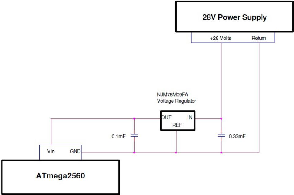
**Figure 8-1: 9 Volt Power Regulation Circuit**
