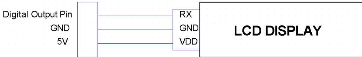
**Figure 6.2-2: LCD Wiring Diagram**
