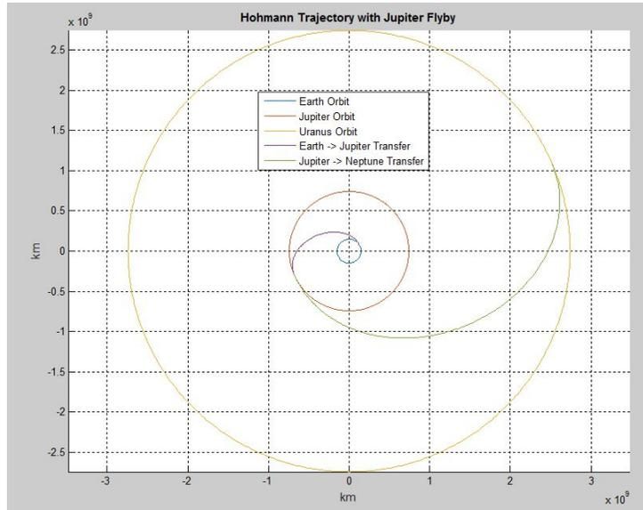
**Figure 3. Orbital Assist Around Jupiter to Uranus for the Case of April 2<sup>nd</sup> 2180**
