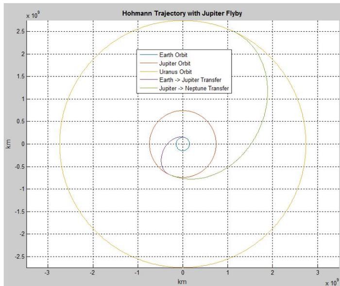
**Figure 2. Orbital Assist Around Jupiter to Uranus for the Case of December 15<sup>th</sup> 2060**
