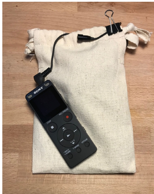
Adapting a voice recorder to be clipped on and carried inside or outside a pocket on young visitors.
