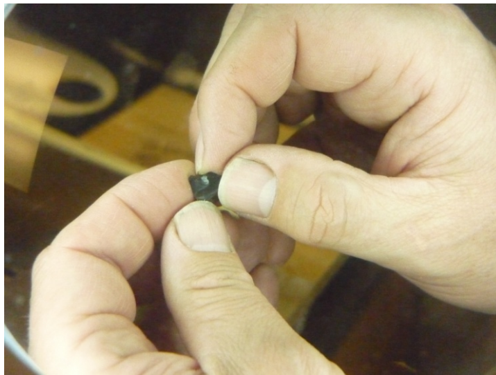
Figure 62: Choosing a Location for Obsidian Thin Section Removal
