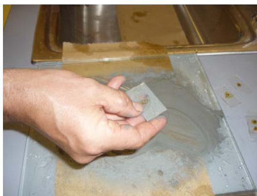
Figure 68: Grinding Obsidian Thin Section to Half its Original Thickness
