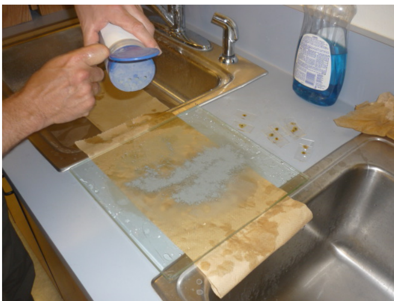
Figure 67: Preparing To Grind Thin Section Slides Using 600-Grit Powder, Glass Plate and Water
