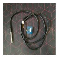
Fig. 3: Temperature Sensor
