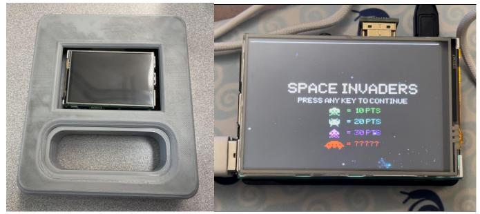
*Figure 1 (left): The handle with the LED screen in it Figure 2 (right): Raspberry Pi running the games that display on the LED screen*
