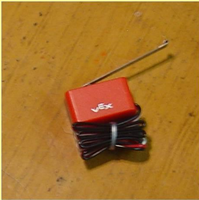
Limit Switch Sensor
