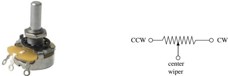
Figure A.5 Potentiometer. A potentiometer (POT) is a variable resistor. The resistance between the center wiper terminal and either of the end terminals depends on the rotation angle of the shaft.
