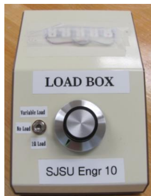
Figure 4 Load Box. LEDs are used as the load for the wind turbine. A POT is used for adjusting the amount of loading to the wind turbine generator.
