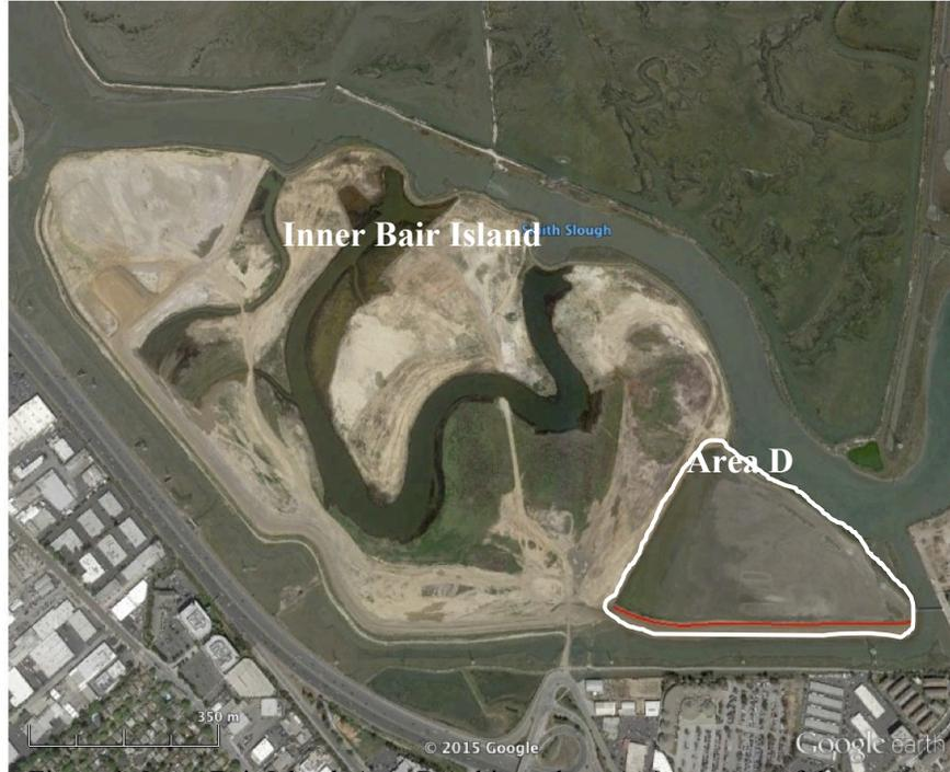
Figure 1. Inner Bair Island, Area D (white polygon). A segment of the northern slope of levee (red line) would be selected for SJSU monitoring.
