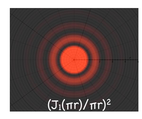
The region inside of this is called the "Airy disk". The size of the airy disk is the minimum size a circular lens can focus light to. If this is larger than any other aberrations the lens or optical system is said to be "diffraction limited"
