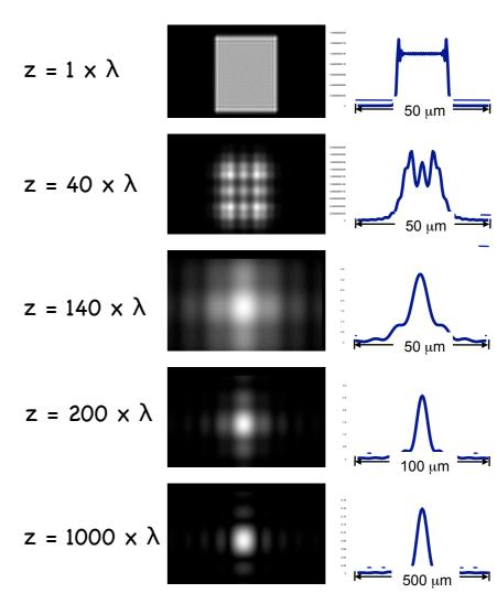
The intensity profile from a uniformly illumiaetd square aperture of size x by x at various distances from the aperture.
