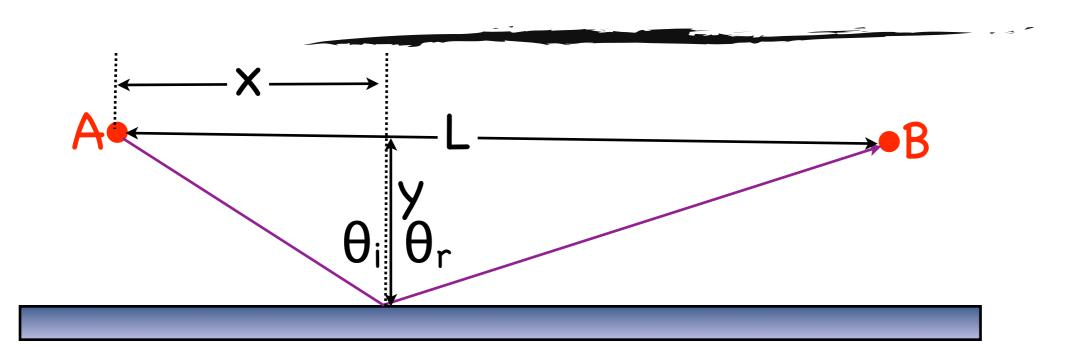
$$\begin{aligned} OPL &= \sqrt{x^2 + y^2} + \sqrt{(L - x)^2 + y^2} \\ \frac{d(OPL)}{dx} &= \frac{x}{\sqrt{x^2 + y^2}} - \frac{L - x}{\sqrt{(L - x)^2 + y^2}} \\ \frac{d(OPL)}{dx} &= \sin \theta_i - \sin \theta_r \to 0 \end{aligned}$$
