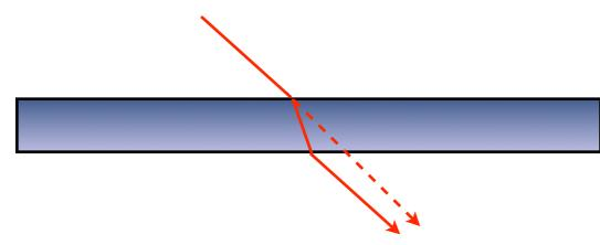
displacement of a ray through a plane of glass
