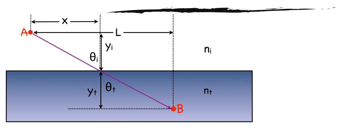
$$\begin{split} OPL &= n_i \sqrt{x^2 + y^2} + n_t \sqrt{(L - x)^2 + \mathbf{y}^2} \\ \frac{d(OPL)}{dx} &= \frac{xn_i}{\sqrt{y_i^2 + x^2}} - \frac{(L - x)n_t}{\sqrt{y_t^2 + (L - x)^2}} \\ \frac{d(OPL)}{dx} &= n_i \sin \theta_i - n_t \sin \theta_t \to 0 \end{split}$$
