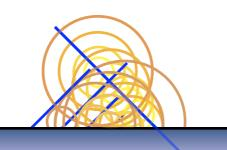
Angle of reflected wavefront is equal to that of incident wavefront
