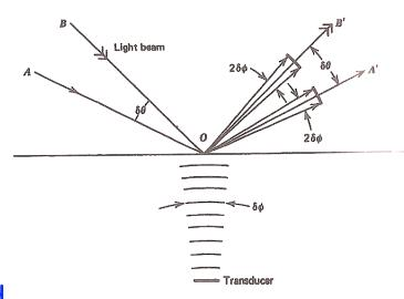
in the acoustic beam must equal or exceed that of the optical beam  $\delta\phi \geq \delta\theta = \lambda/\pi n\omega_0$  giving a bandwdith
